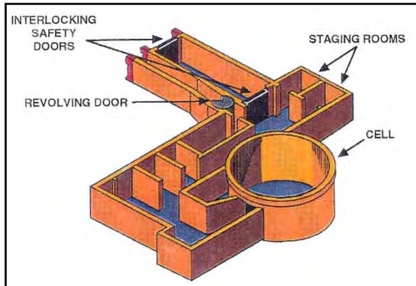
Figure 2-5. Generic representation of a nuclear explosive cell.
