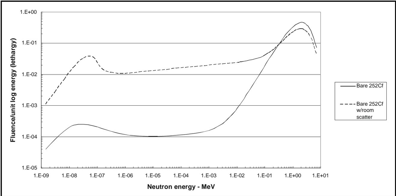
Figure 6-11. Lethargy neutron spectra for <sup>252</sup>Cf calibration source with and without room scatter (IAEA 2001).
