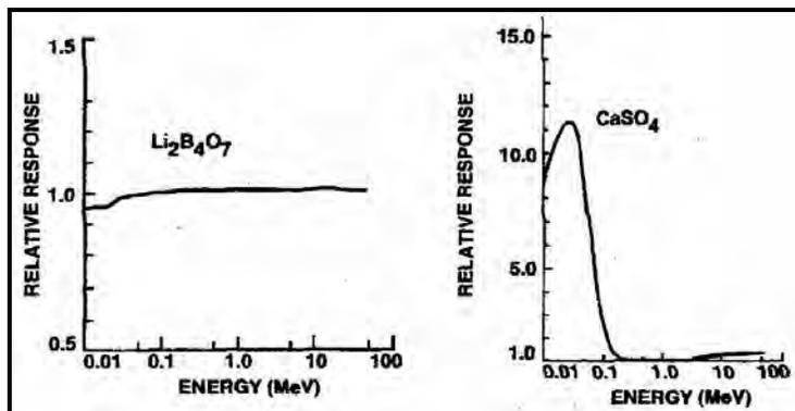
Figure 6-4. Typical photon energy response curves for Li<sub>2</sub>B<sub>4</sub>O<sub>7</sub> and CaSO<sub>4</sub> TLD elements (REEC0 1995b).
