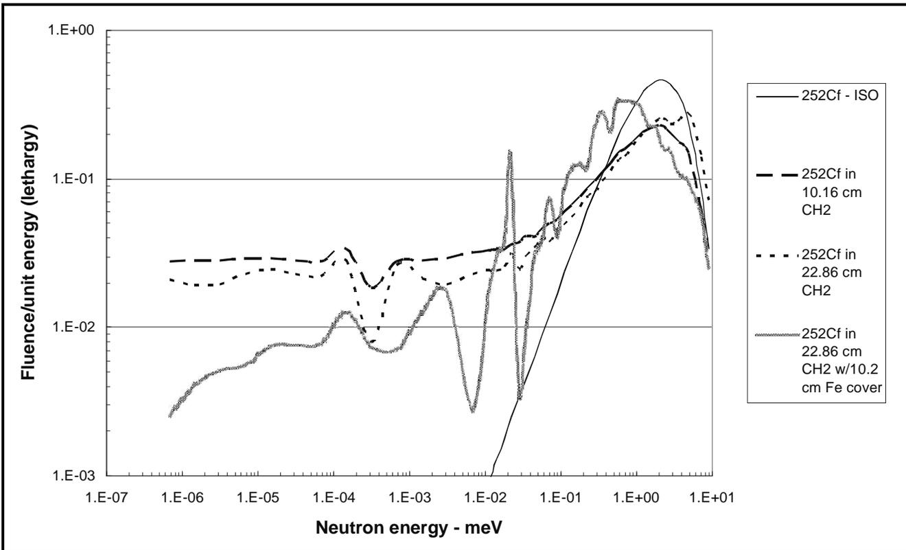
Figure 6-12. Lethargy neutron spectra for <sup>252</sup>Cf with various thickness moderators (IAEA 2001).
