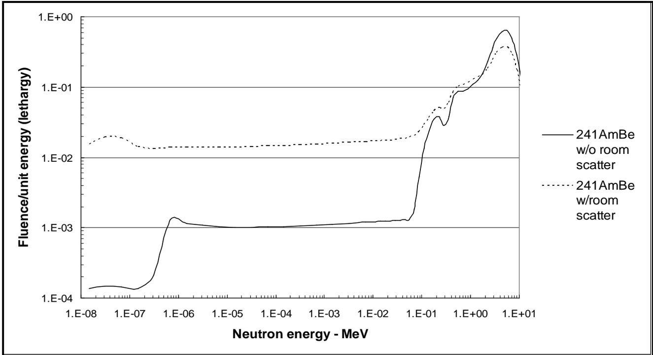
Figure 6-13. Lethargy neutron spectra for an <sup>241</sup>Am-Be calibration source with and without room scatter (IAEA 2001).
