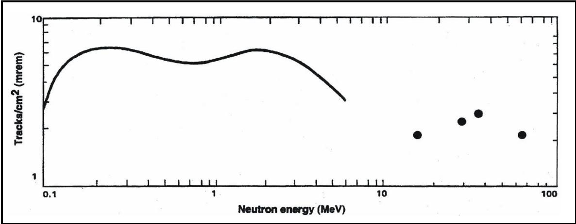
Figure 6-9. Neutron energy response of NTS TED (REECo 1995b).
