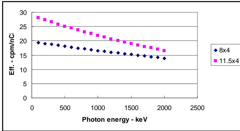
Figure A-2. NaI detector efficiency (cpm per photon nCi).
