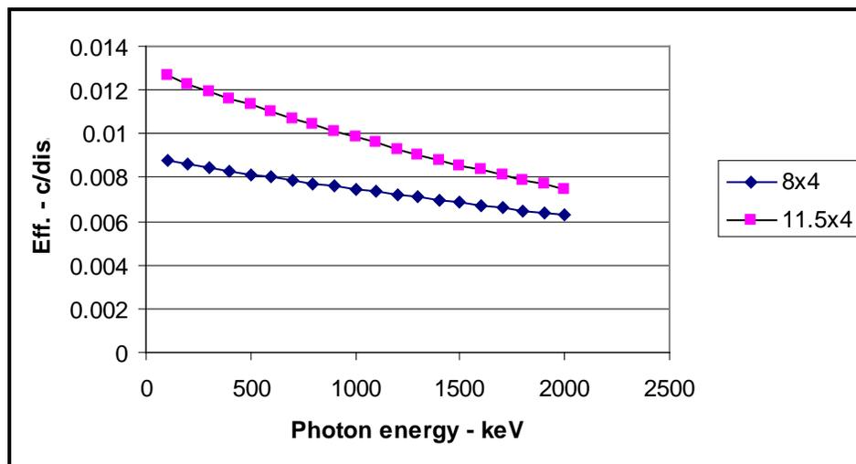
Figure A-1. NaI detector efficiency, counts per photon disintegration.
