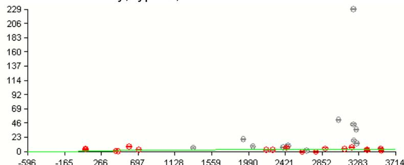
At Adrian Plant, the intake rates of 740 pCi/d inhalation and 15.4 pCi/d ingestions estimated from air samples and a type M assumption overestimate most of the GM data, and overestimate the early 84<sup>th</sup> percentile data. For a type S, assumption the air concentration determined intake rate is a low for the GM data, and underestimates all of the 84<sup>th</sup> percentile data.
