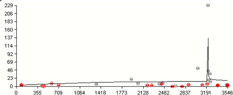
Graphs showing fitting of coworker bioassay data with two inhalation intakes. The first listed intake rate is for the period May 24, 1954 to December 31, 1962. The second listed intake rate is for the period October 1, 1961 to April 11, 1961.
