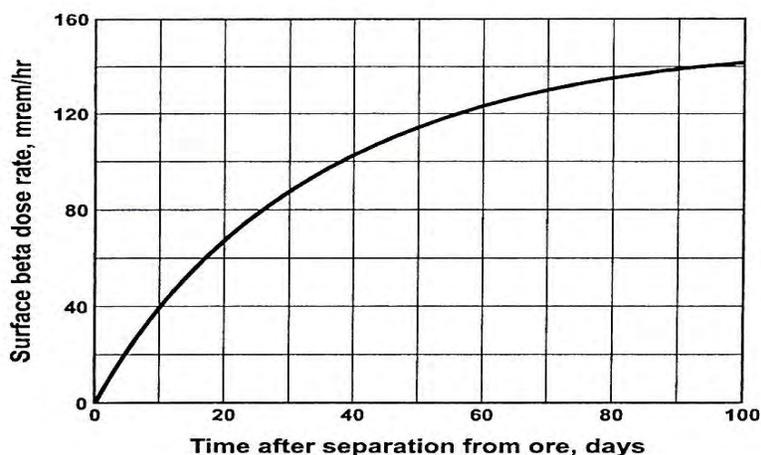
**Figure 3. Beta dose rate from yellowcake separated from ore for more than 100 days as a function of distance from the surface. [Reproduced from US NRC 2002a]**
