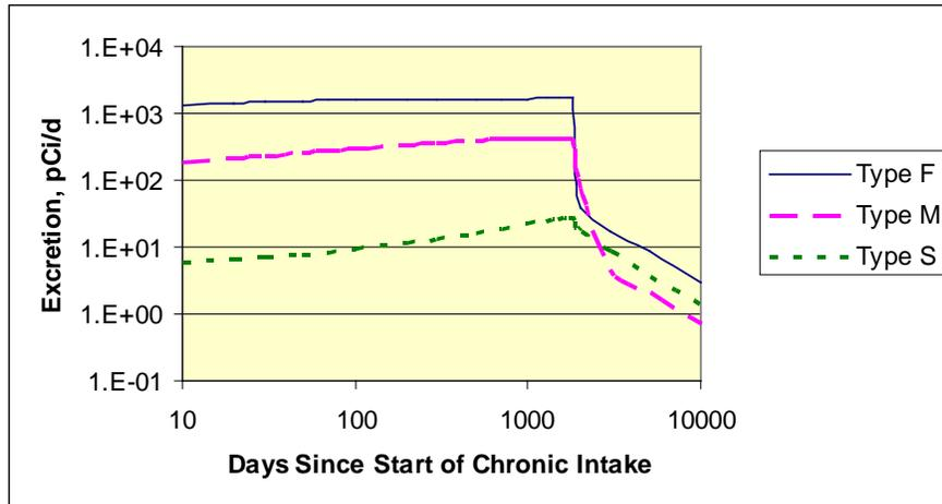
Figure 5-3. Urinary excretion of uranium expected from 1,826-d chronic intake at 6,061 pCi/d inhalation and 124 pCi/d ingestion.
