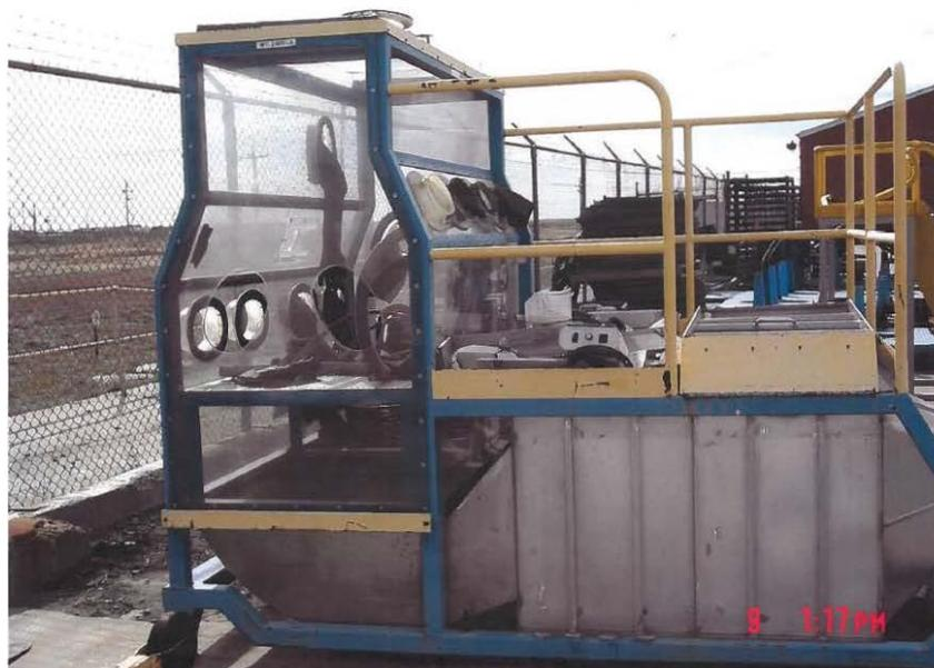
**Figure 3. Gloveboxed Downdraft Table, Installed late-1991, for W55 Dismantlement**
