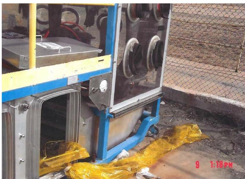
**Figure 4. Closeup of Downdraft Table used for W55 Dismantlement**
