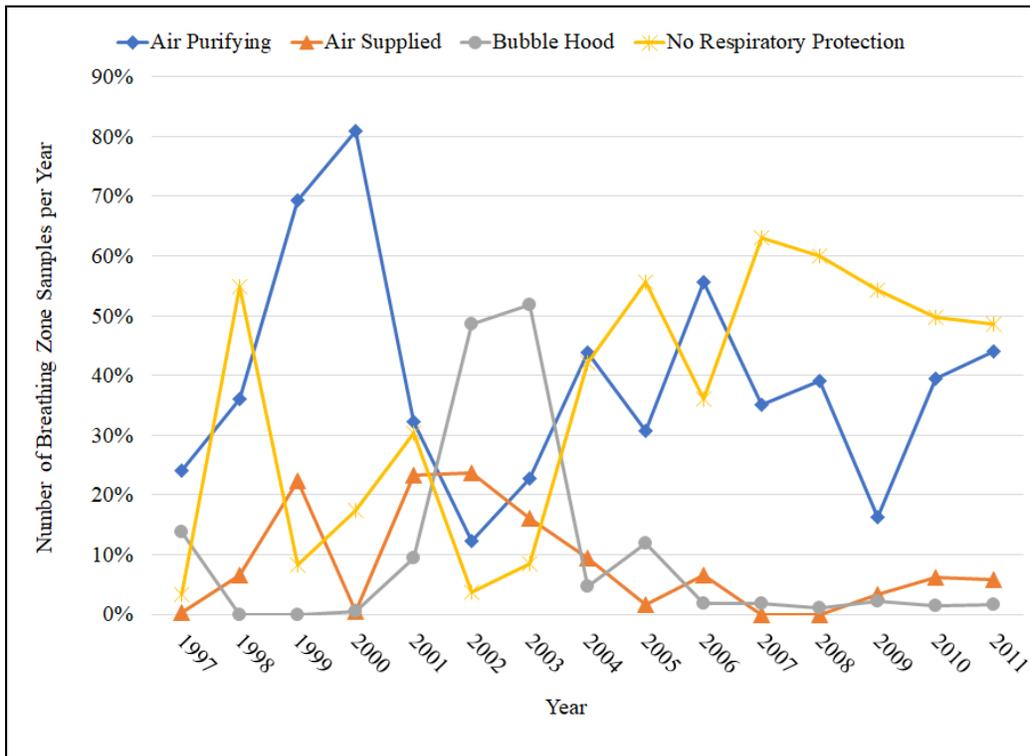
Figure 9. Overall respiratory protection used by workers identified with BZ operation
