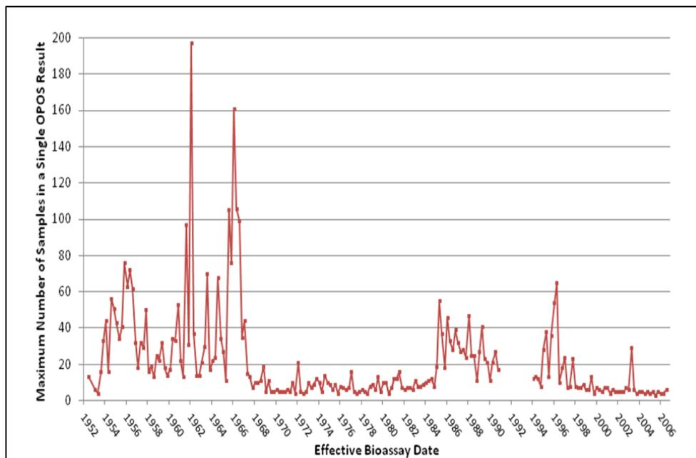
**Figure C-3: Maximum Number of Samples per Quarter Taken from a Single Worker**
