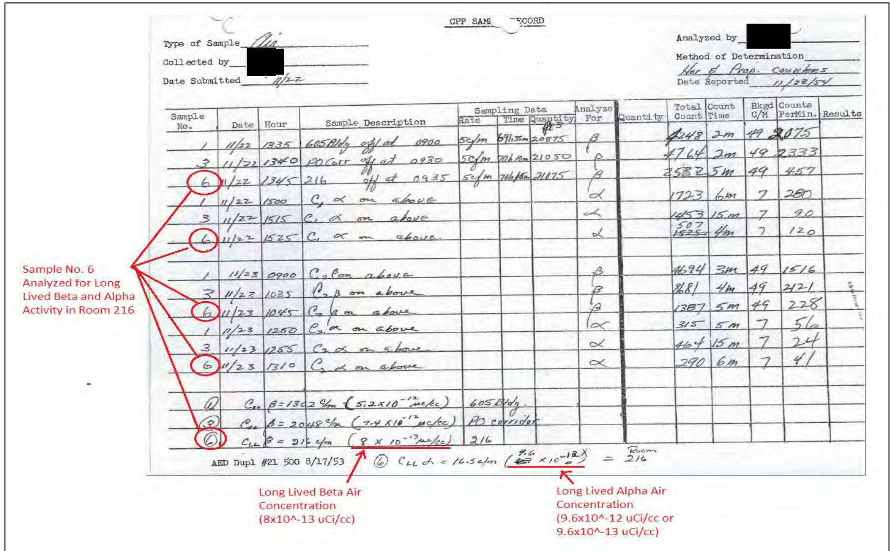
**Figure 19. Air Sample Taken in Room 216 and Analyzed for Both Long-Lived Beta and Alpha Activity on November 30, 1954 (CPP HP Various Dates-b)**
