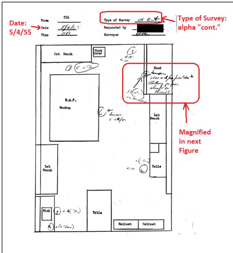
Figure 8. Close Up of Hood in Figure 7 Showing Alpha Contamination Prompting Clean-up Action (CPP HP 1955)
