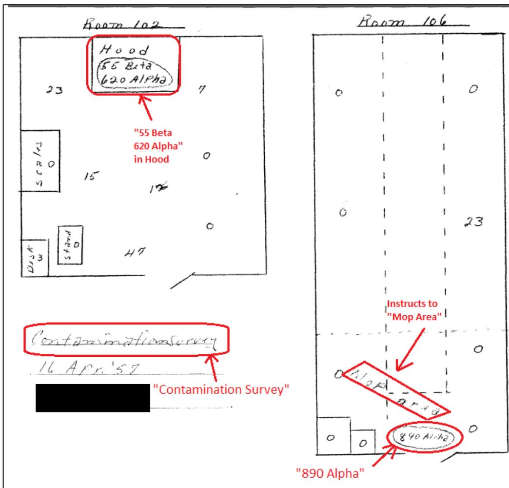
Finally, Figure 14 shows an alpha contamination survey report from Lab 32 in November of 1954. The survey shows that alpha contamination was found on the floors, in a hood, on lab benches, and in a sink. As a result of the survey, it was recommended that the floor be mopped and rechecked. Also, it was recommended that a glass plate on the bench at the spot welder be cleaned, as well as the sink drain boards.
