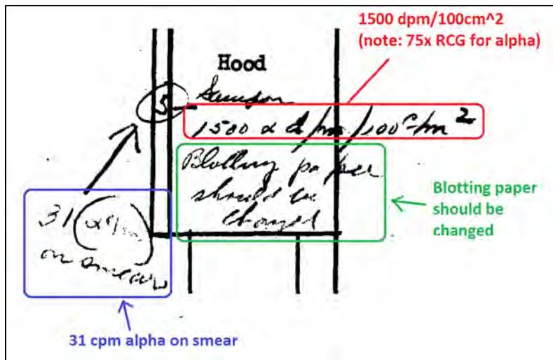
Figure 9 shows an alpha/beta/gamma contamination survey of the X-Cell which occurred in October 1961. As the figure shows, alpha contamination was found in several locations within the cell (sink, desk, bench, hood, table, and floor). Only one location within the X-Cell was noted to have beta/gamma
