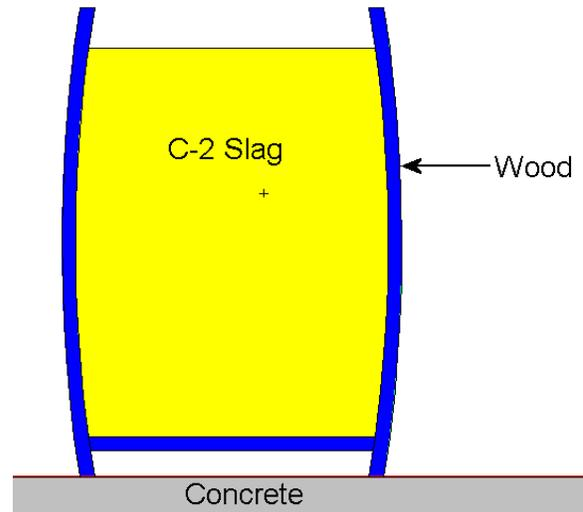
Figure A-2. Cross-Section of MCNP Model of Slag in a Whiskey Barrel
