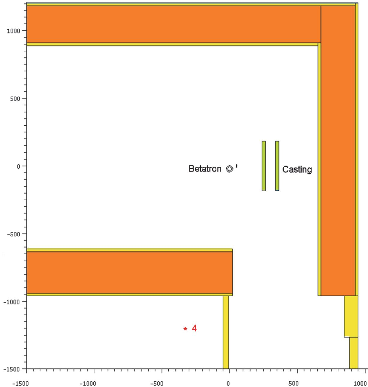
Figure 4. MCNPX Model of Radiography of Steel Casting in New Betatron Building
