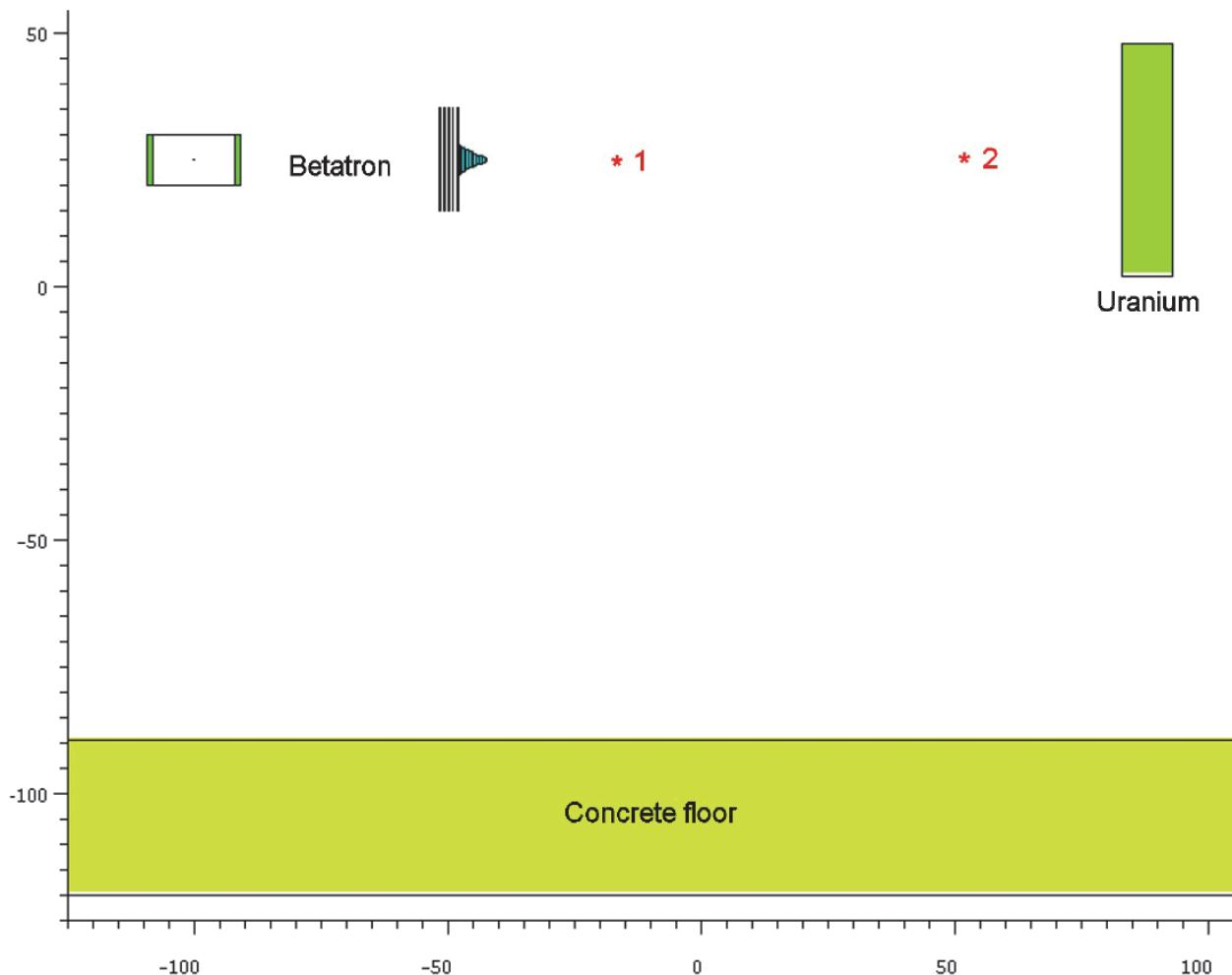
Figure 1. MCNPX Model of Exposure to Irradiated Uranium in Old Betatron Building
