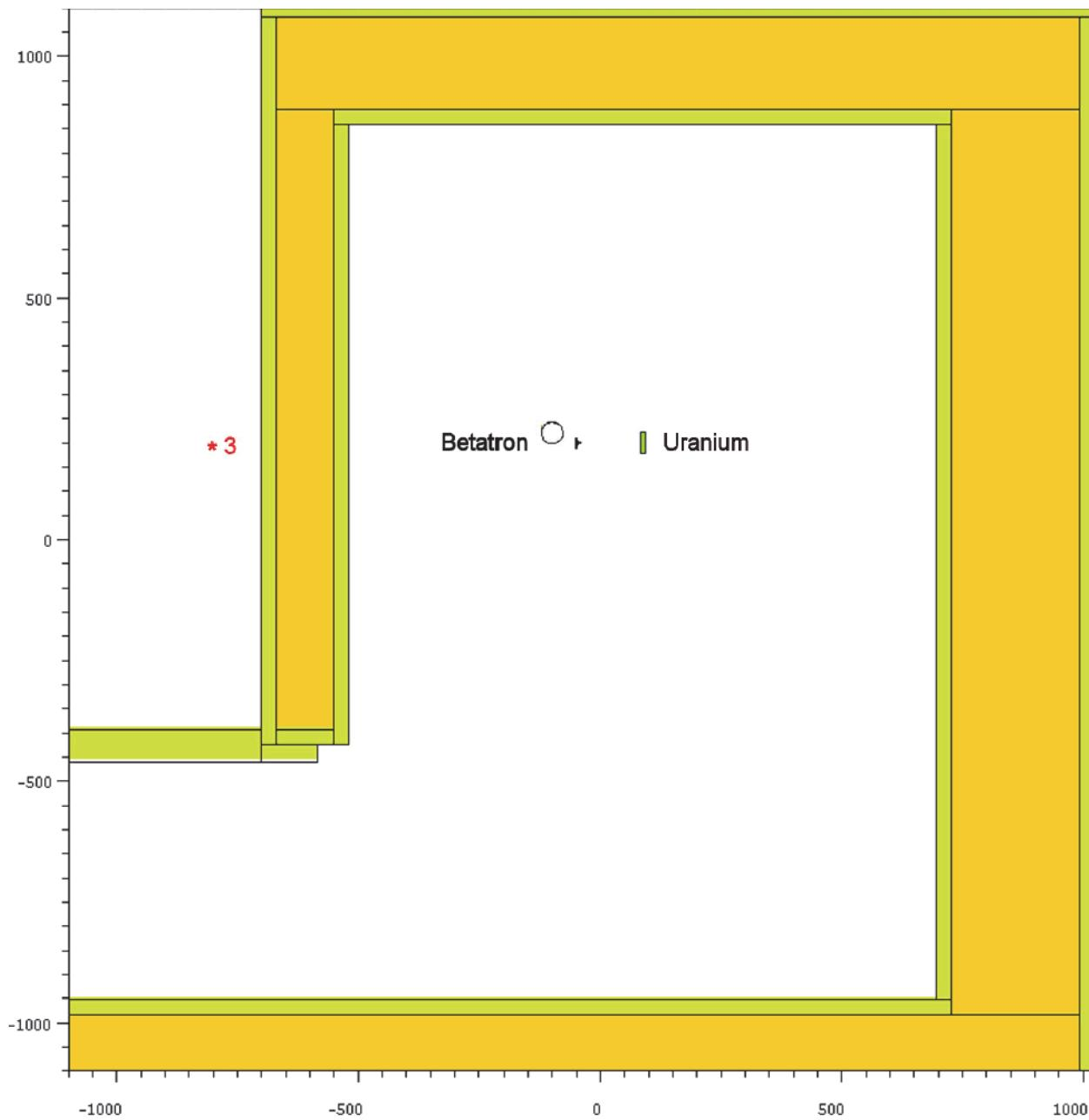
Figure 2. MCNPX Model of Radiography of Uranium in Old Betatron Building (scales in cm)
