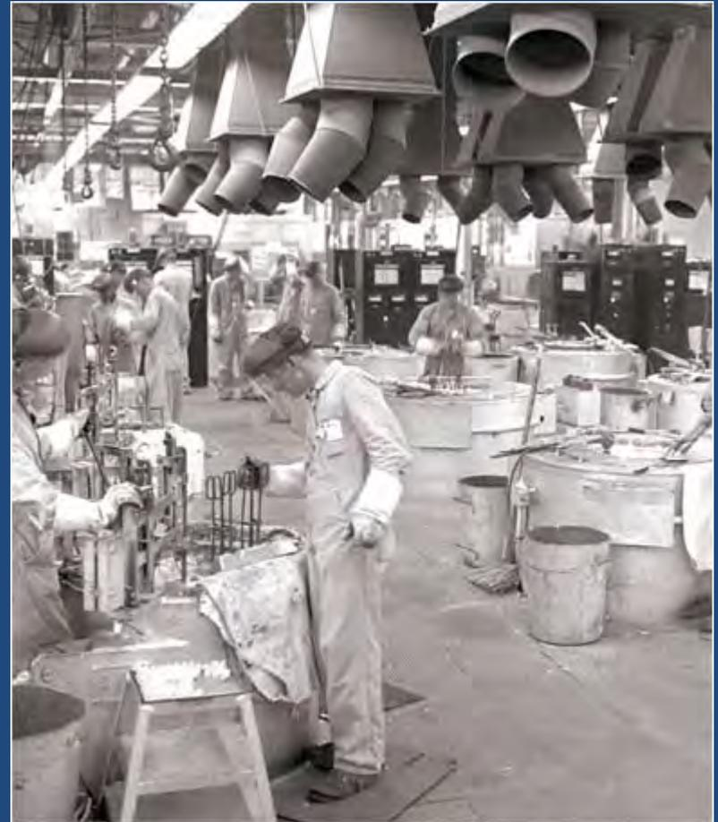
*Interior of canning building illustrating dip canning process,
