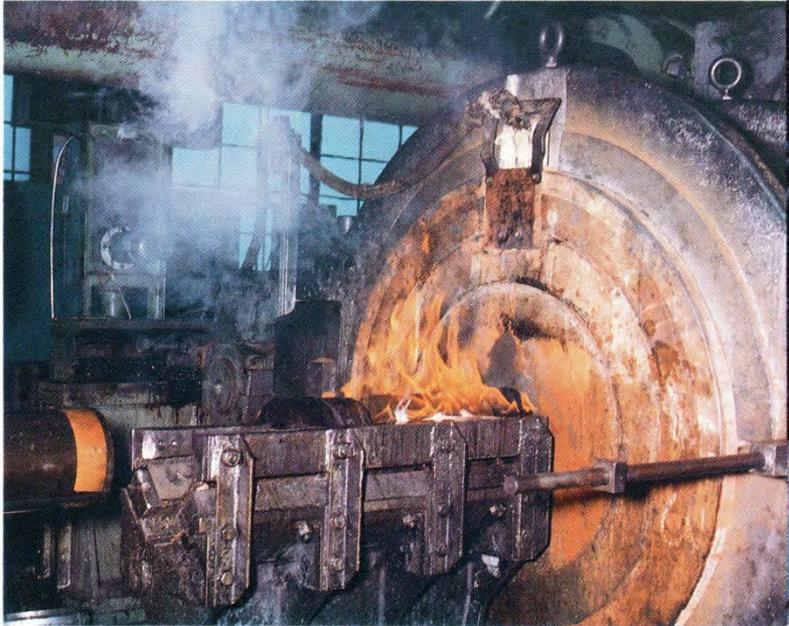
**Billet being forced into extrusion die; flames are lubricant ignited by the hot die.**
