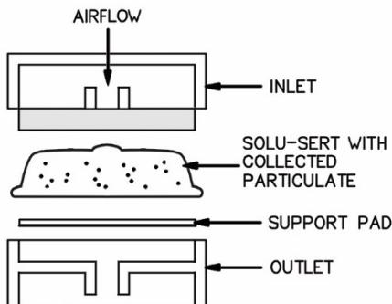
**Figure 1. Schematic of closed-face filter cassette (CFC) aerosol sample collection using an internal capsule (Used with permission of Zefon International, Inc. [8])**
