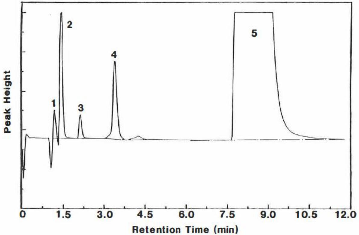
Figure 1. IC separation of chloride (2), chlorite (1), chlorate (3), sulfate (4), and thiosulfate (5).
