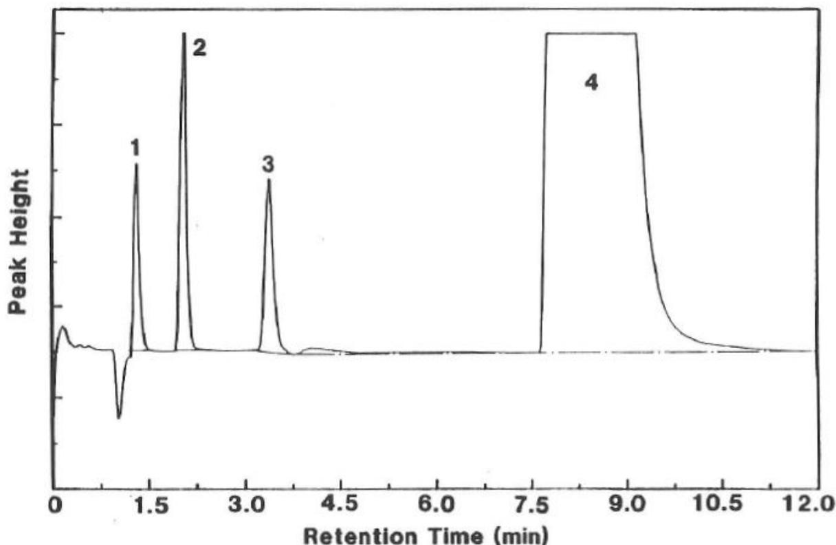
**Figure 2.** IC separation of bromate (1), bromide (2), sulfate (3) and thiosulfate (4).
