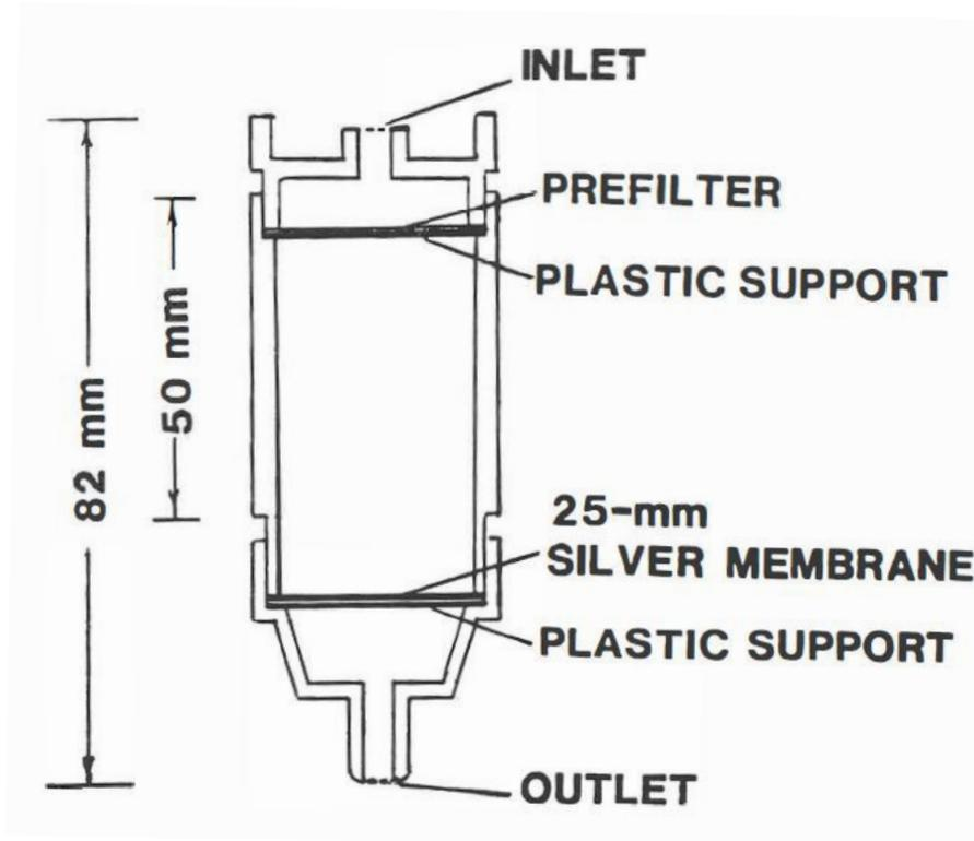
**Figure 3.** Silver filter sampler
