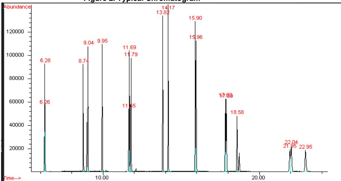
The mass spectrometer is operated in Selected-Ion Monitoring (SIM) mode using a dwell time of 30 ms for each ion. Six different SIM windows are used as shown in Table 4. Table 5 lists ions to use for quantitation, ions for spectral confirmation and internal standard references.
