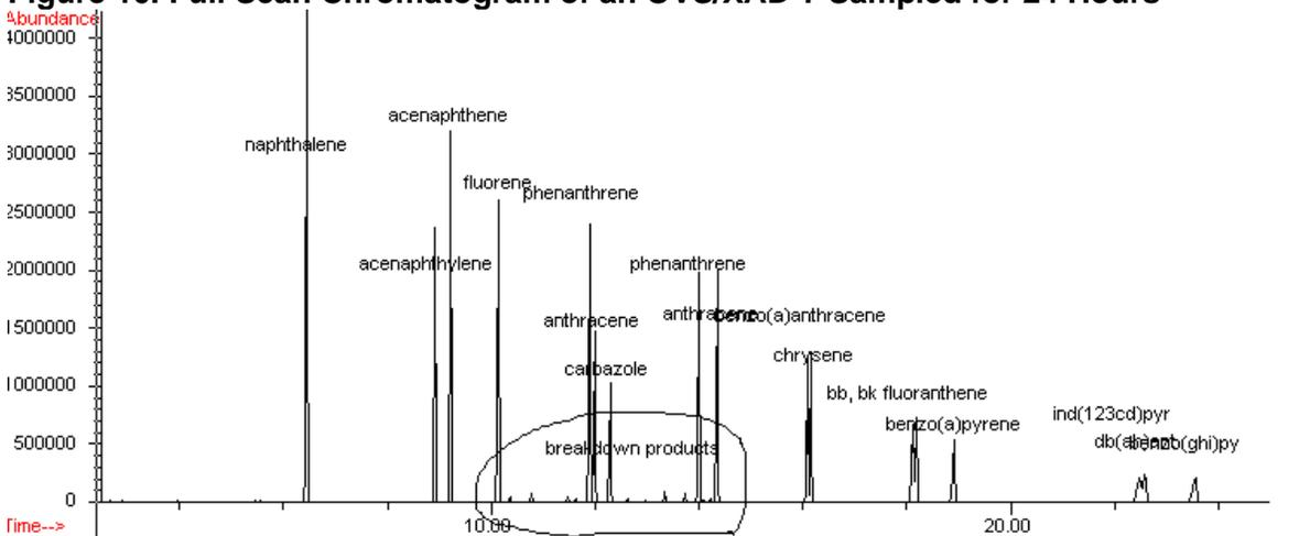
An examination of these full scan data gives evidence that acenaphthylene may in fact be degrading to one or more reaction products during sampling. The evidence is not conclusive; for example, some of these breakdown products appear to be fluorene derivatives, yet fluorene recovery is not significantly inhibited over time. The presence of acenaphthenone as a breakdown product does, however, provide substantiation that acenaphthylene loss may be a result of degradation
