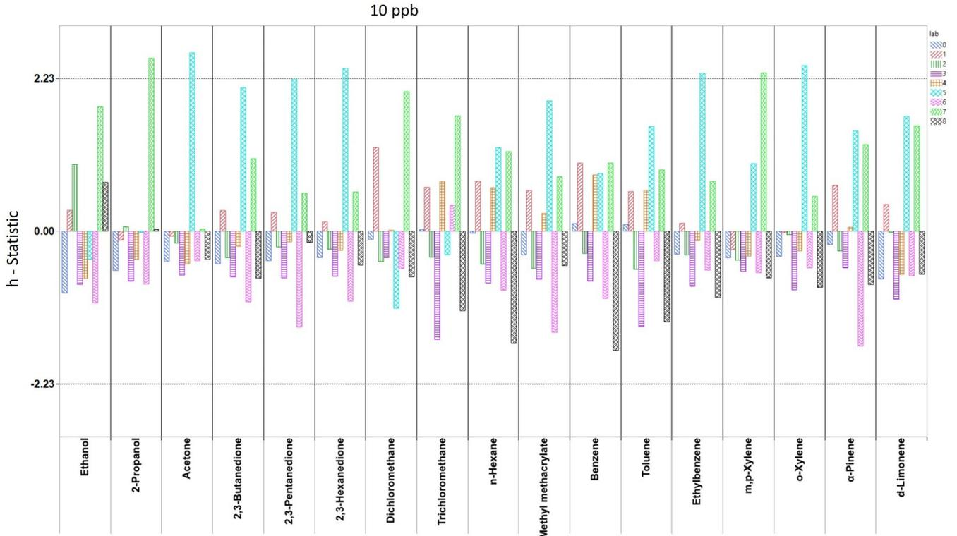
Figure 9. Between-laboratory statistic (h-plot) for 10 ppb nominal level. Dashed line = 2.23 to -2.23 criteria.
