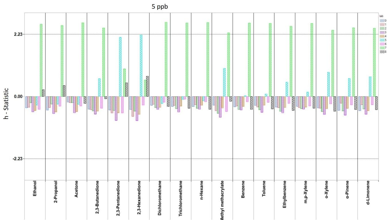
Figure 8. Between-laboratory statistic (h-plot) for 5 ppb nominal level. Dashed line = 2.23 to -2.23 criteria.
