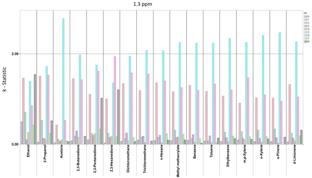
Figure 6. Within-laboratory statistic (k-plot) for 1.3 ppm nominal level. Dashed line = 2.09 criterion.
