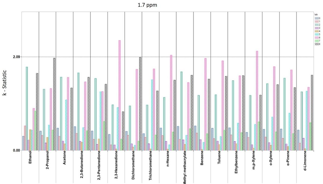
Figure 7. Within-laboratory statistic (k-plot) for 1.7 ppm nominal level. Dashed line = 2.09 criterion.
