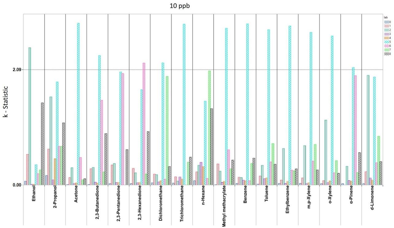
Figure 3. Within-laboratory statistic (k-plot) for 10 ppb nominal level. Dashed line = 2.09 criterion.
