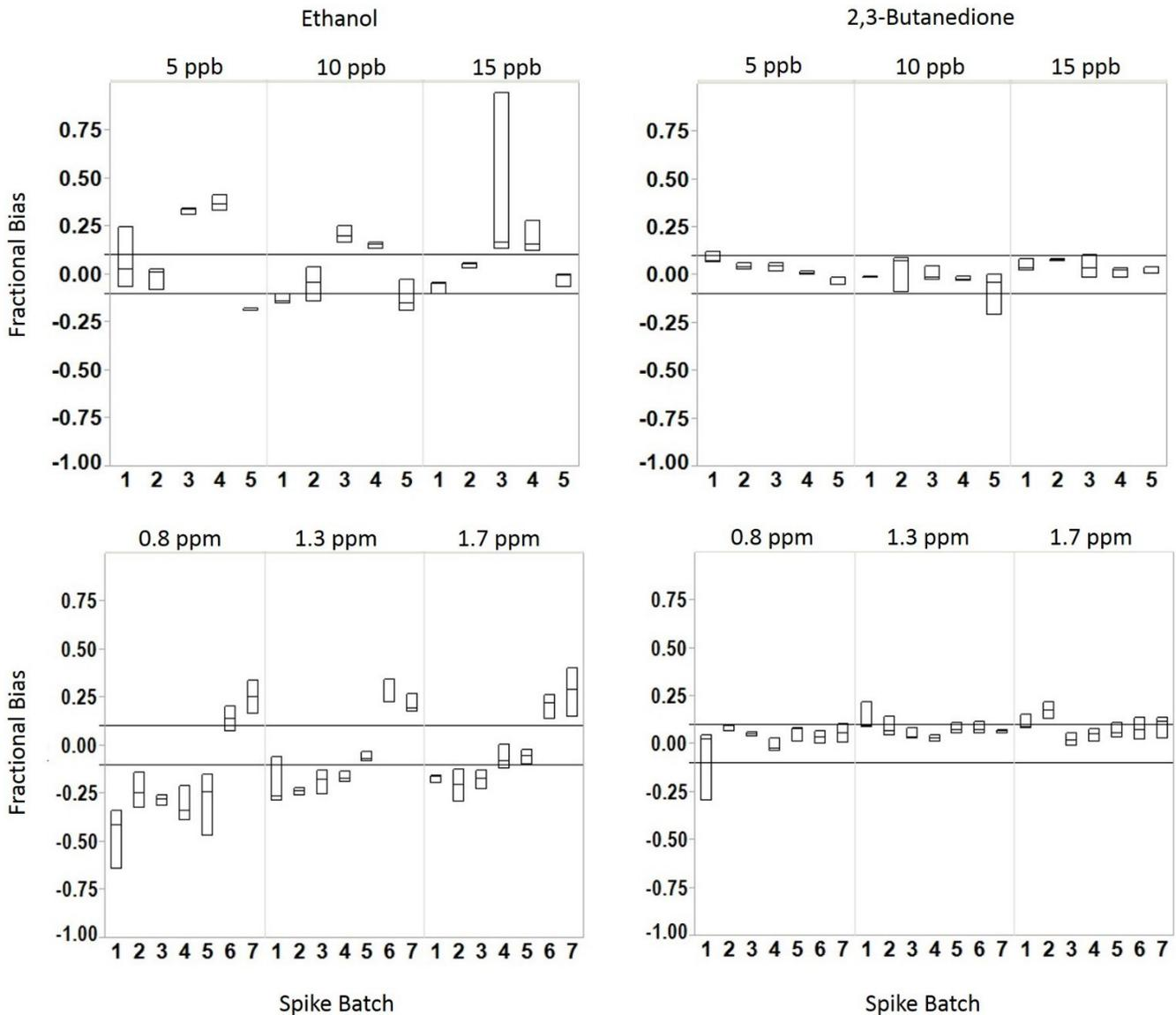
Figure 1. Representative box plots of reference laboratory bias across spike batches and nominal level for ethanol (left) and 2,3-butanedione (right).  $n=3$  per box. Solid line represents  $\pm 10\%$  bias criterion.
