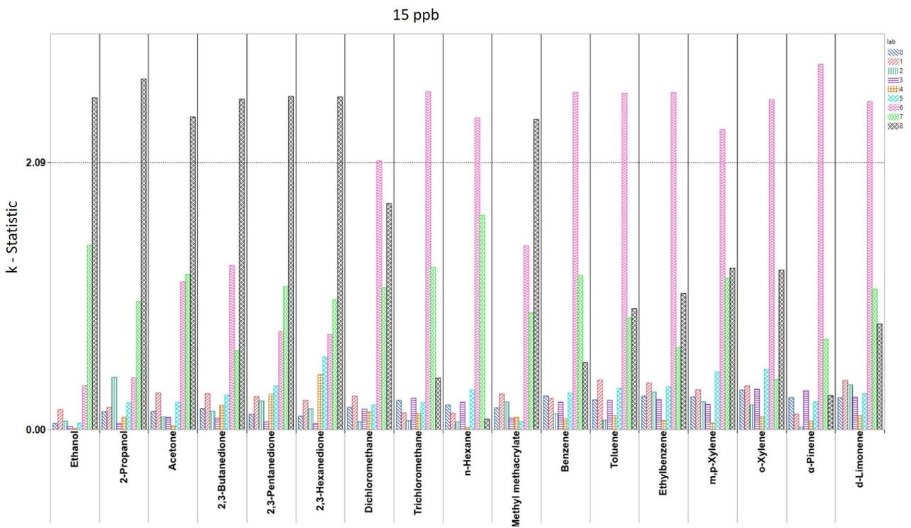
Figure 4. Within-laboratory statistic (k-plot) for 15 ppb nominal level. Dashed line = 2.09 criterion.
