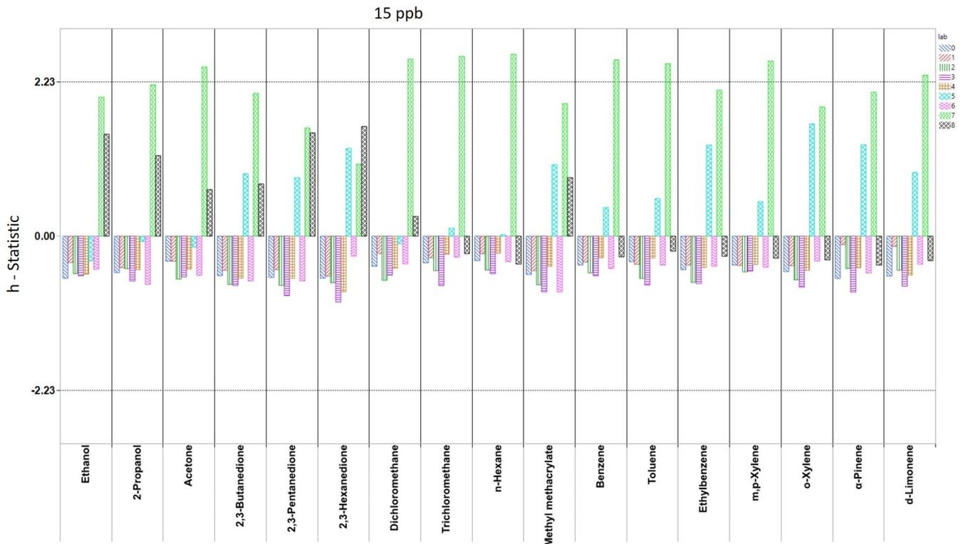
Figure 10. Between-laboratory statistic (h-plot) for 15 ppb nominal level. Dashed line = 2.23 to -2.23 criteria.
