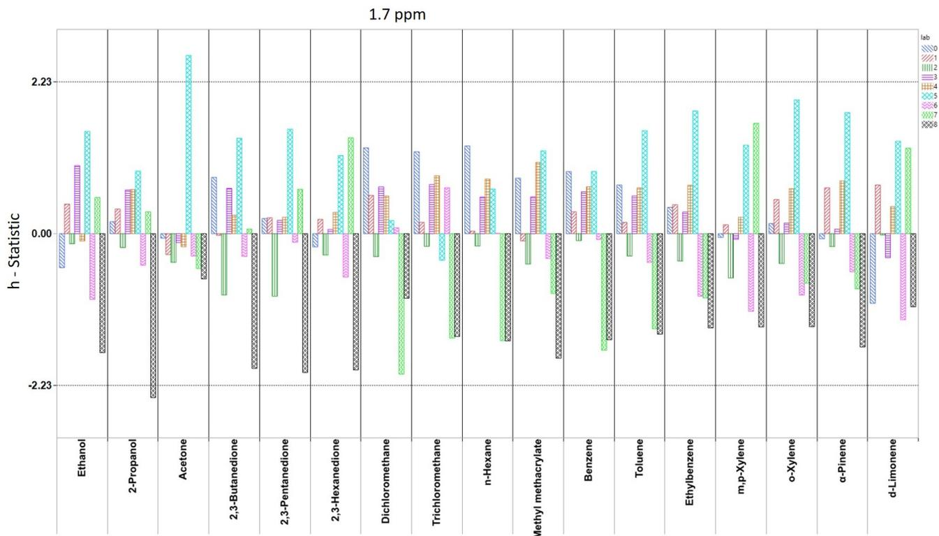
Figure 13. Between-laboratory statistic (h-plot) for 1.7 ppm nominal level. Dashed line = 2.23 to -2.23 criteria.
