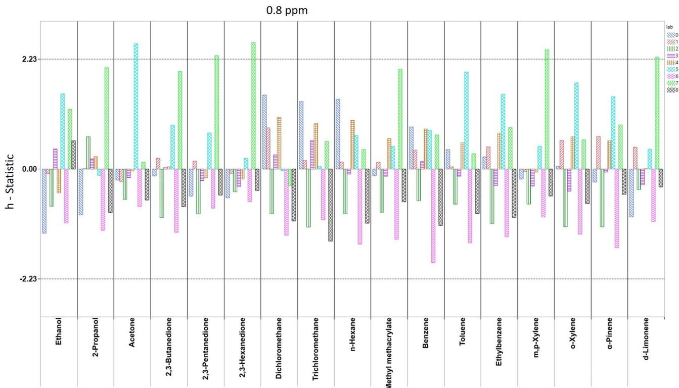
Figure 11. Between-laboratory statistic (h-plot) for 0.8 ppm nominal level. Dashed line = 2.23 to -2.23 criteria.
