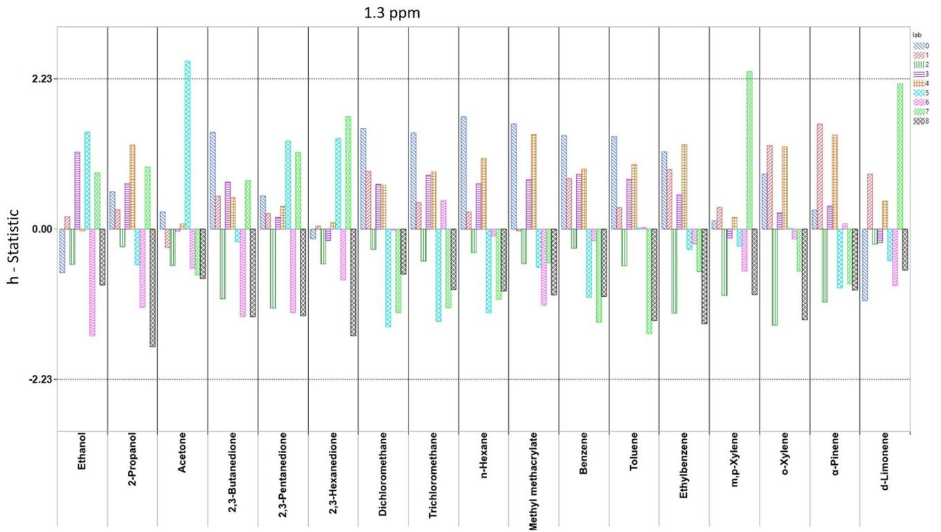
Figure 12. Between-laboratory statistic (h-plot) for 1.3 ppm nominal level. Dashed line = 2.23 to -2.23 criteria.
