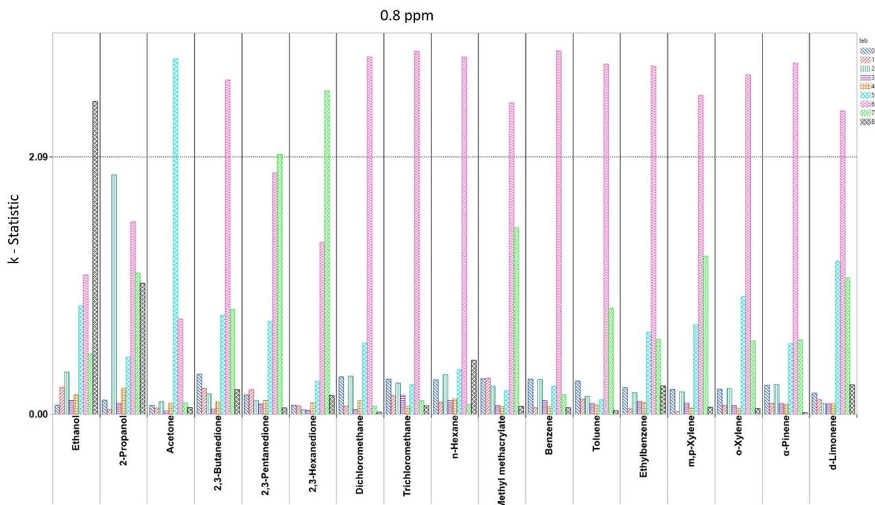
Figure 5. Within-laboratory statistic (k-plot) for 0.8 ppm nominal level. Dashed line = 2.09 criterion.
