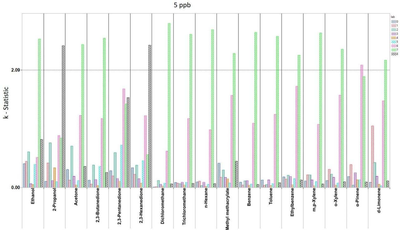
Figure 2. Within-laboratory statistic (k-plot) for 5 ppb nominal level. Dashed line = 2.09 criterion.
