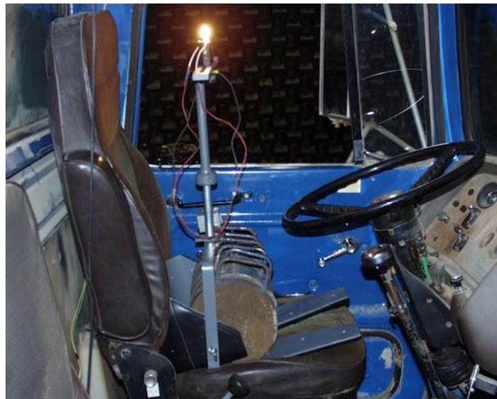
***Figure 3. Light Support Device Test Setup.***
