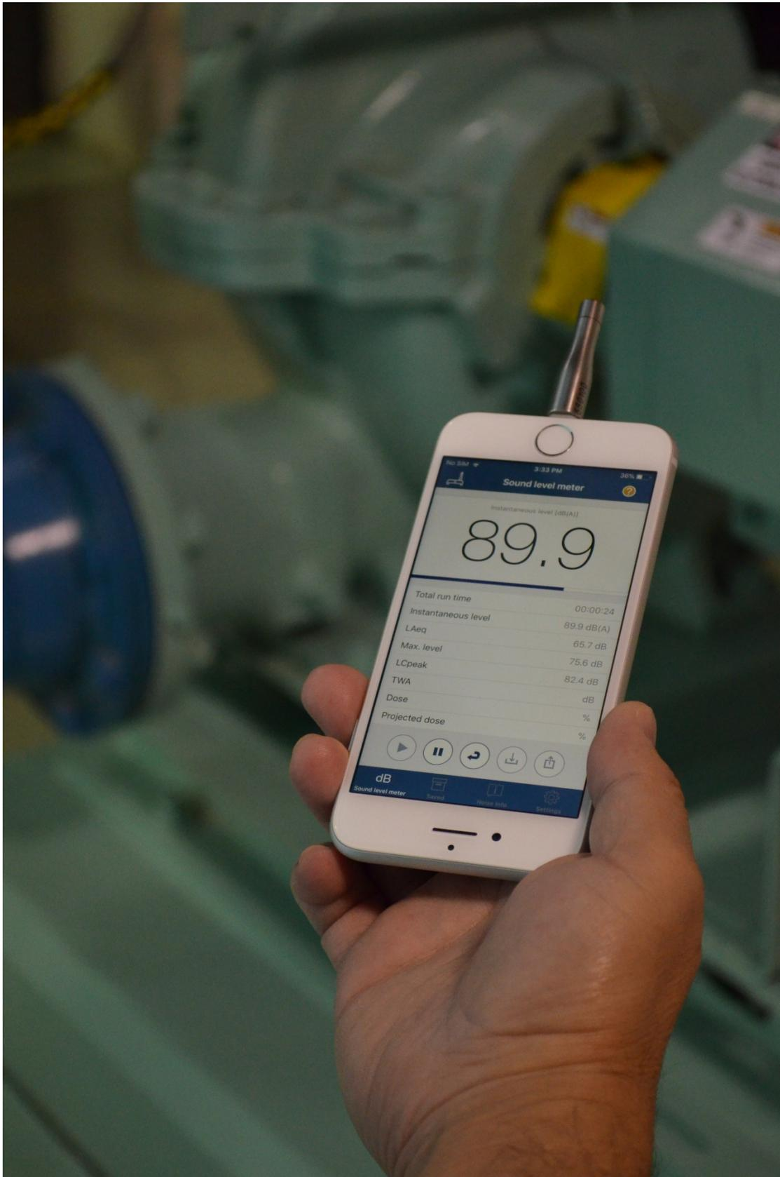
Figure 1. The main screen of the NIOSH SLM app (shown with an external microphone on iPhone 8)
