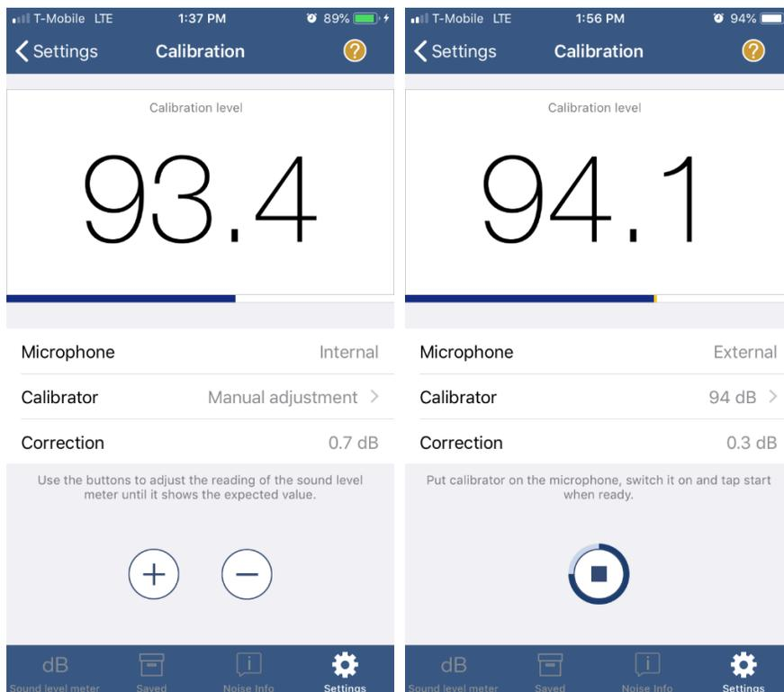
The image below shows how to calibrate the app with an external microphone using an acoustical calibrator:
