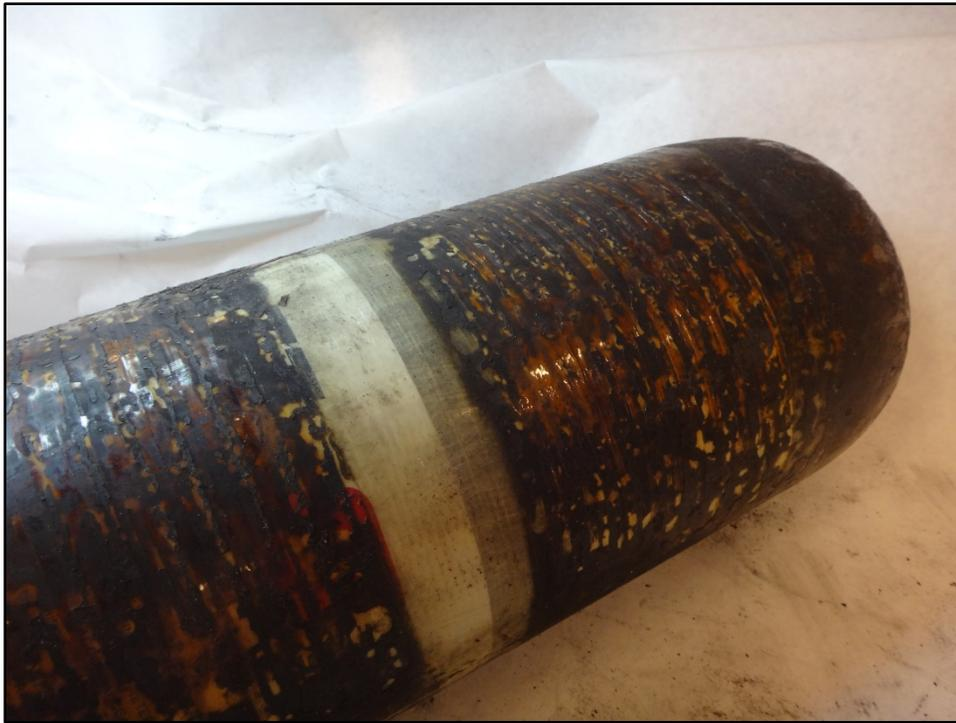
**Figure 27: Heat damage to cylinder**
