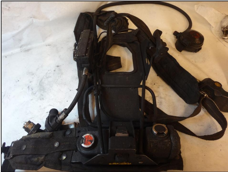
**Figure 18: PASS control module heat damage**
