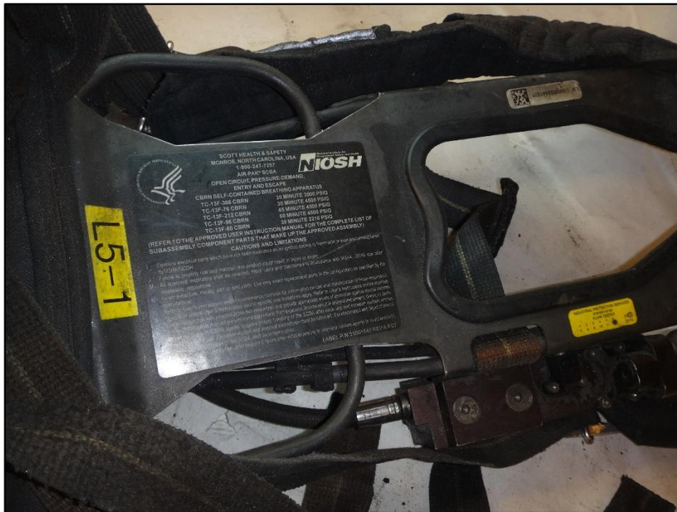
Figure 19: Interior side of backframe assembly
