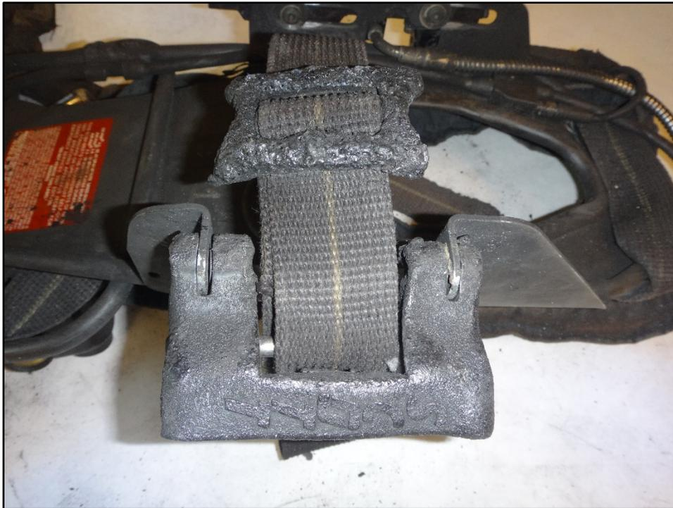
**Figure 21: Melted cylinder strap**
