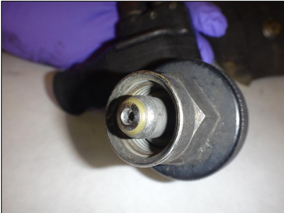
**Figure 14: O-ring and threads of cylinder attachment**
