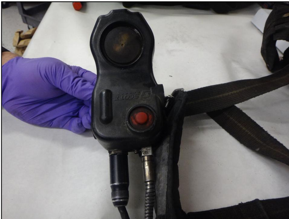
**Figure 16: Front of PASS console**
