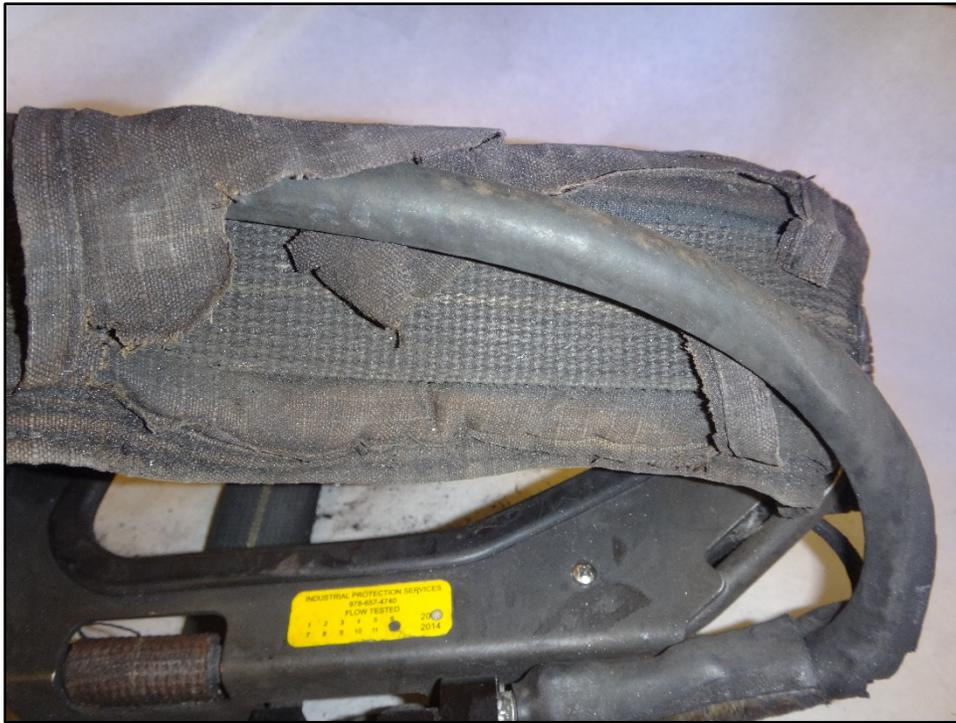
**Figure 23: Left side shoulder strap heat damage**
