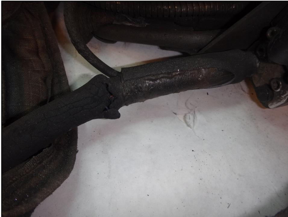
**Figure 10: Low pressure hose sheath heat damage**
