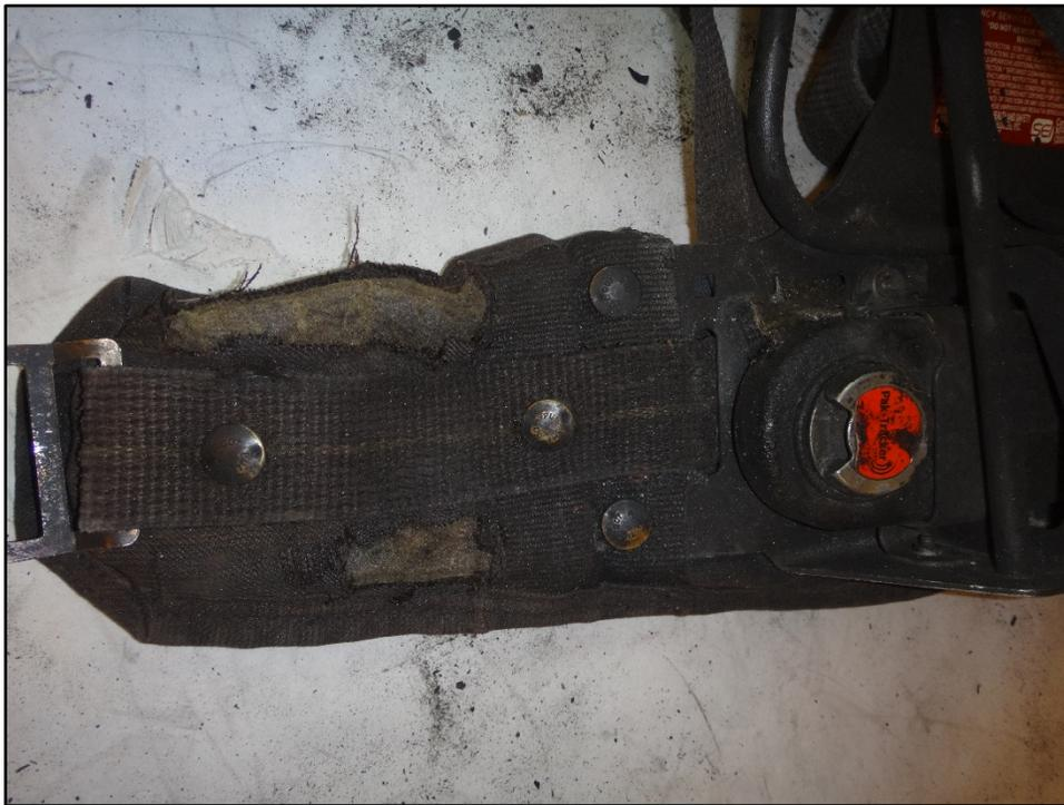
**Figure 24: Left side waist strap heat damage**
