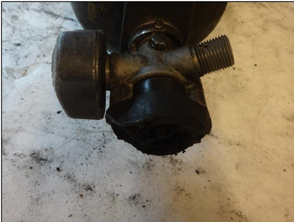
**Figure 26: Gauge, rubber bumper and valve**
