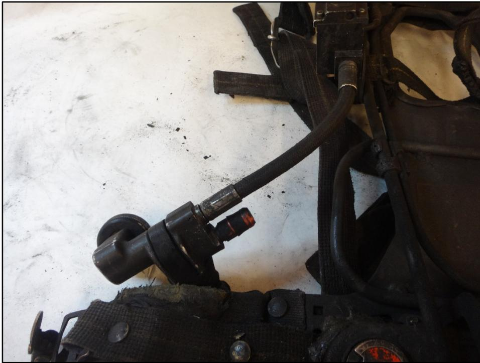
**Figure 13: High pressure hose and cylinder attachment**
