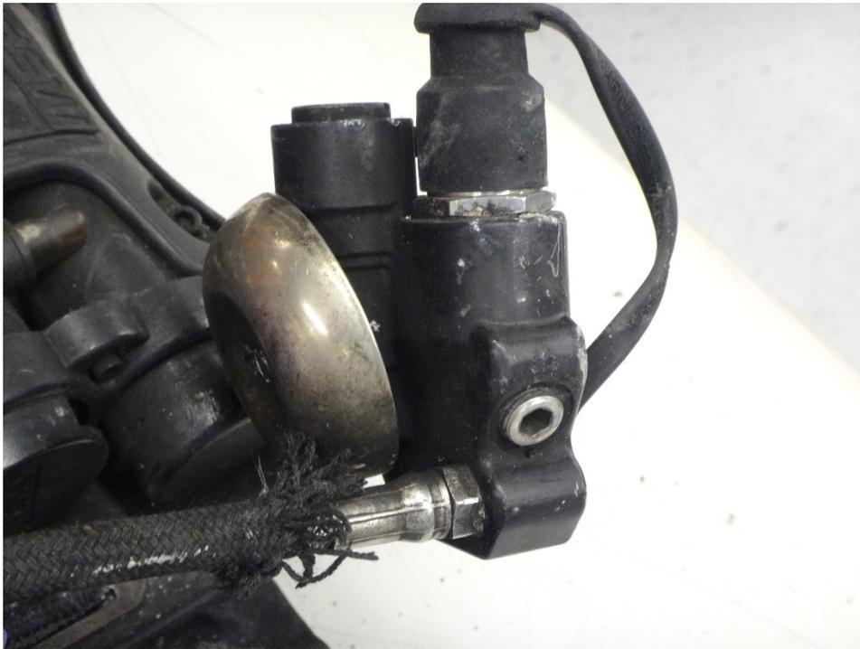
**Figure 10224: Dust cap for the RIC UAC system connector**
