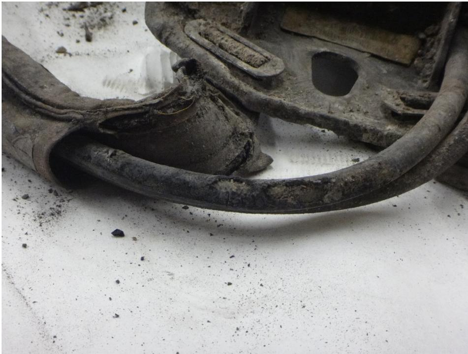
**Figure 71: Damaged medium pressure line and shoulder strap**
