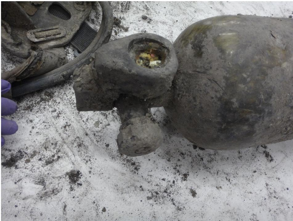
**Figure 726: Damaged cylinder gauge**
