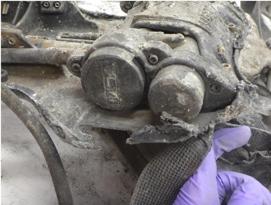
**Figure 677: Left view of damage to control module and backframe**
