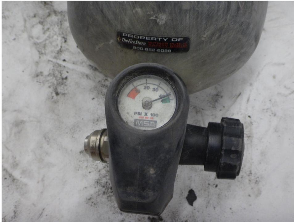
**Figure 27: Cylinder gauge**
