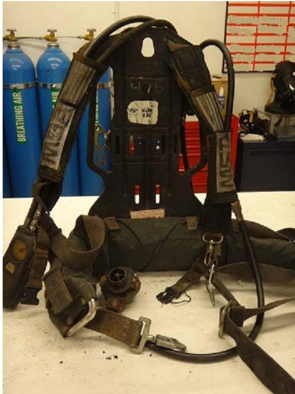
**Figure 52: Top view of backframe, straps, and buckles**
