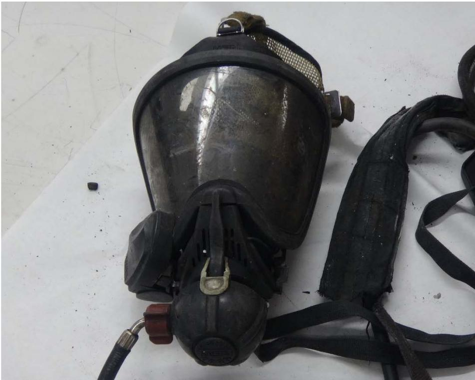
**Figure 91: Top view of facepiece with attached MMR**
