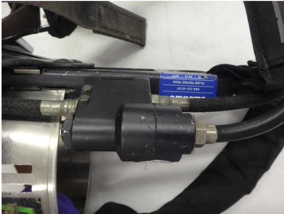
**Figure 12244: Outside view of pressure reducer assembly**
