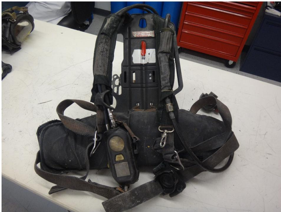
**Figure 11133: Top view of waist belt, straps, and buckles**
