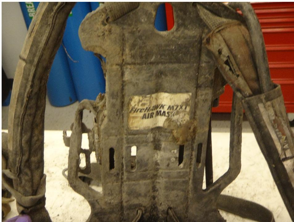
**Figure 82: Labels on back of backframe**
