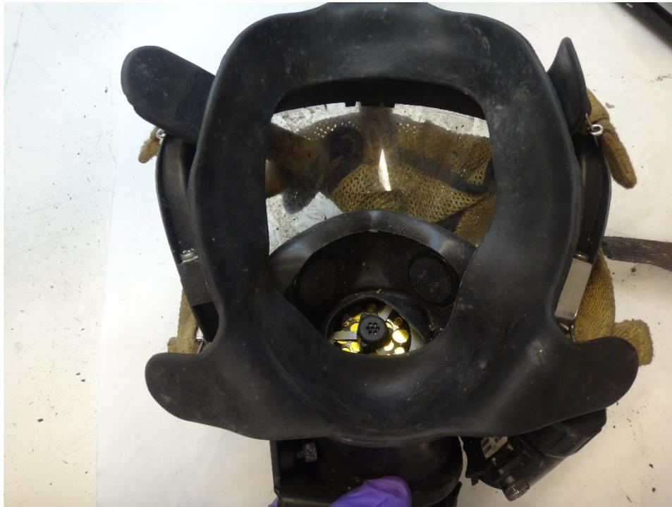
**Figure 92: Inside view of facepiece and nosecup**
