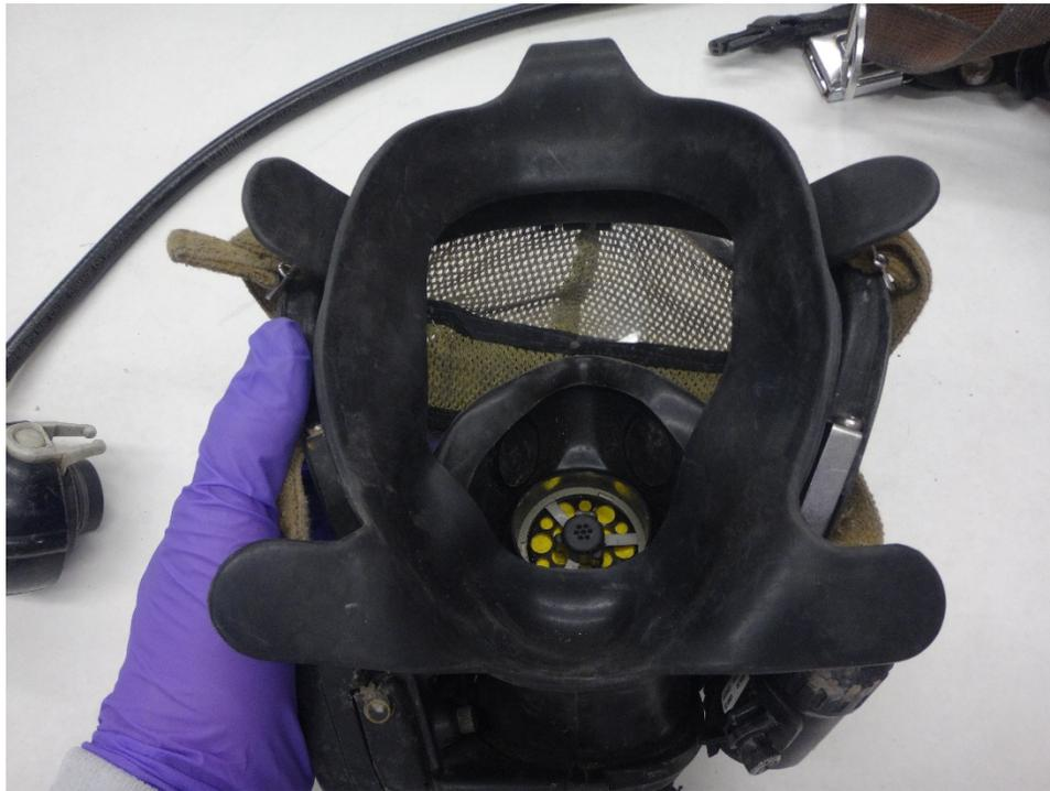
**Figure 1180: Inside view of facepiece and nosecup**
