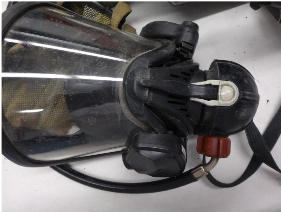
**Figure 1179: Top view of facepiece with attached MMR**
