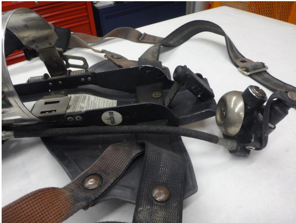
**Figure 12345: High pressure hose, cylinder attachment, and bell assembly**
