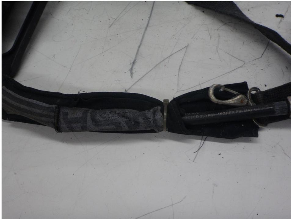
Figure 9820: Low pressure line running through shoulder strap
