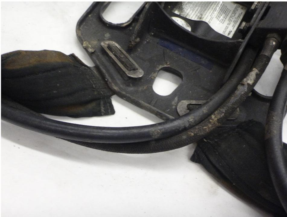
**Figure 43: Heat damage and melted debris on medium pressure lines to PASS console**
