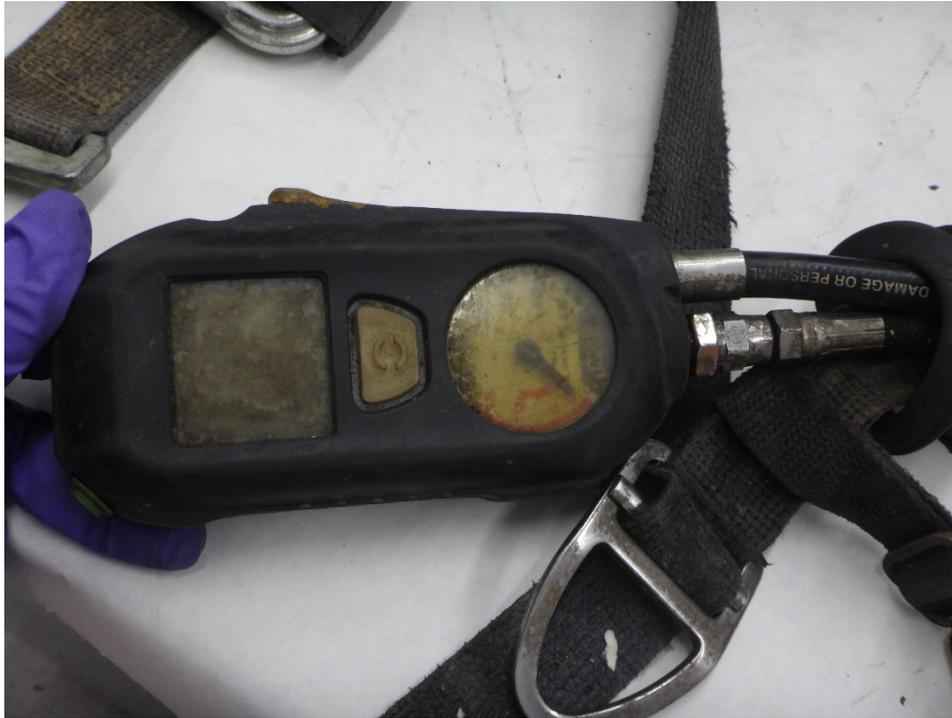
Figure 44: PASS control console
