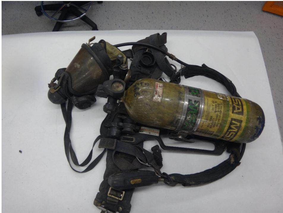
**Figure 30: All components of SCBA unit #13 to be examined**
