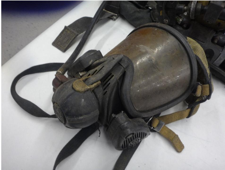
**Figure 34: Top view of facepiece with MMR attached**
