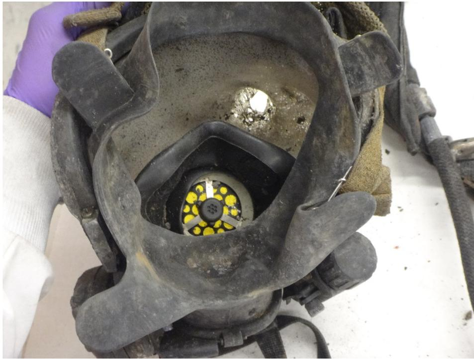
**Figure 61: Inside view of facepiece and nosecup**
