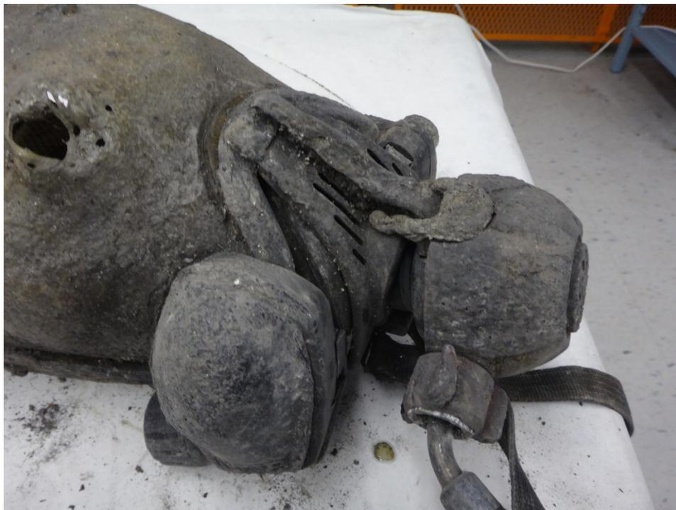
**Figure 62: MMR attached to facepiece**
