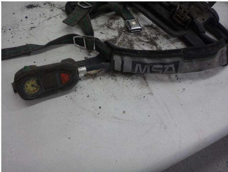
**Figure 10: PASS console and medium pressure line**
