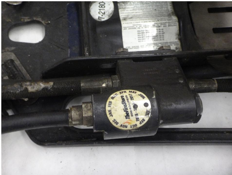
Figure 38: Inside view of pressure reducer assembly with “The Fire Store” Sticker
