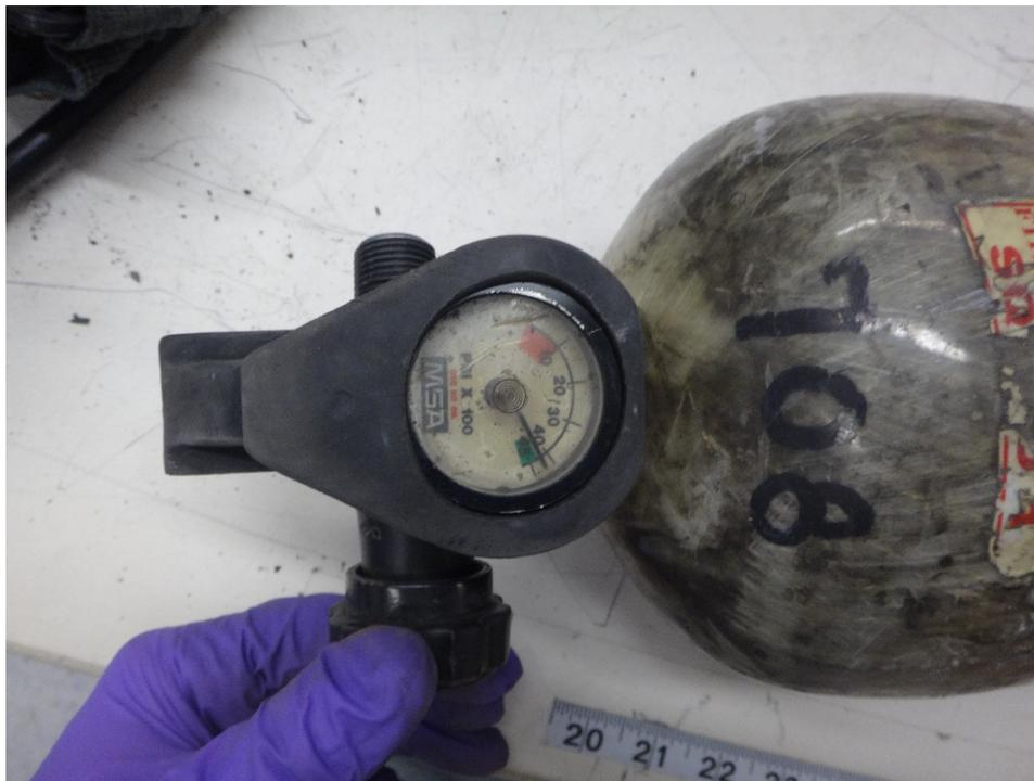
Figure 11335: Cylinder gauge
