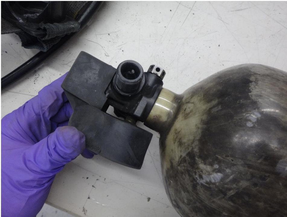
**Figure 1146: Cylinder threads**
