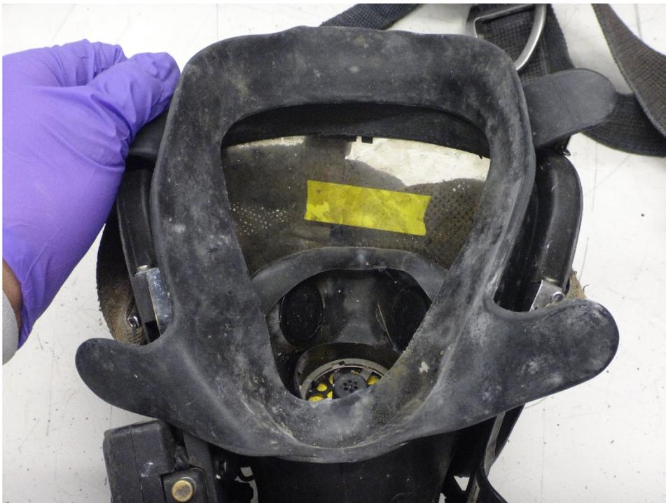
**Figure 957: Inside view of facepiece and nosecup**
