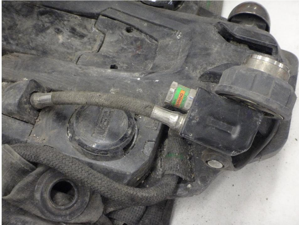
**Figure 12: High pressure hose and cylinder attachment**
