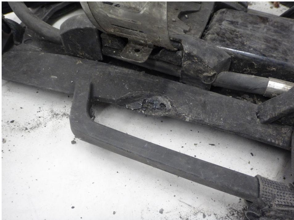
**Figure 20: Heat damage to side rail**
