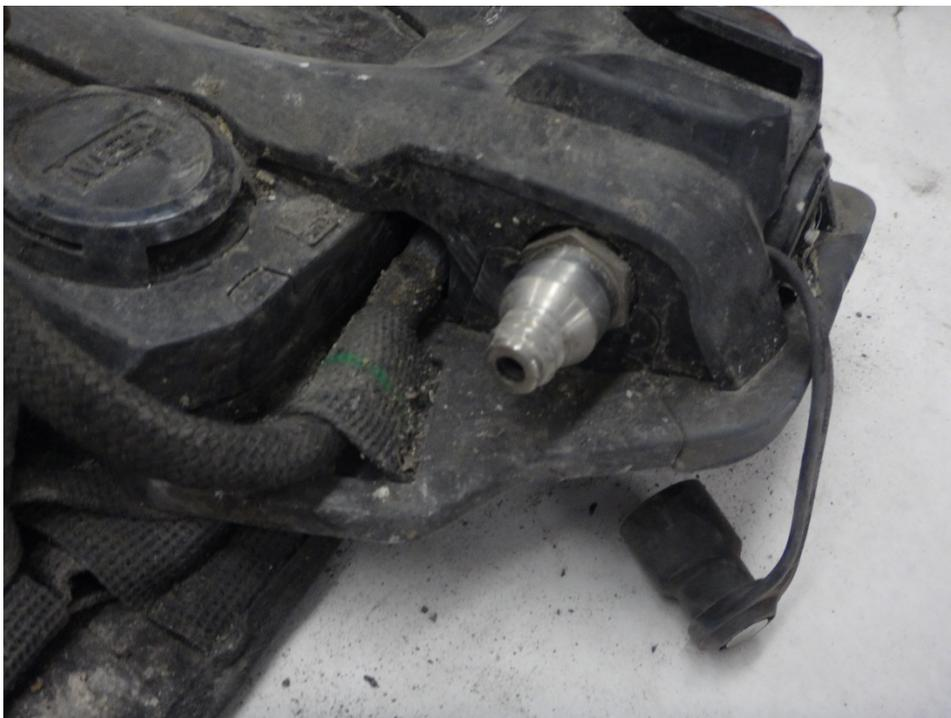
**Figure 16: Quick-Fill adapter**
