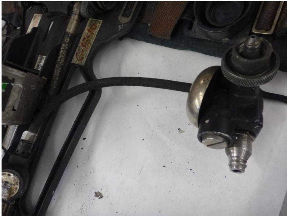
**Figure 808: High pressure line, bell assembly, and cylinder attachment**
