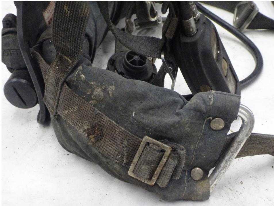
**Figure 50: Heat damage to waist belt**
