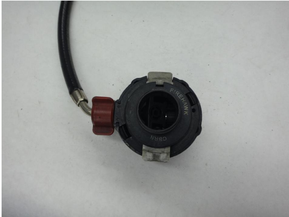
**Figure 11941: Inside flange of MMR with identifying markings**
