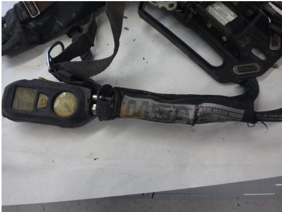
**Figure 99: Medium pressure line and PASS console**
