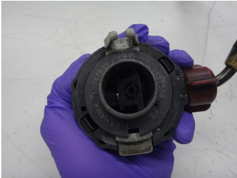
**Figure 968: Inside flange of MMR with identifying markings**
