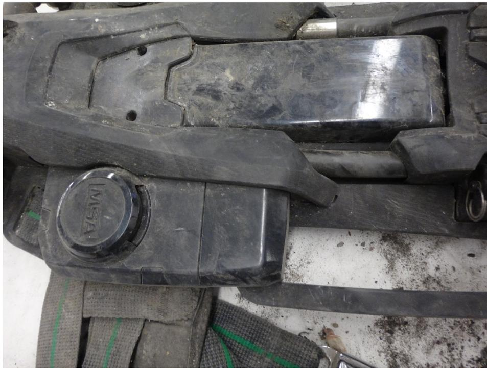
**Figure 9: Low pressure hose attachment to SCBA**
