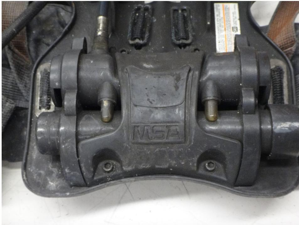
**Figure 1068: Top view of control module**
