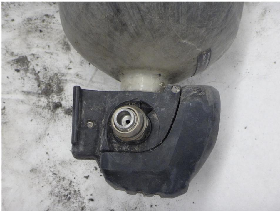
**Figure 28: Cylinder assembly and quick connect adapter**
