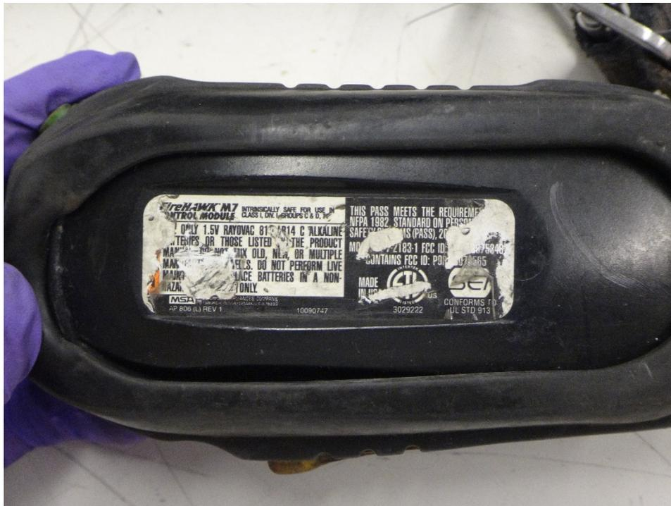
Figure 1057: Back view of PASS console
