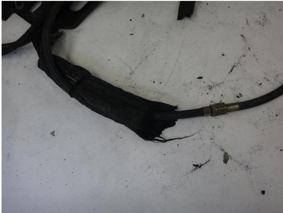
**Figure 95: Low pressure line, connecting link, and damaged shoulder strap**
