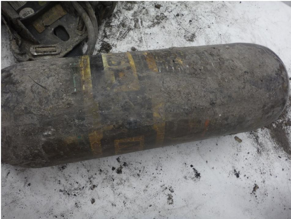
**Figure 759: Melted debris on cylinder**
