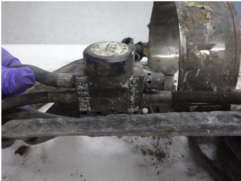
**Figure 66: Pressure reducer assembly and "The Fire Store" sticker**
