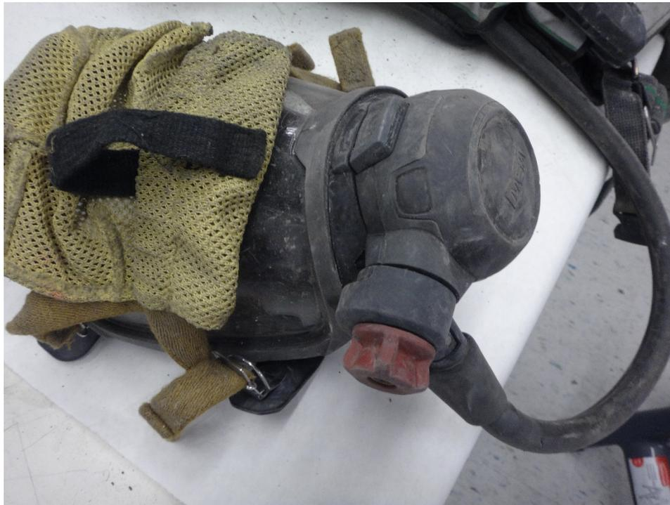
**Figure 5: MMR attached to facepiece**
