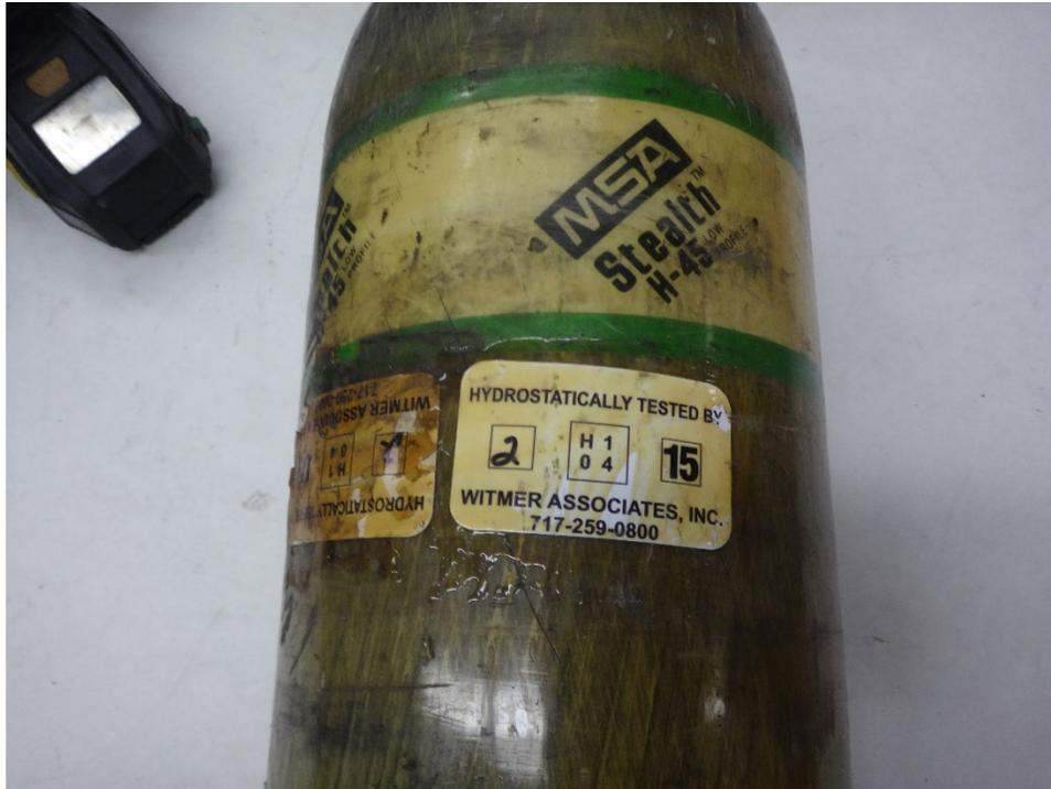
Figure 1335: Hydrostatic test sticker
