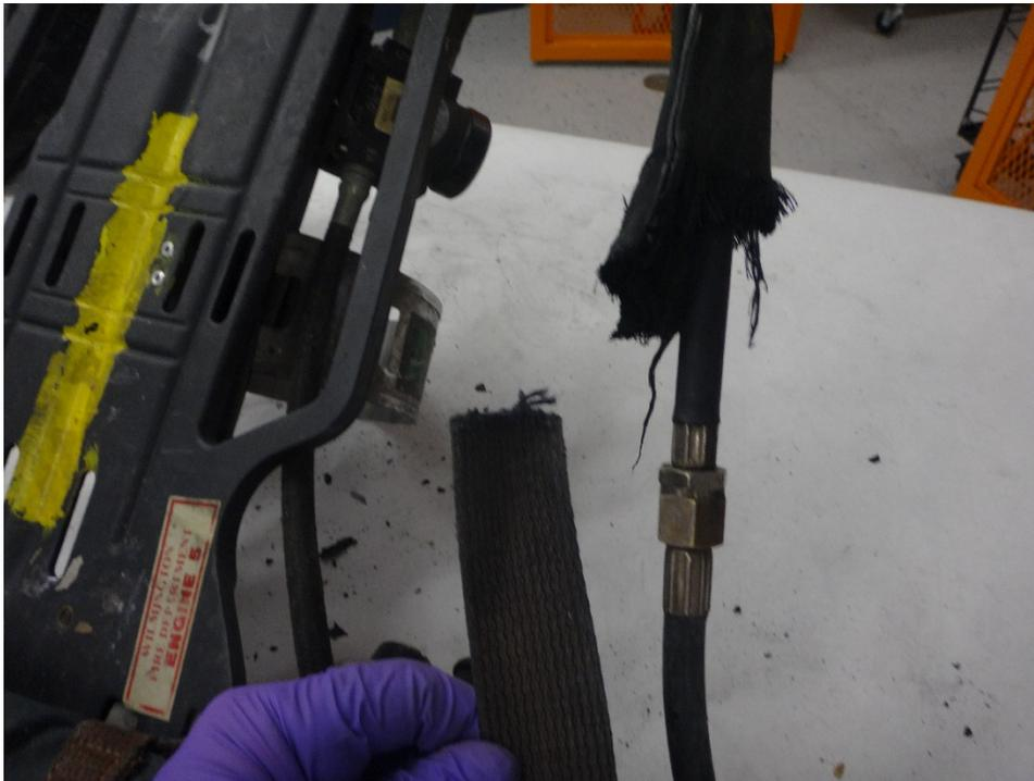
Figure 879: Damage of left shoulder strap
