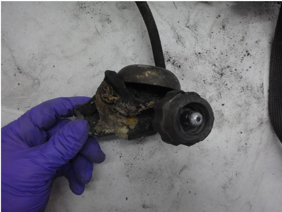
**Figure 72: Cylinder attachment threads and bell assembly**
