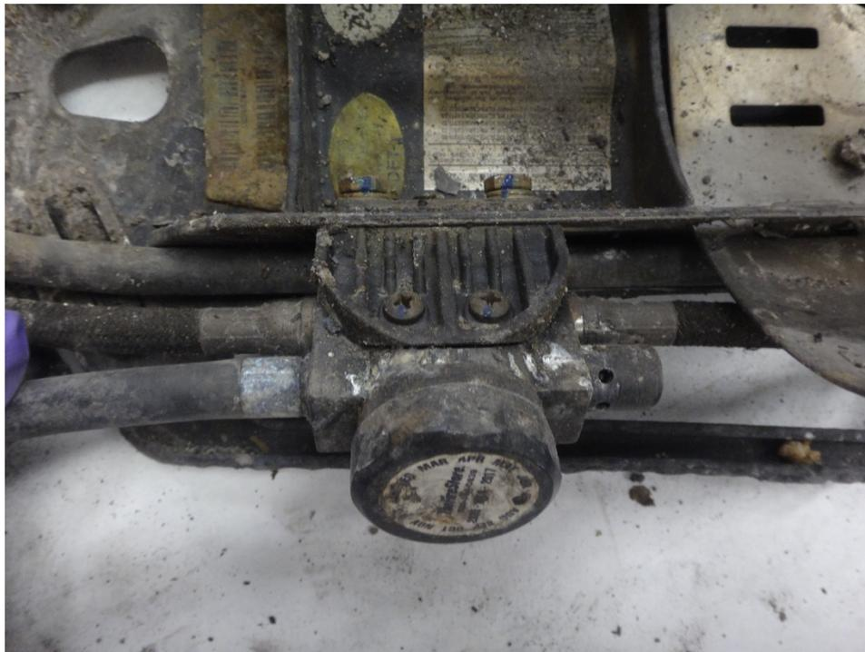
**Figure 65: Pressure reducer assembly inside view**
