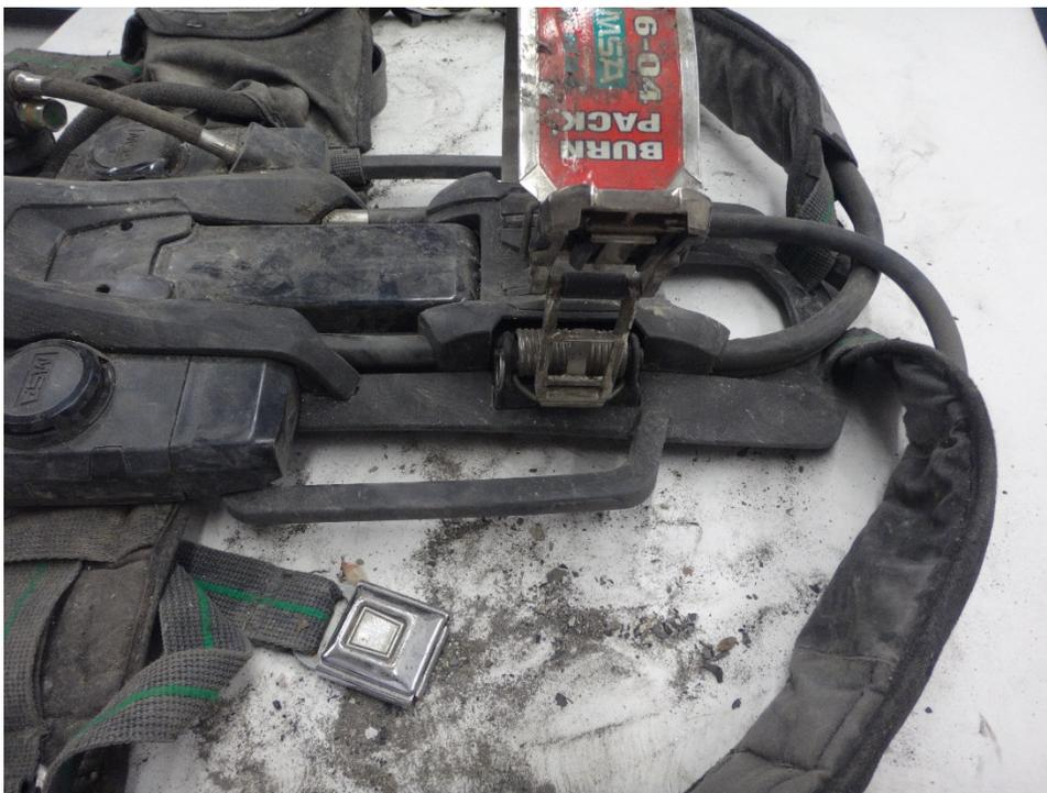
**Figure 8: Low pressure line through shoulder strap**
