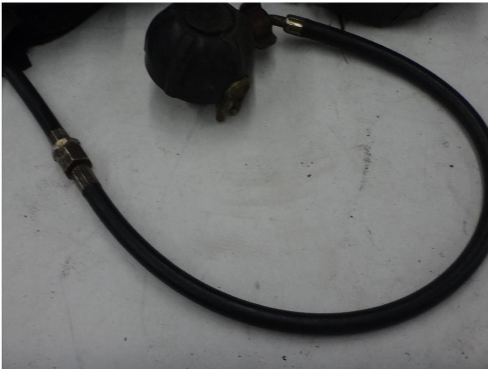
**Figure 37: Low pressure line and MMR**
