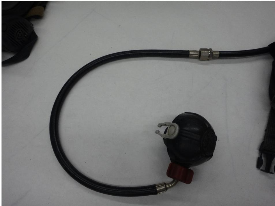
**Figure 12042: Low pressure hose and connecting link**
