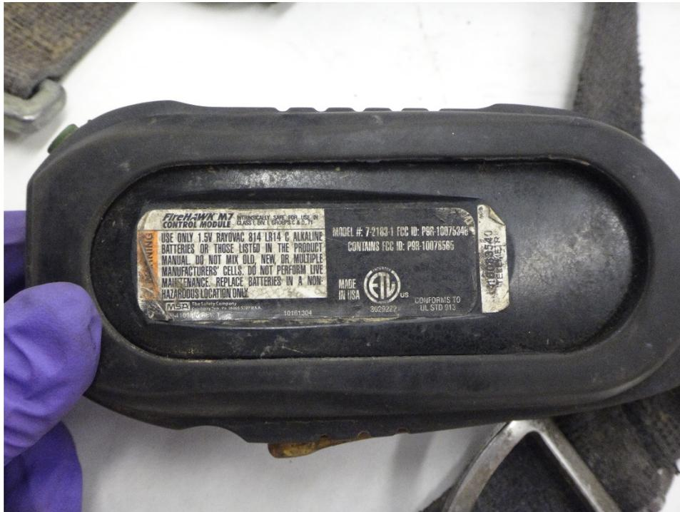
Figure 45: SEI label on the back of the PASS console
