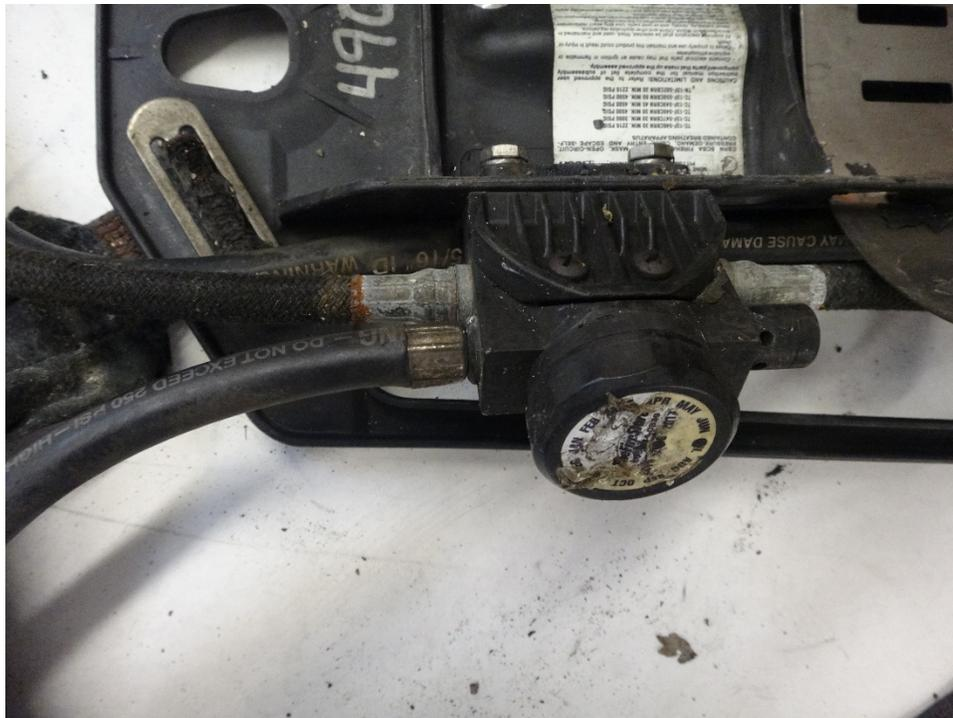
Figure 797: Pressure reducer with "The Fire Store" sticker
