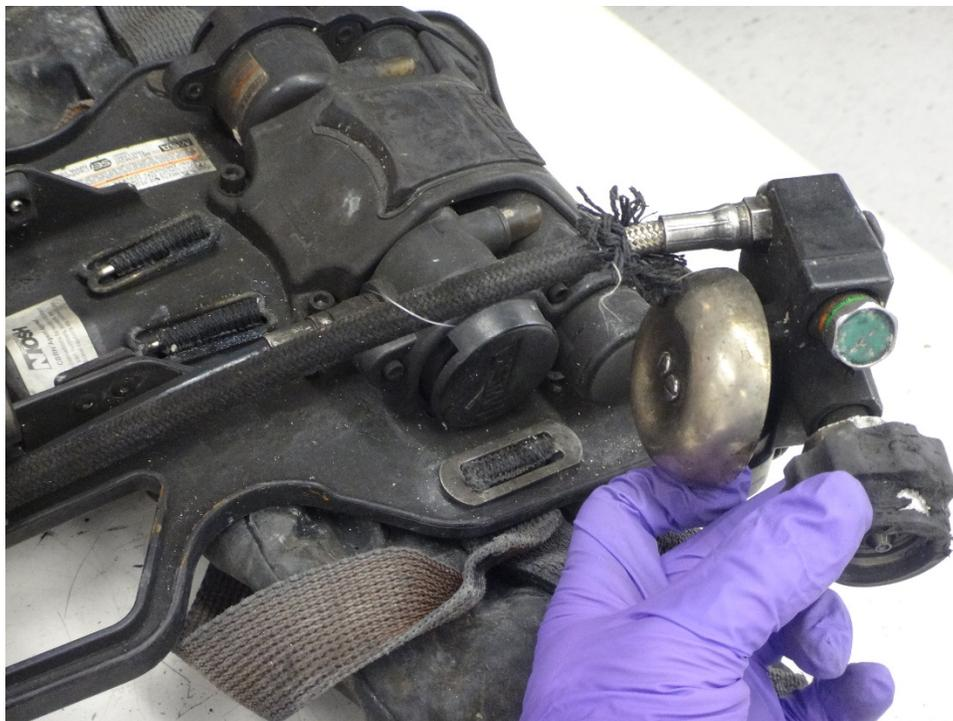
**Figure 10123: High pressure hose, bell assembly, and cylinder attachment**
