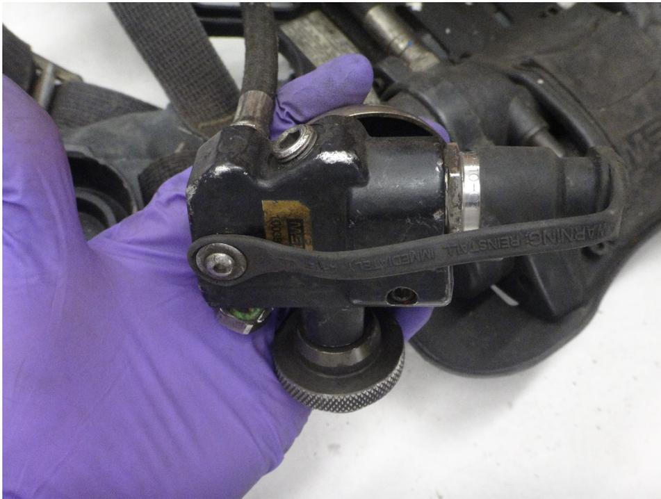
**Figure 42: Dust cap for the RIC UAC system connector**
