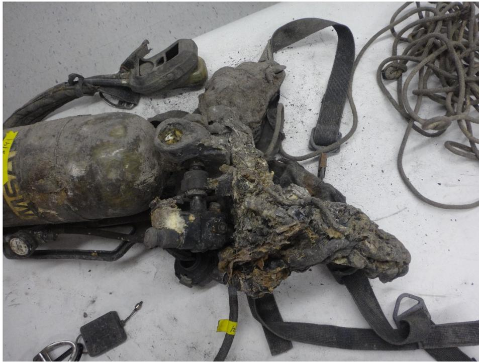
**Figure 637: Debris melted to bottom of unit**
