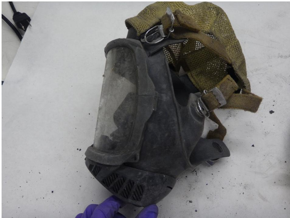
**Figure 4: Side view of facepiece, skirt, and nosecup**
