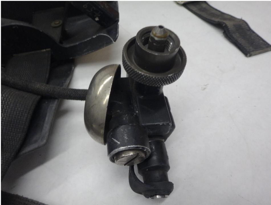
**Figure 1246: Cylinder attachment threads and O-ring**
