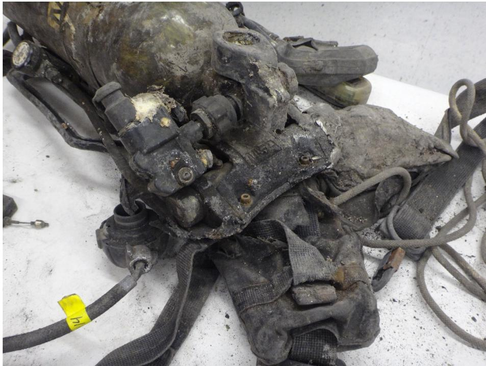
**Figure 659: High pressure line and cylinder attachment attached**
