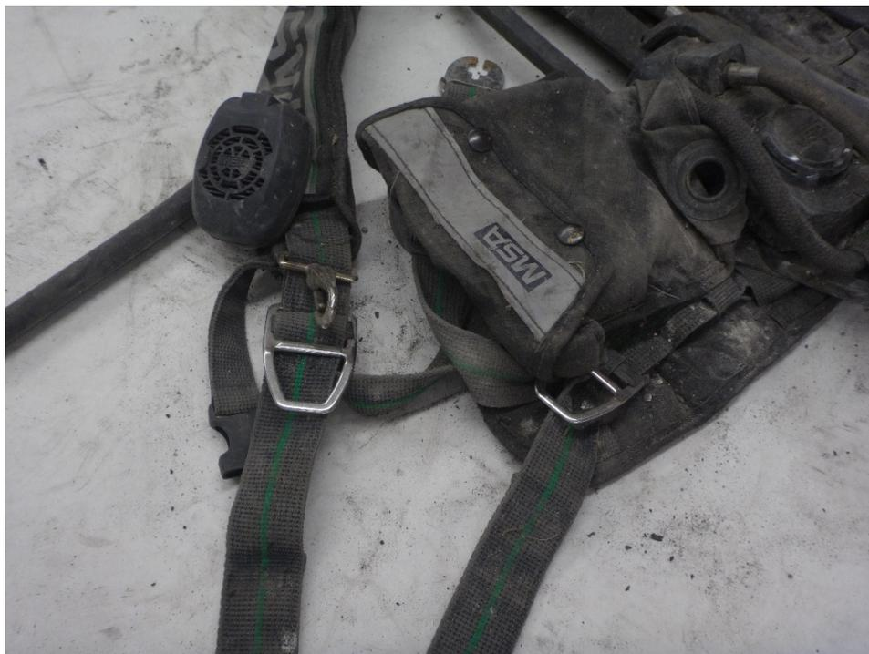
**Figure 22: Communication device and left side straps and buckles**
