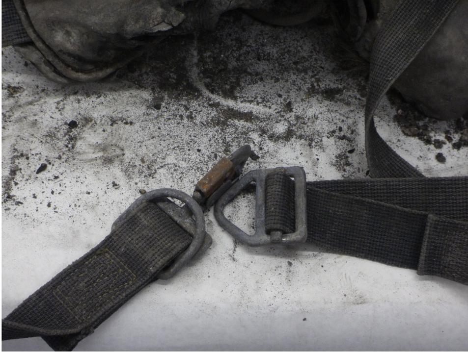
**Figure 8371: Corroded buckles**
