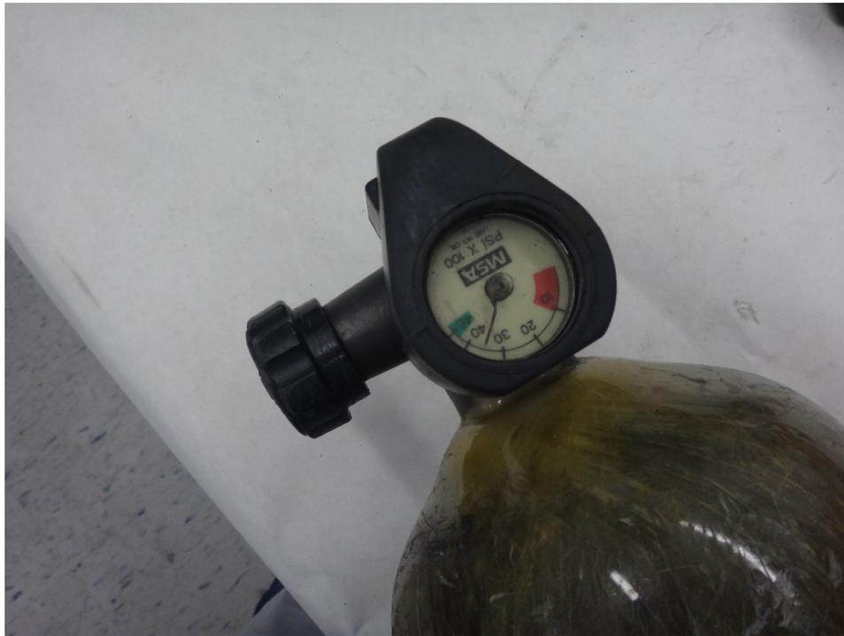
**Figure 1346: Cylinder gauge**
