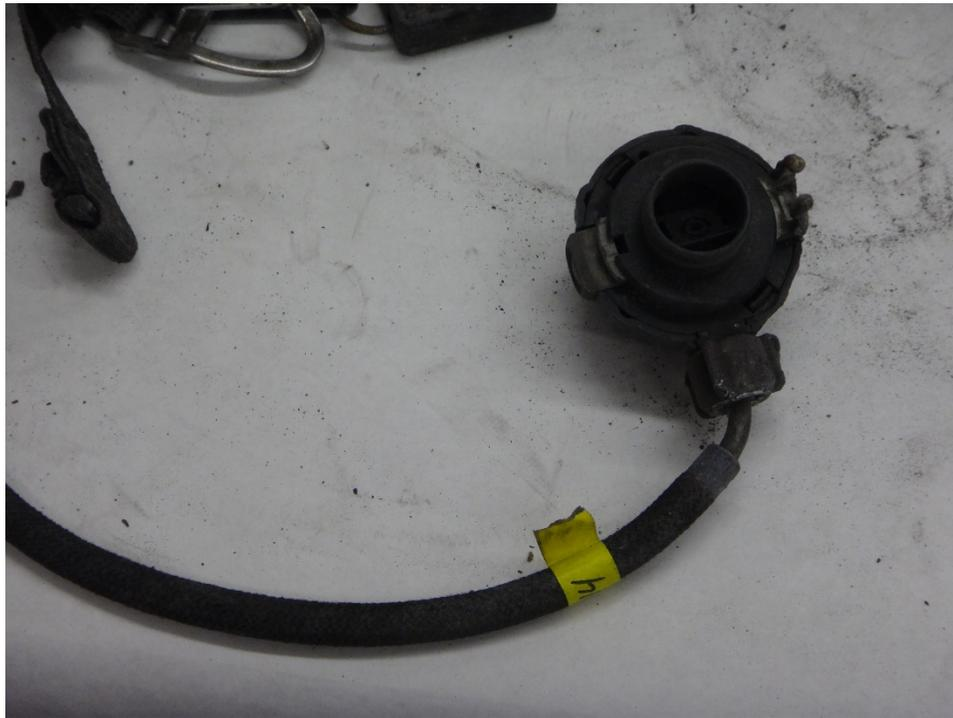
**Figure 613: Sealing flange of MMR and low pressure line**
