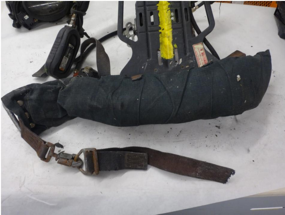
Figure 868: Top view of damage to waist belt
