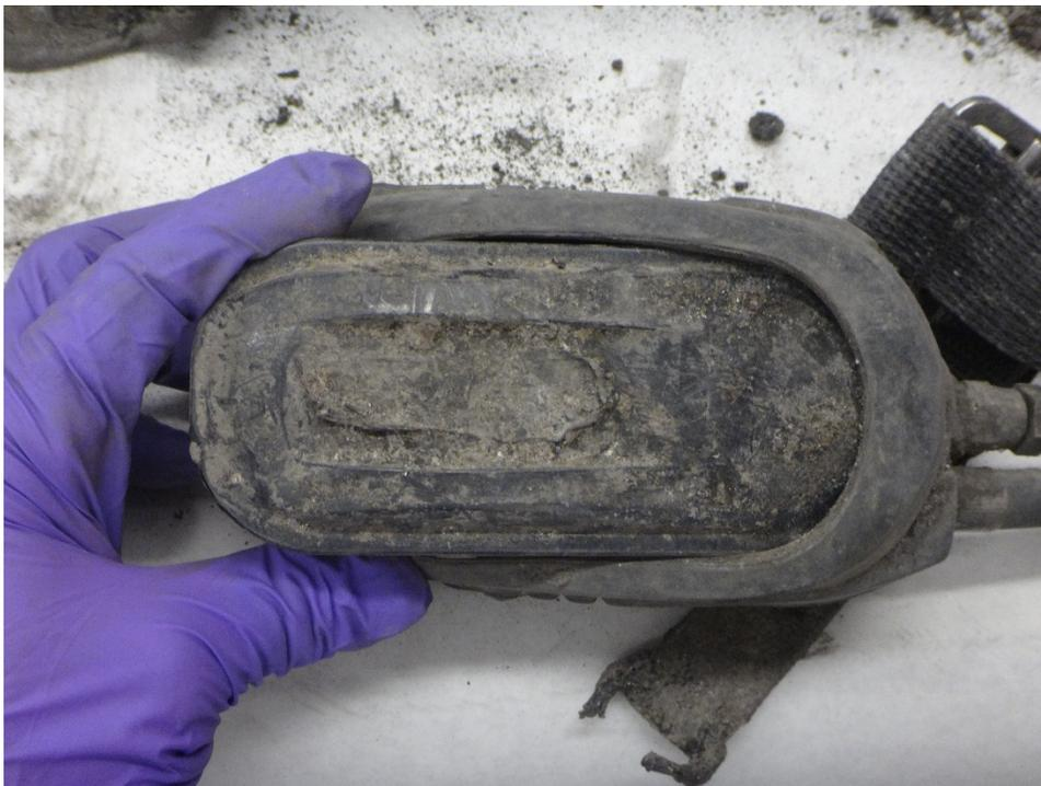
**Figure 74: Back view of PASS console**
