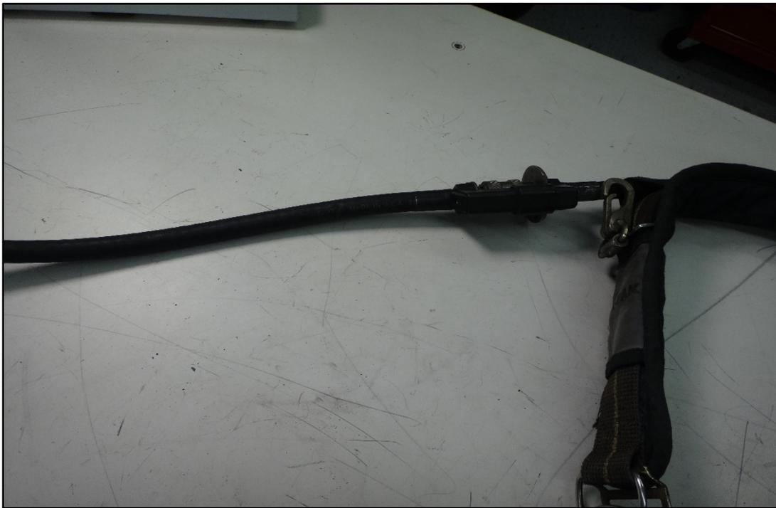
**Figure 28: Low pressure hose and Quick Disconnect**
