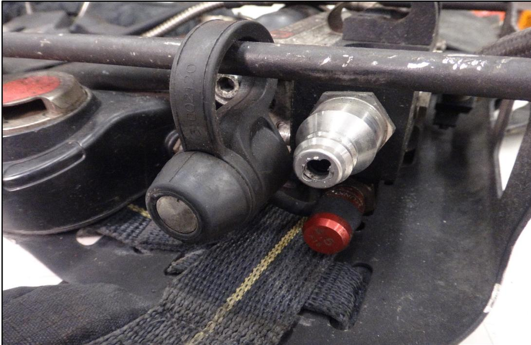
**Figure 33: RIC UAC system connector with cap off**
