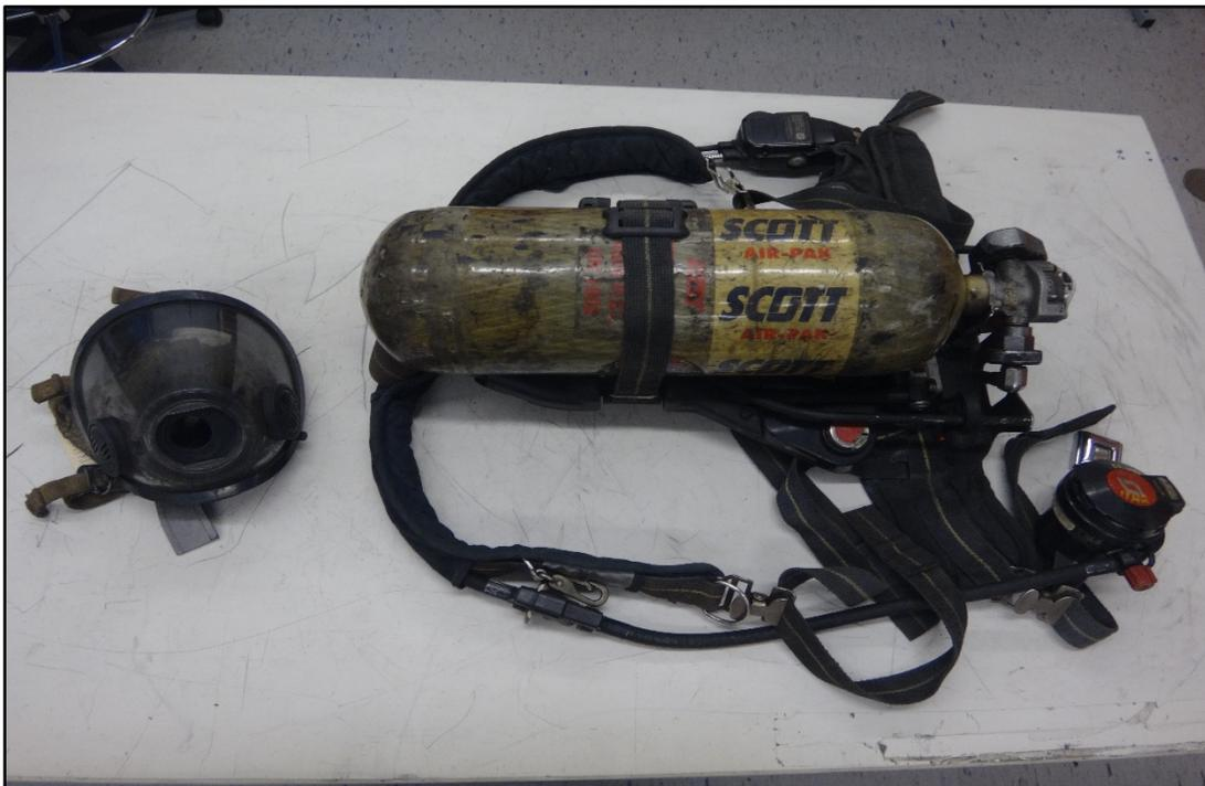
**Figure 20: All components of Unit #3 to be examined**
