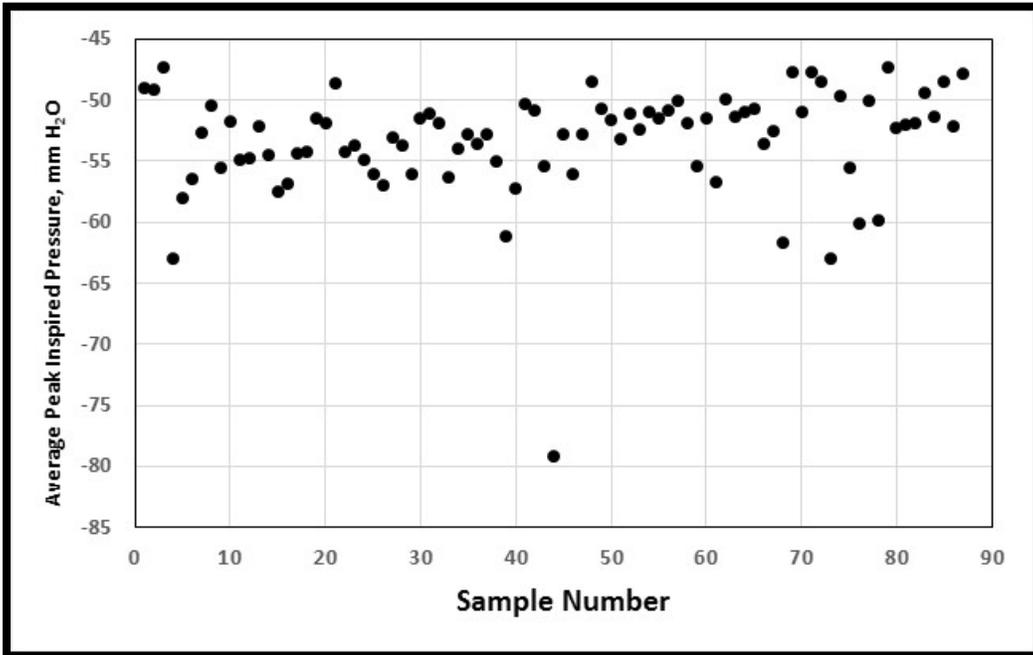
Figure 19. Average Peak Inspired Pressure of Dräger Oxy K SCSR
