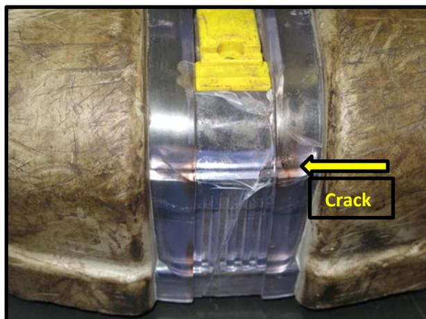
Figure 10. Ocenco M-20 with Cracks in Top Lid
