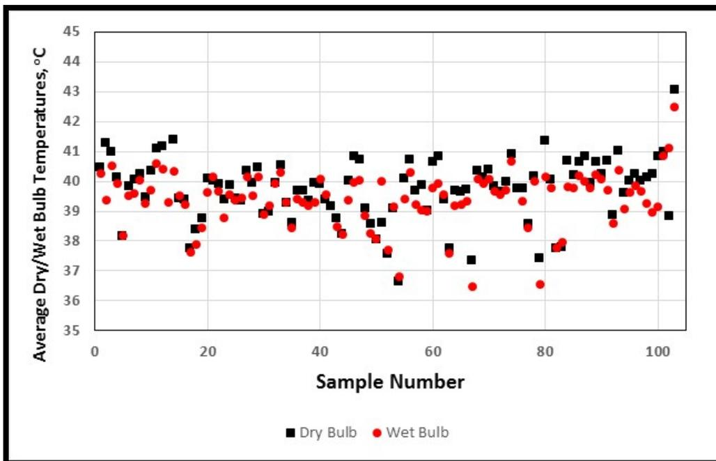
Figure 24. Average Dry/Wet Bulb Temperature of Ocenco EBA 6.5 SCSR
