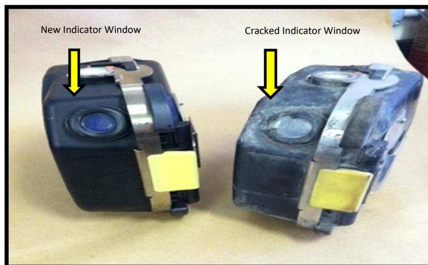
Figure 8. New Moisture Indicator and Cracked Indicator Found After Cleaning at NIOSH
