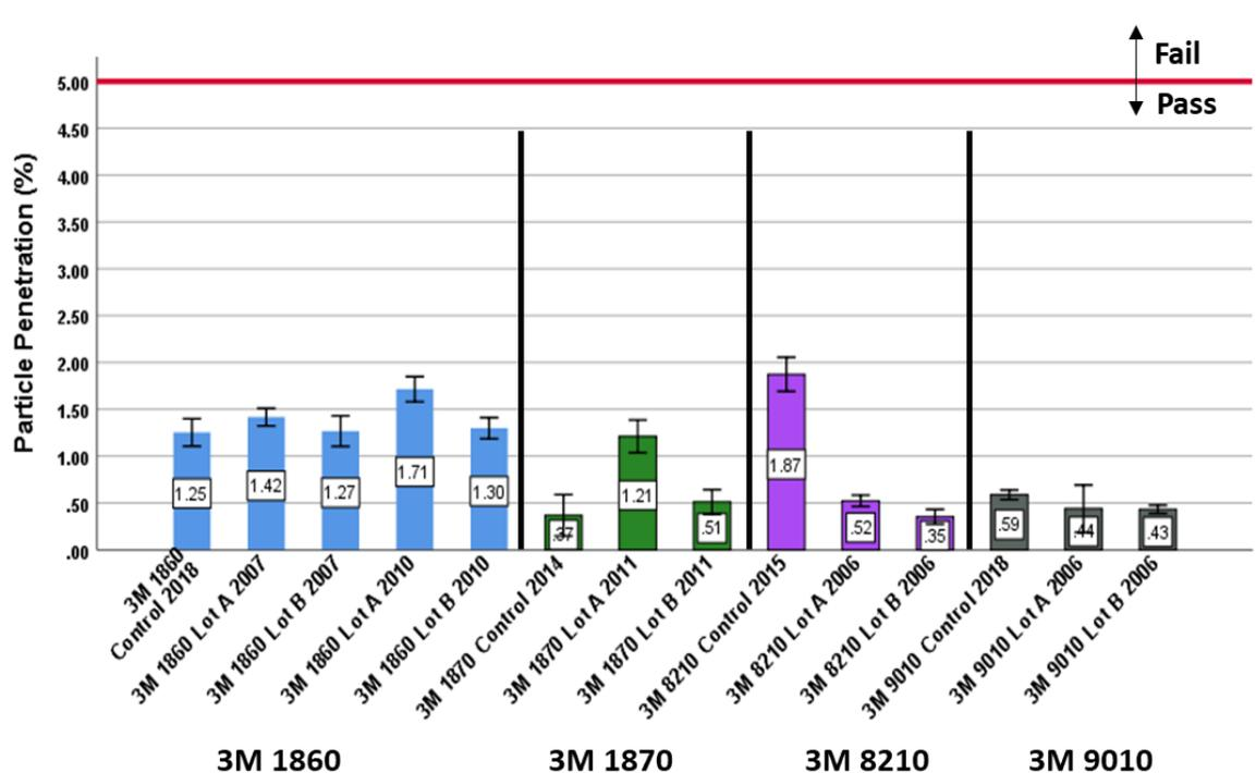
**Figure 9:** Control and stockpiled respirator particle filtration performance data for the 3M 1860, 3M 1870, 3M 8210, and 3M 9010 models. N95 FFRs must have a particle penetration of less than 5.0%. Error bars represent the 99% confidence interval and estimate the population parameters. This confidence interval suggests that 99% of any repeated samples tested and evaluated from this lot will have a mean between the upper and lower bounds.
