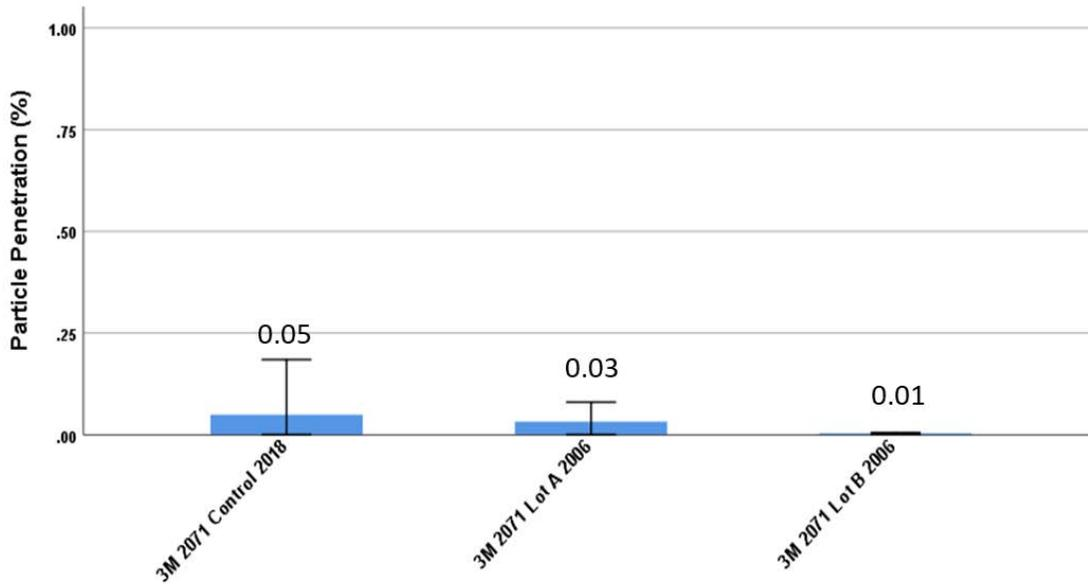
**Figure 10:** Control and stockpiled respirator particle filtration performance data for the 3M 2071 model. P95 FFRs must have a liquid particle penetration of less than 5.0%. Error bars represent the 99% confidence interval and estimate the population parameters. This confidence interval means that 99% of any repeated samples tested and evaluated from this lot will have a mean between the upper and lower bounds.
