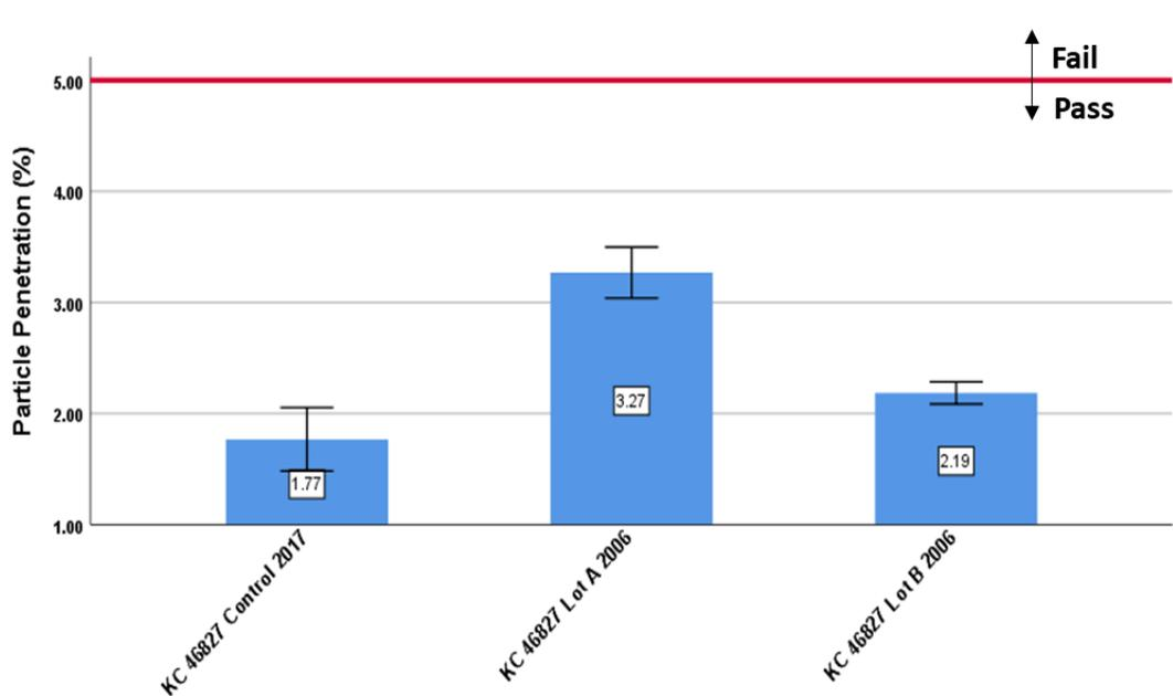
**Figure 11:** Control and stockpiled respirator particle filtration performance data for the KC 46827 model. N95 FFRs must have a particle penetration of less than 5.0%. Error bars represent the 99% confidence interval and estimate the population parameters. This confidence interval suggests that 99% of any repeated samples tested and evaluated from this lot will have a mean between the upper and lower bounds.
