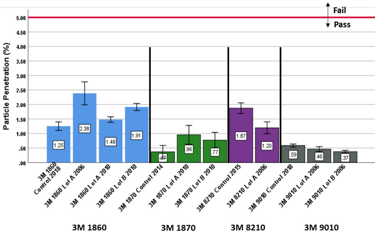
**Figure 10:** Control and stockpiled respirator particle filtration performance data for the 3M 1860, 3M 1870, 3M 8210, and 3M 9010 models. N95 FFRs must have a particle penetration of less than 5.0%. Error bars represent the 99% confidence interval and estimate the population parameters. This confidence interval suggests that 99% of any repeated samples tested and evaluated from this lot will have a mean between the upper and lower bounds.
