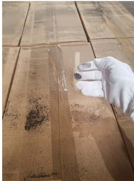
**Figure 2:** Most amount of dust observed on product cases from Facility Four.
