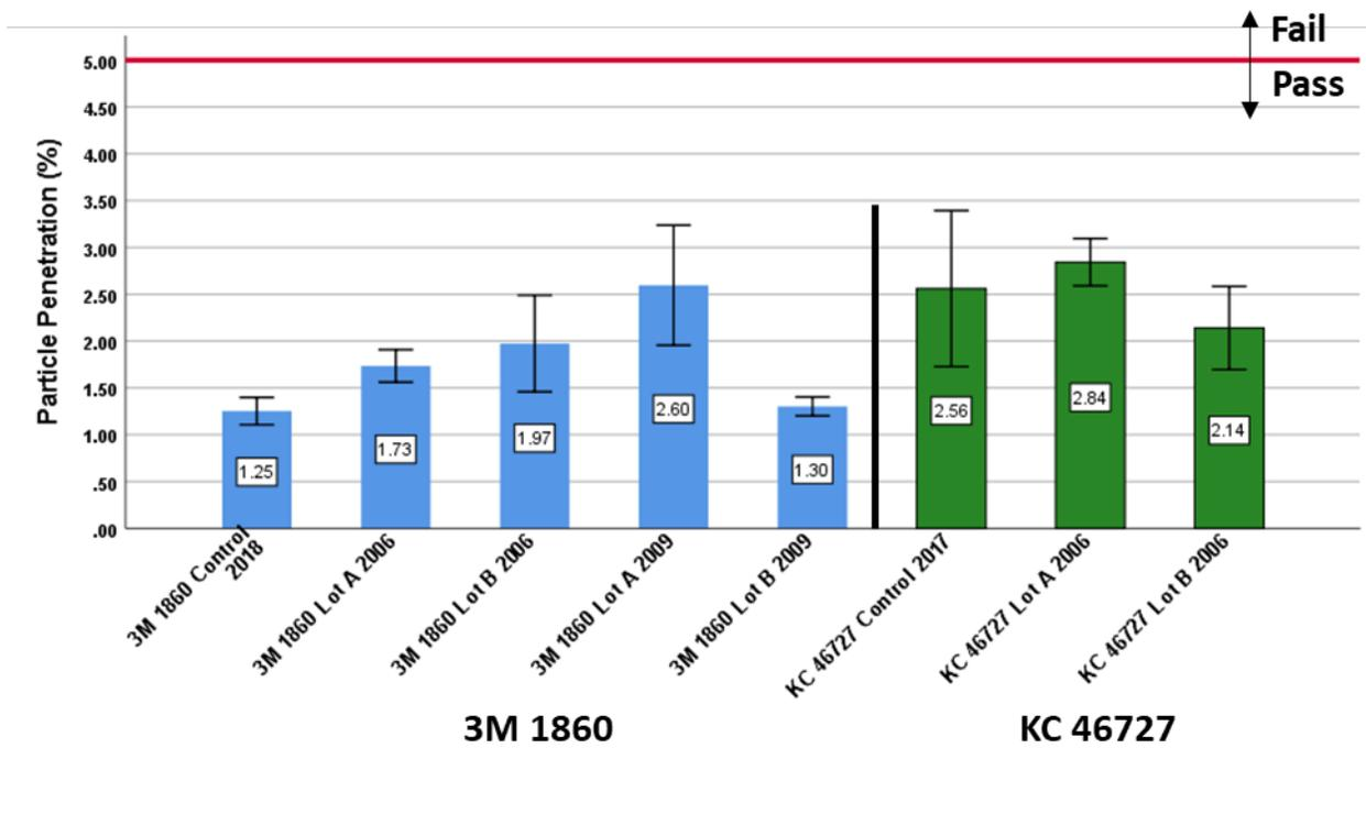
**Figure 8:** Control and stockpiled respirator particle filtration performance data. N95 FFRs must have a particle penetration of less than 5.0%. Error bars represent the 99% confidence interval and estimate the population parameters. This confidence interval suggests that 99% of any repeated samples tested and evaluated from this lot will have a mean between the upper and lower bounds.
