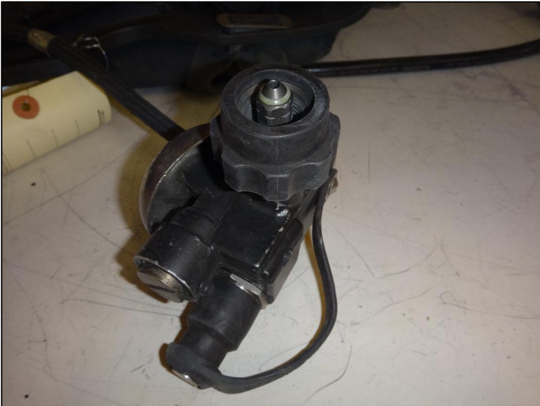
**Figure 9: Cylinder attachment overview and relief valve with bell assembly**
