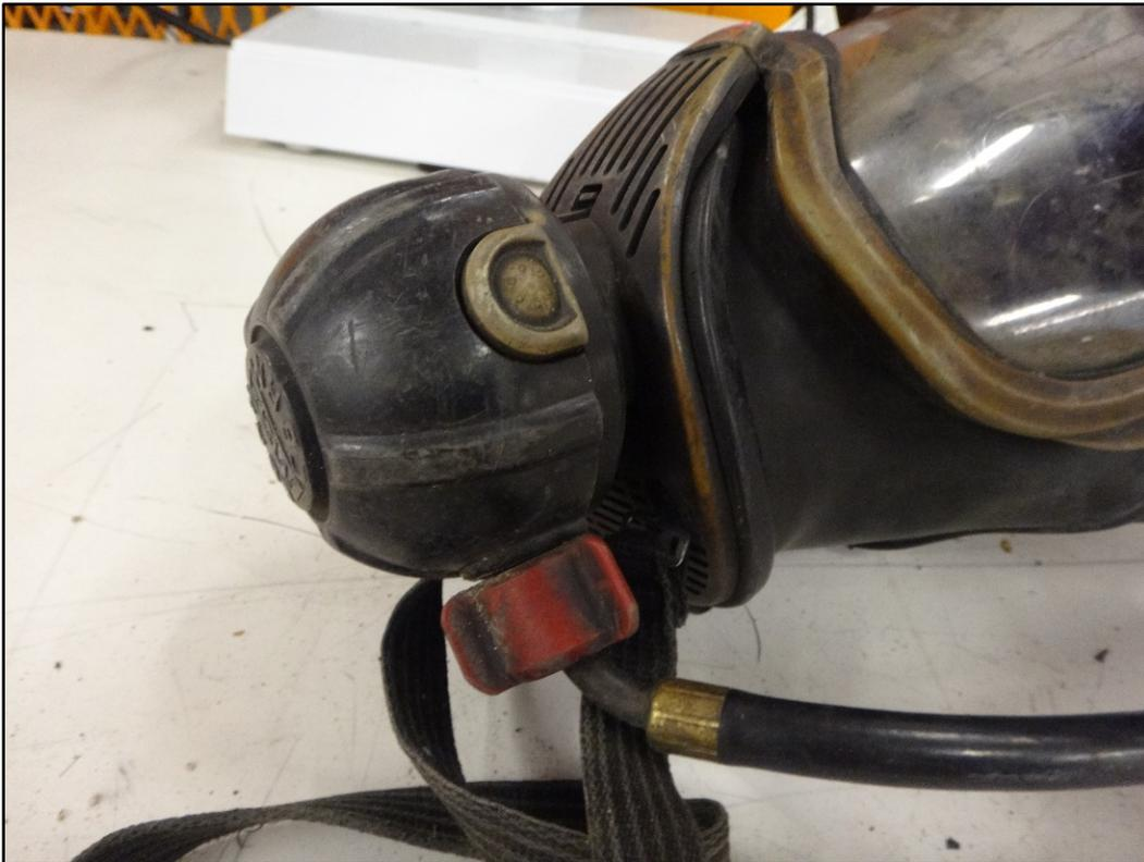
**Figure 5: Mask mounted regulator (MMR) attached to facepiece**
