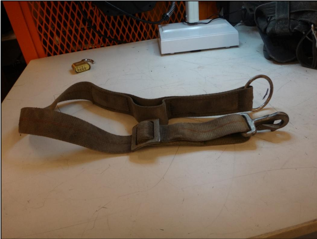
**Figure 29: Fall restraint belt**
