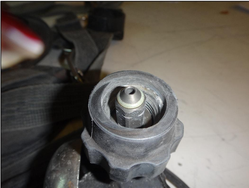
**Figure 18: Cylinder attachment overview with O-ring present**
