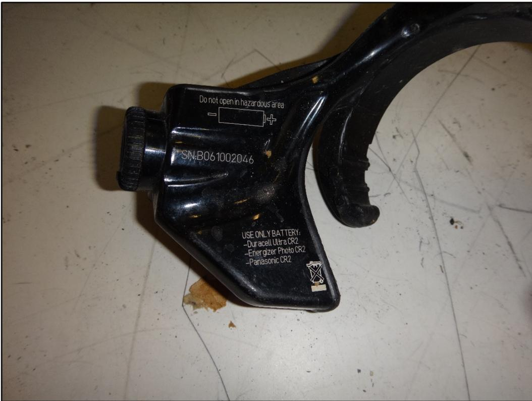
**Figure 10: HUD Removed from facepiece to display markings (left side)**
