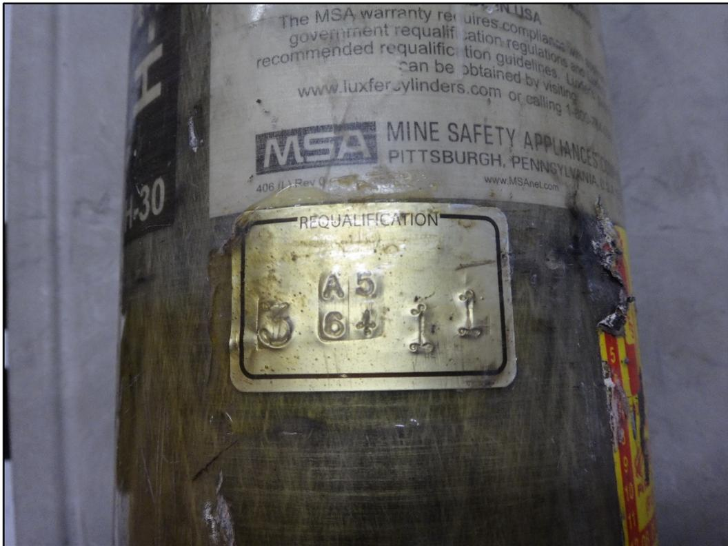
Figure 32: Hydrostatic test date
