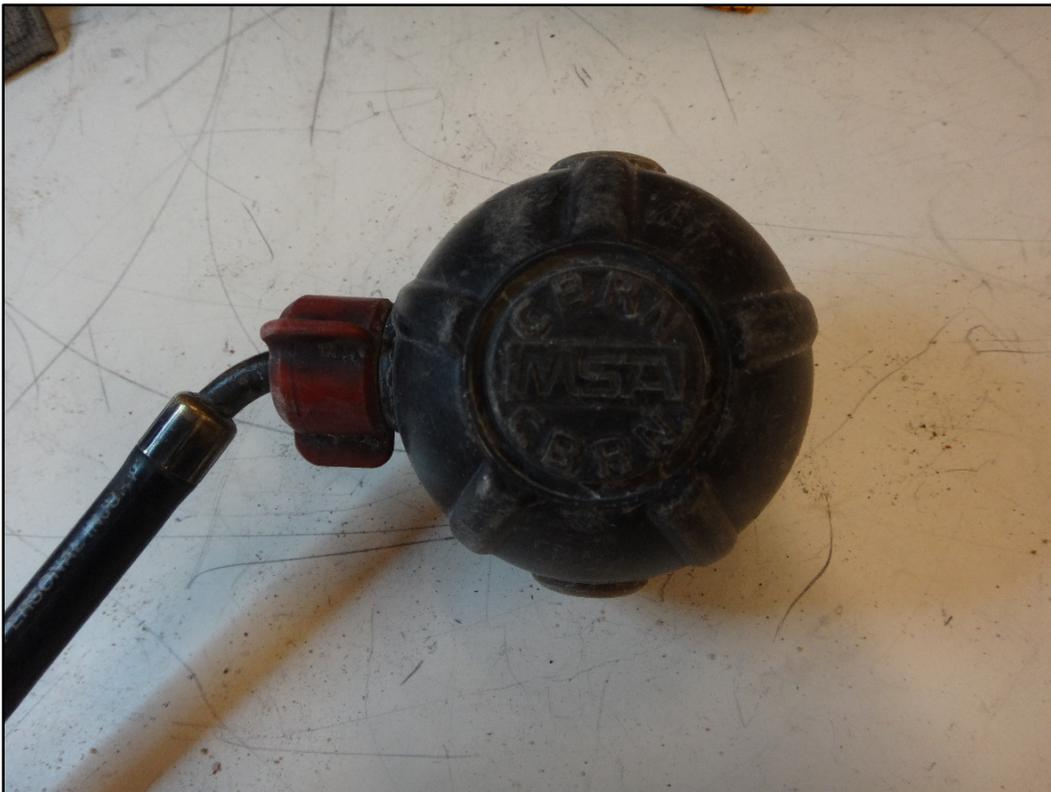
**Figure 14: Mask mounted regulator (MMR)**
