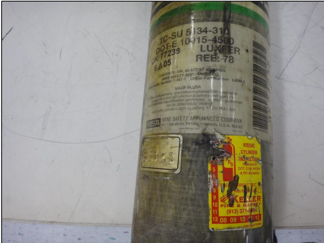
Figure 31: Identifying markings and cylinder information
