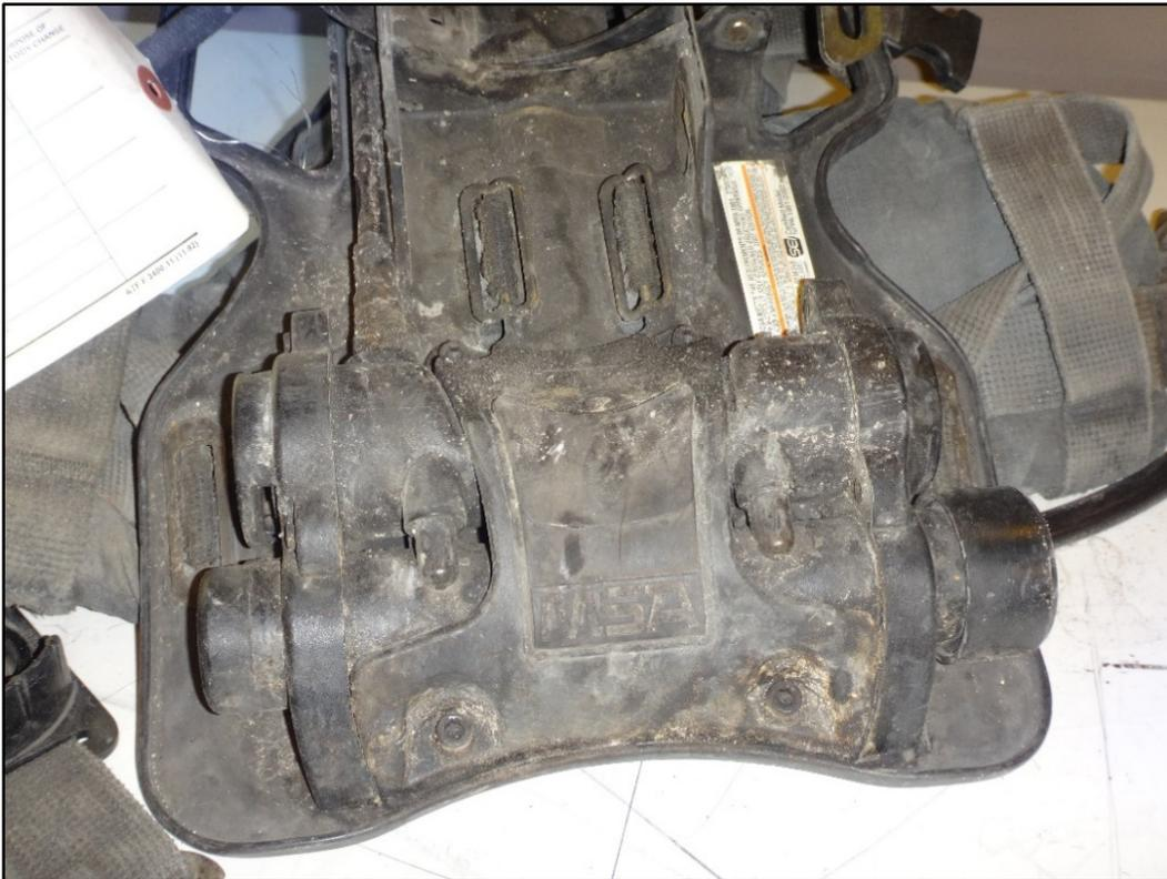
**Figure 17: PASS control module**
