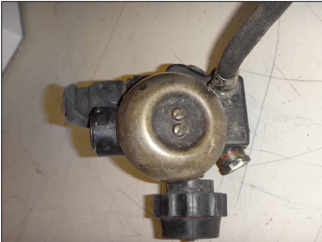
**Figure 10: Cylinder attachment overview and relief valve with bell assembly**
