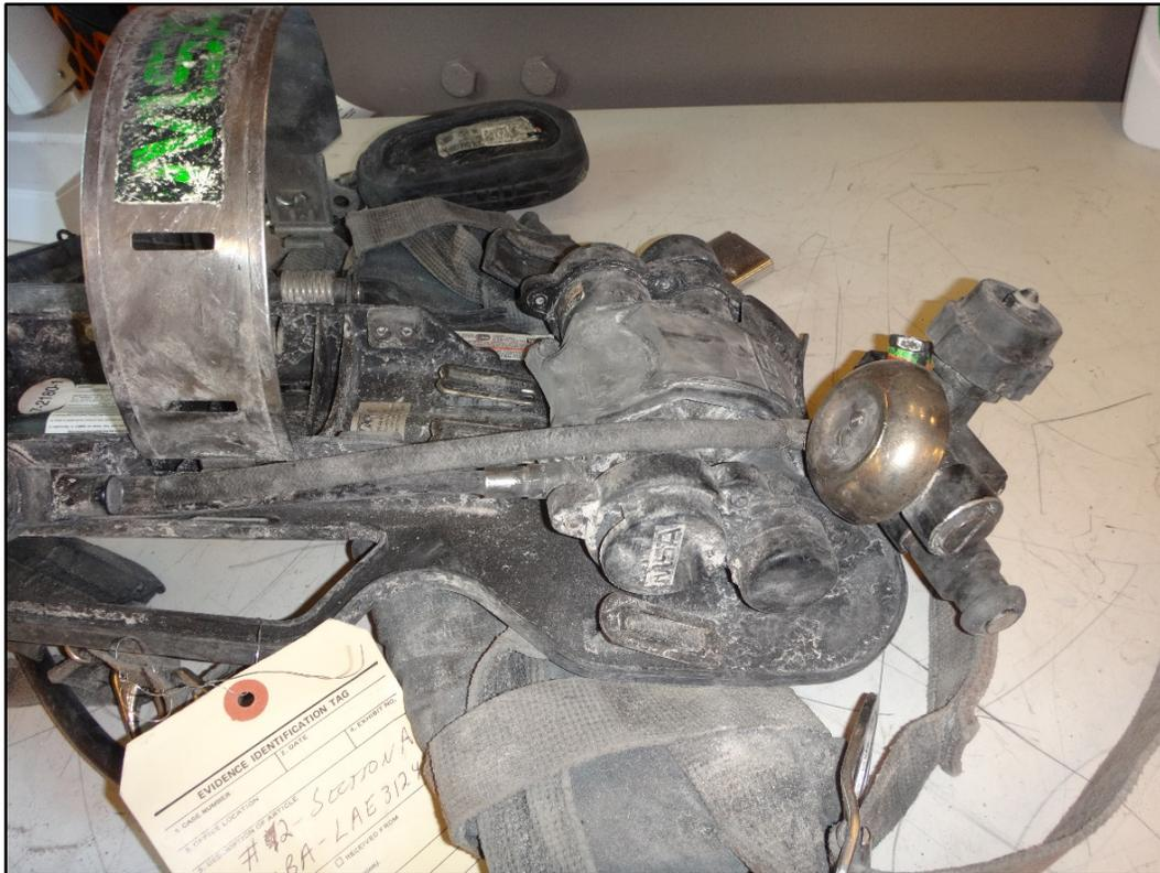
**Figure 19: High-pressure hose and cylinder attachment**
