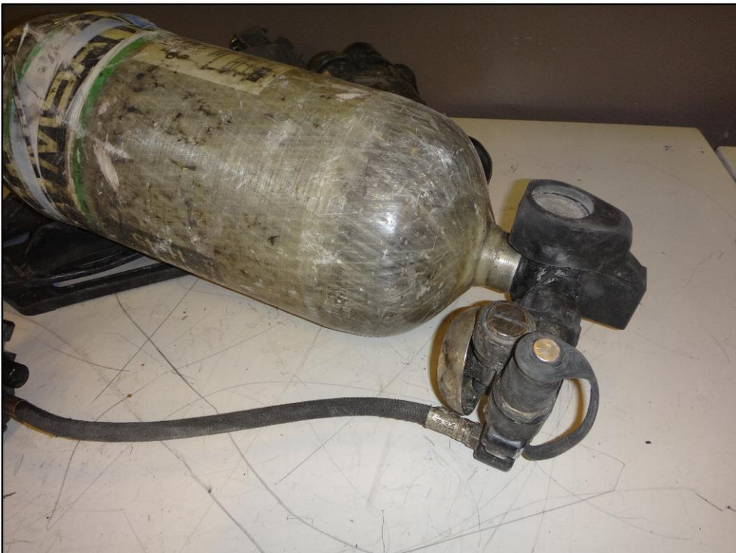
**Figure 18: High-pressure hose and cylinder attachment**
