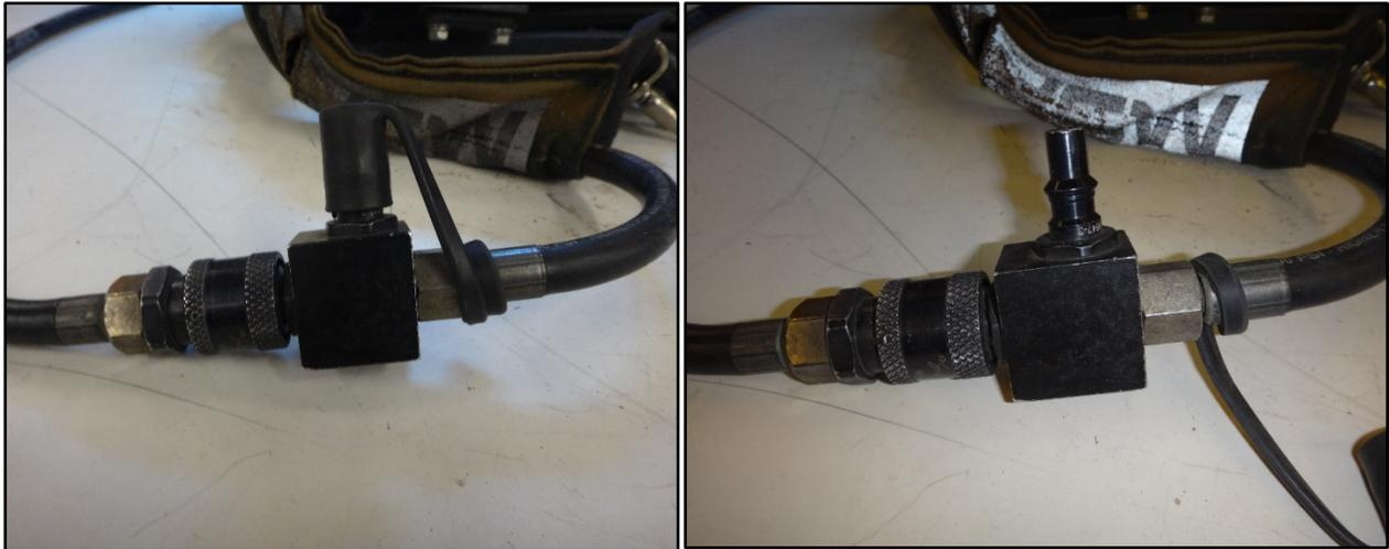
**Figure 14: Low-pressure connection with and without cover**
