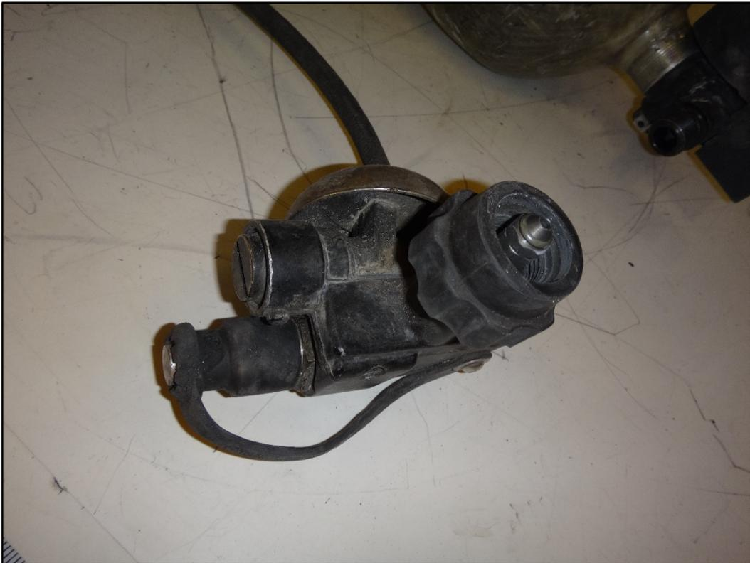
**Figure 19: Cylinder attachment overview and relief valve with bell assembly**
