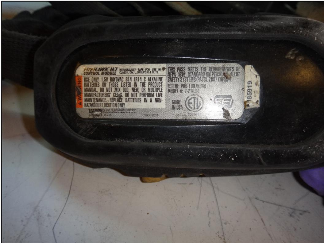
Figure 21: Back of PASS console, SEI label
