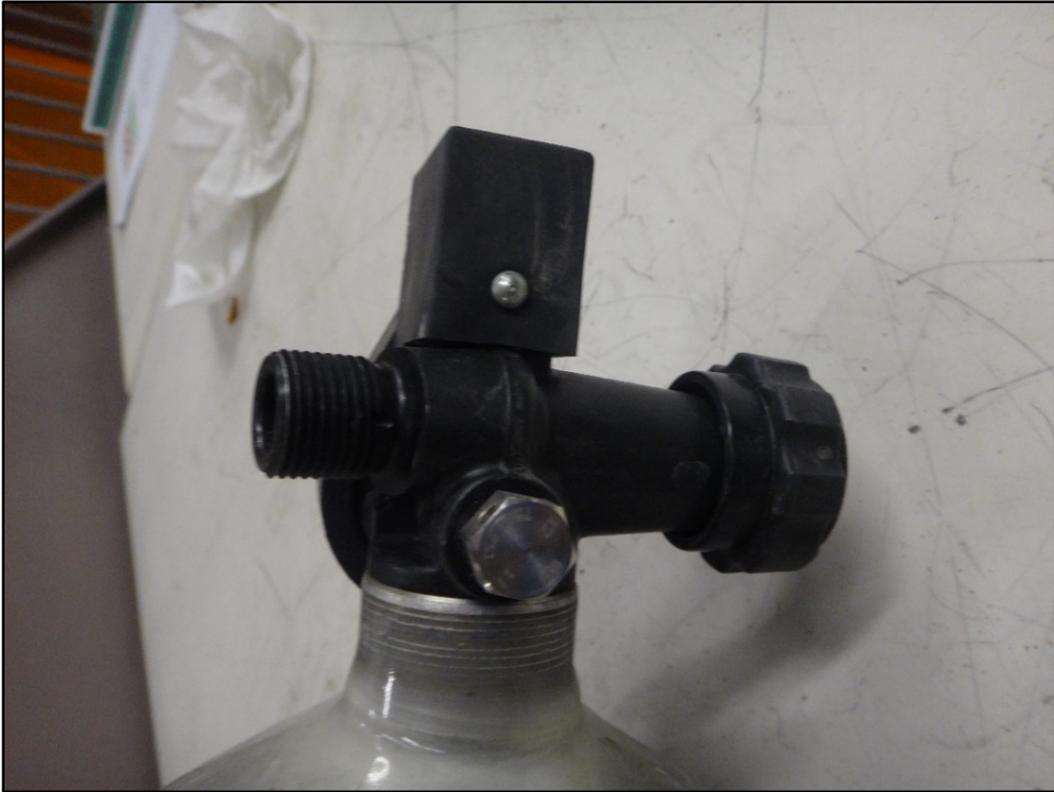
**Figure 21: Threads on cylinder attachment**
