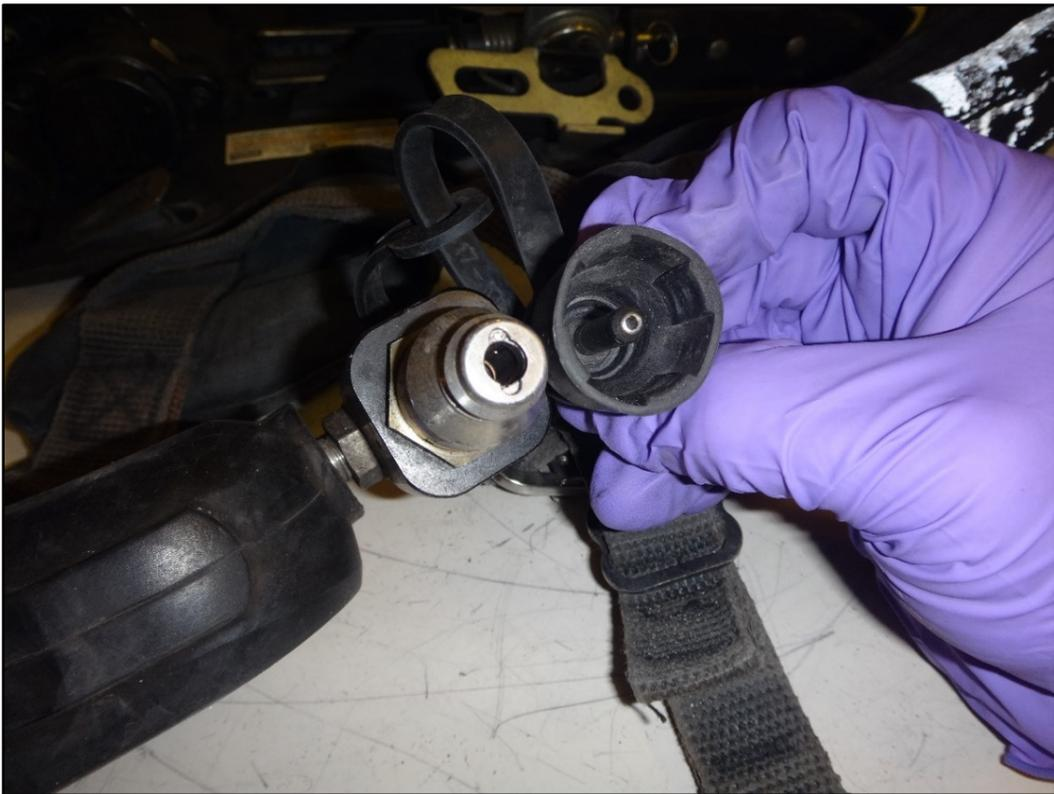
Figure 14: Additional Quick-Fill port on console
