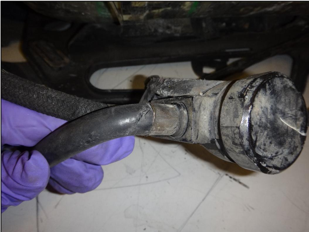
**Figure 16: Low-pressure line at reducer connection**
