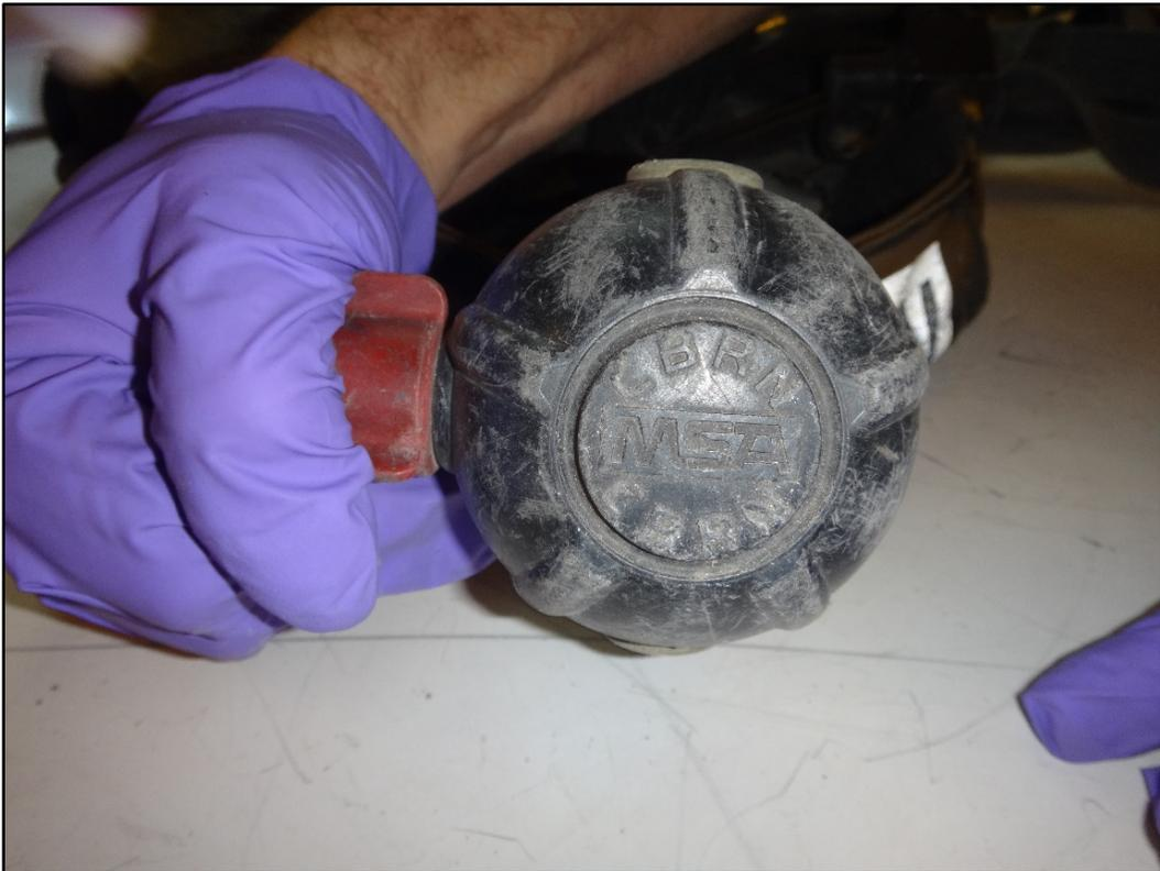
**Figure 9: Mask mounted regulator (MMR)**
