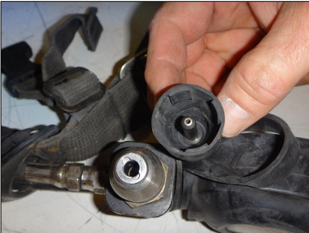
**Figure 16: Additional Quick-Fill port on console**
