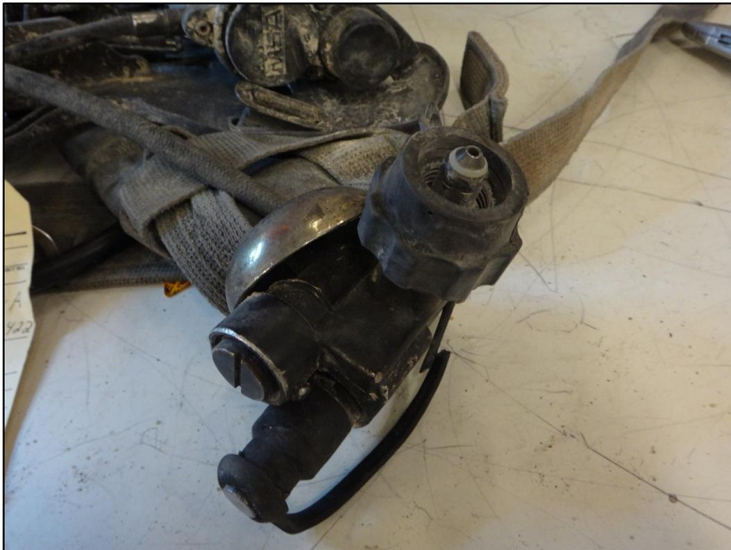
**Figure 20: Cylinder attachment overview and relief valve with bell assembly**
