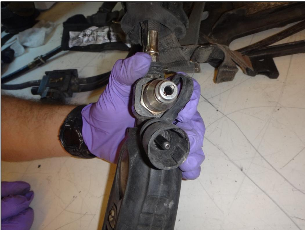
**Figure 24: Overview of Quick-Fill port on console**
