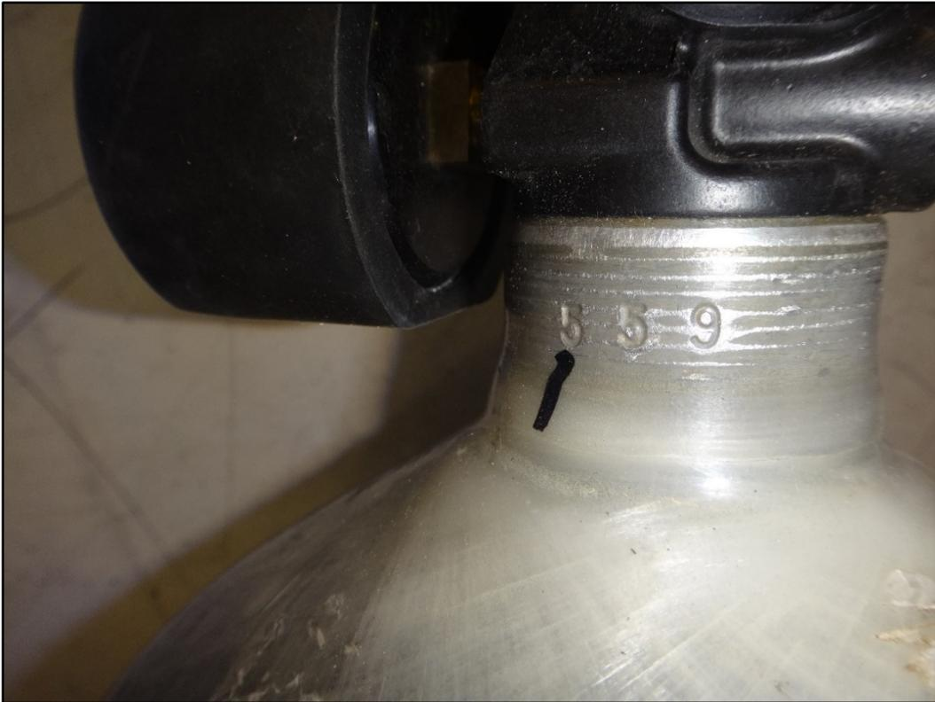
**Figure 22: Cylinder identifier**
