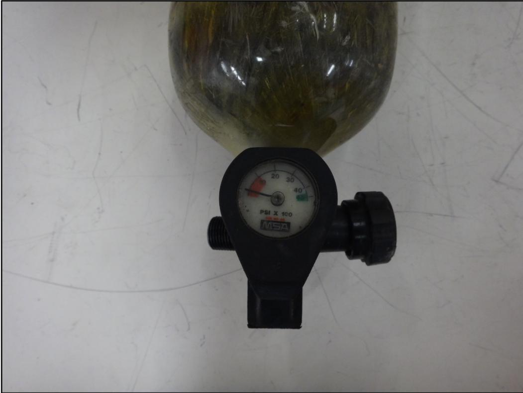
**Figure 33: Cylinder gauge**
