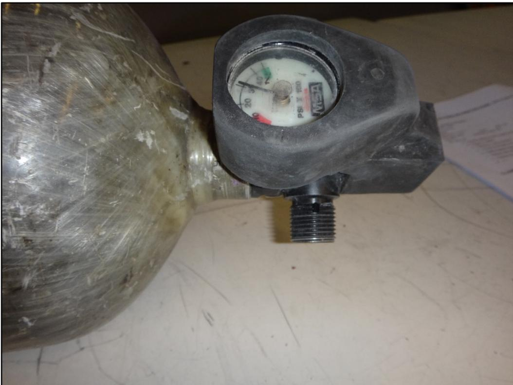
**Figure 37: Cylinder gauge is readable and threads clean**
