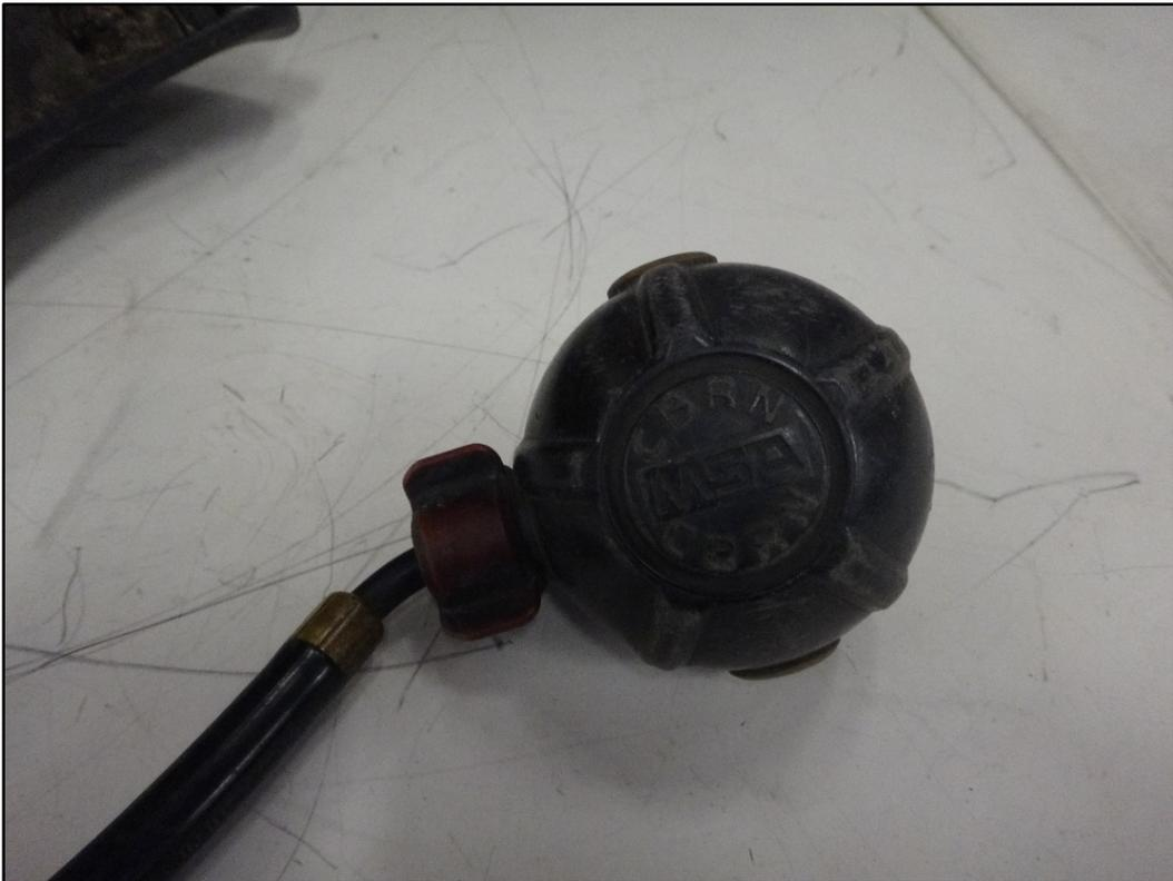
**Figure 5: Mask mounted regulator (MMR)**
