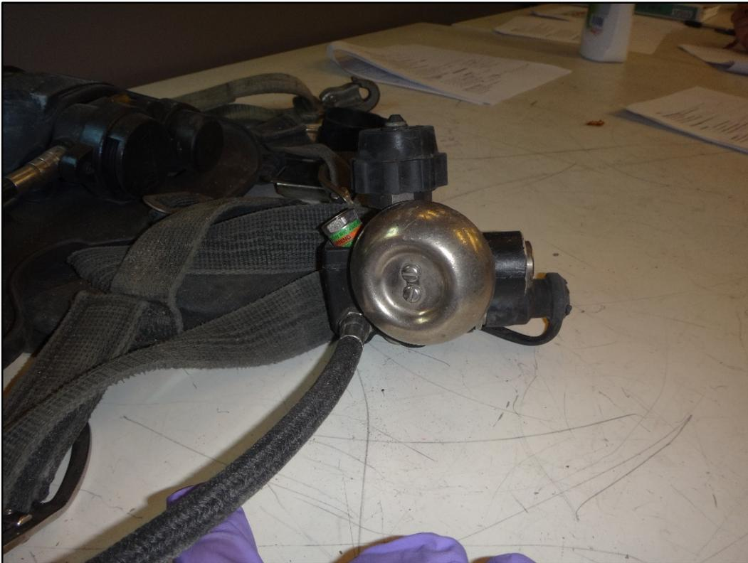
**Figure 17: High-pressure hose and cylinder attachment**
