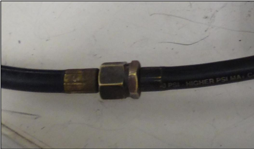
**Figure 15: Low-pressure connection**
