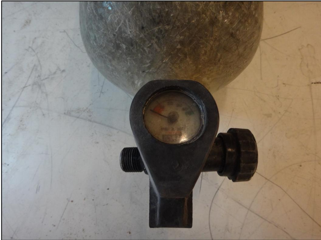
**Figure 36: Cylinder gauge is readable**
