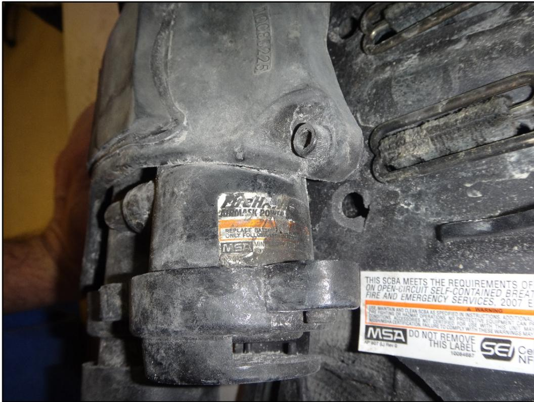
Figure 25: Label on side of PASS control module
