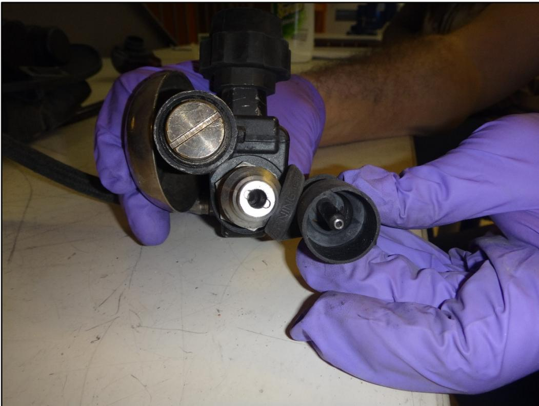
**Figure 10: Quick-Fill port on cylinder attachment overview**
