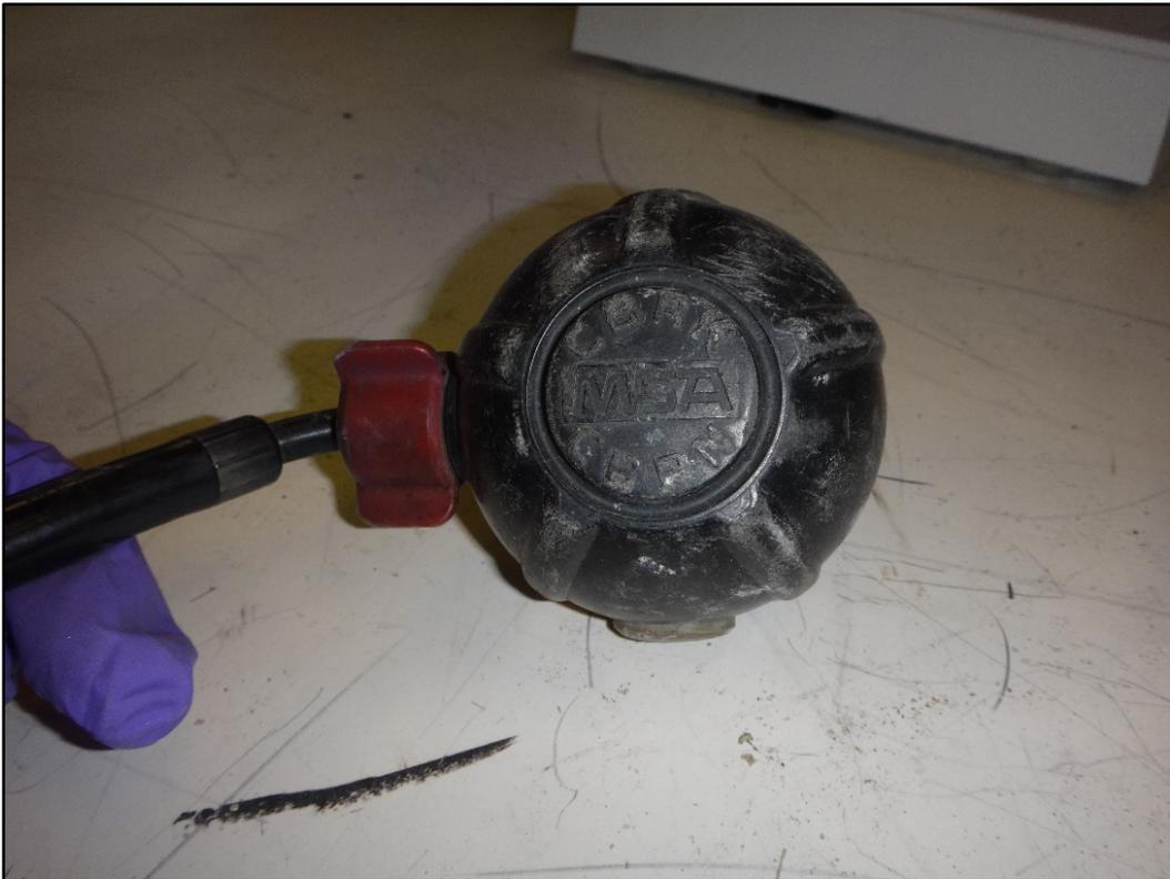
**Figure 5: Mask mounted regulator (MMR)**
