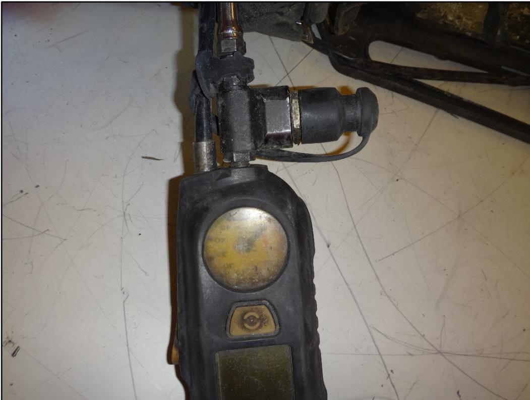
**Figure 23: Additional Quick-Fill port on console**
