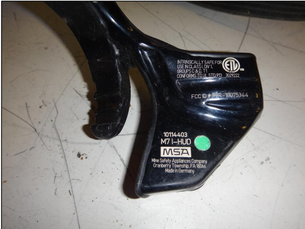
Figure 11: HUD removed from facepiece to display markings (right side)
