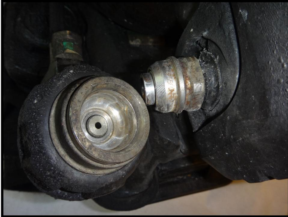
**Figure 17: Cylinder attachment and Quick Connect adapter**
