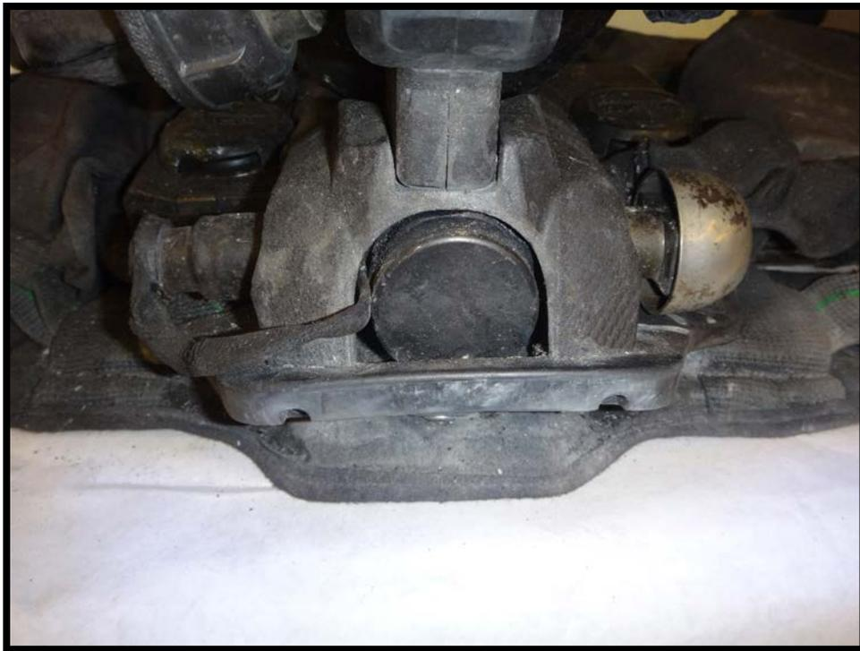
**Figure 10: Pressure reducer, RIC UAC with primary low pressure warning device (bell)**
