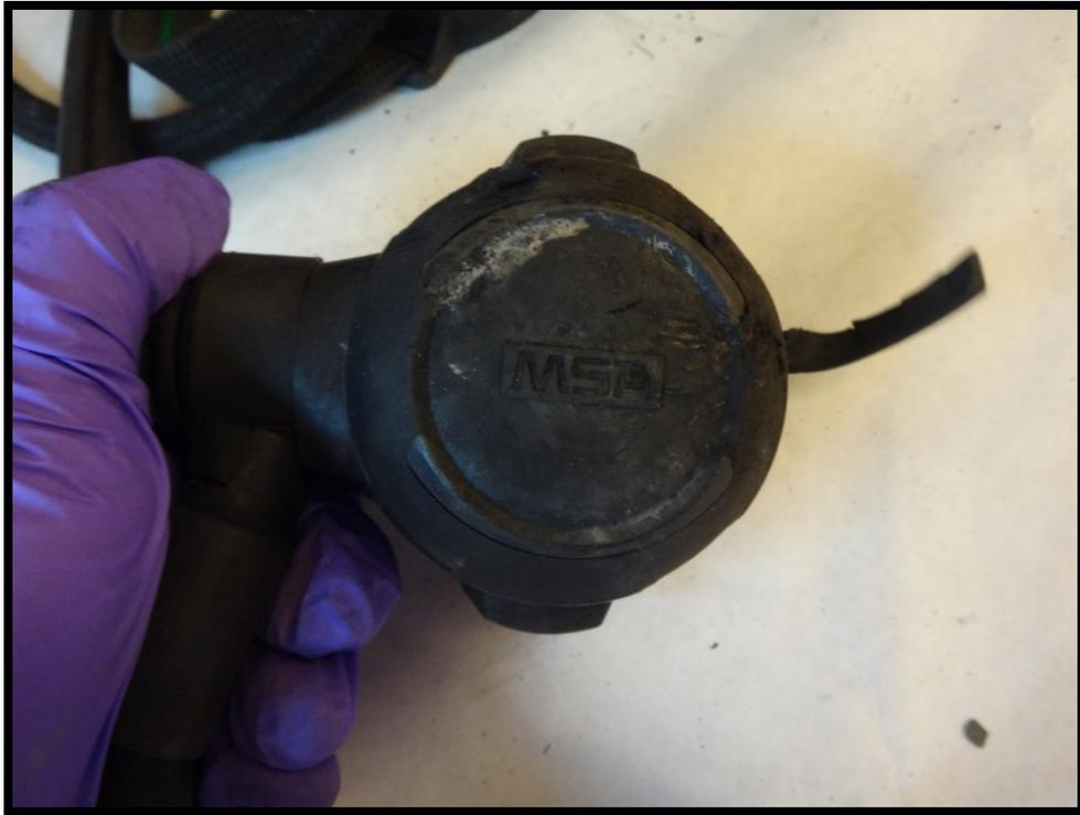
**Figure 6: Mask mounted regulator with signs of heat damage**
