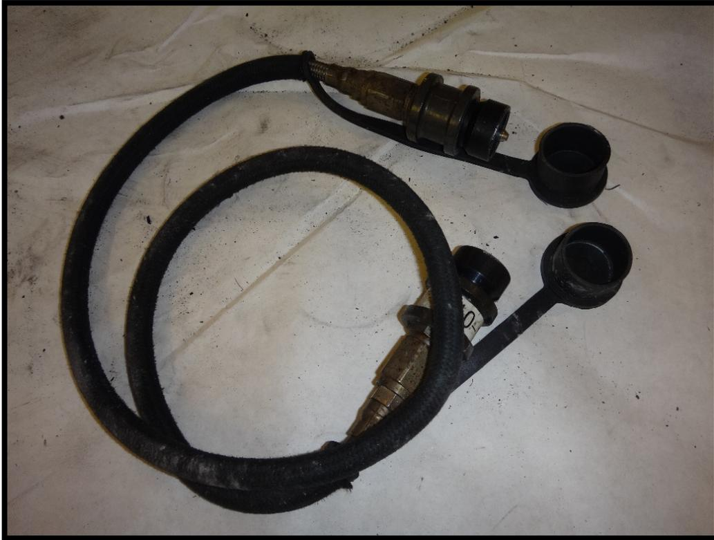
Figure 24: Quick-Fill hose with covers off
