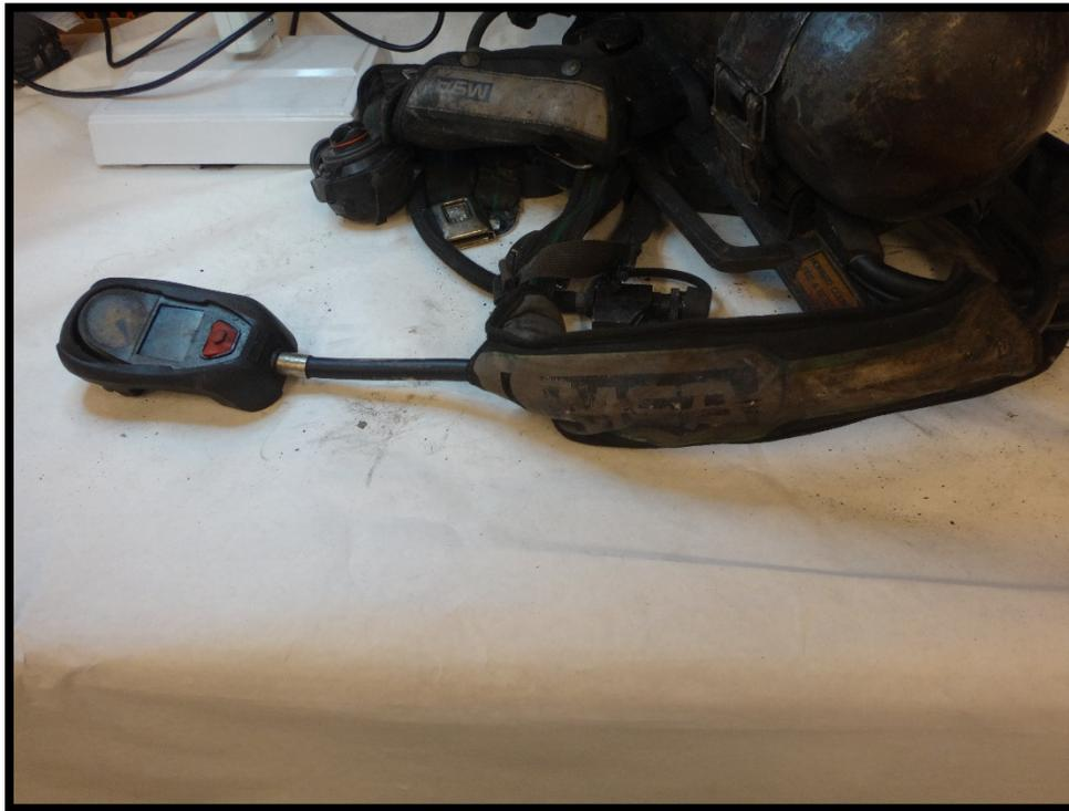
**Figure 12: PASS control module and medium pressure line**
