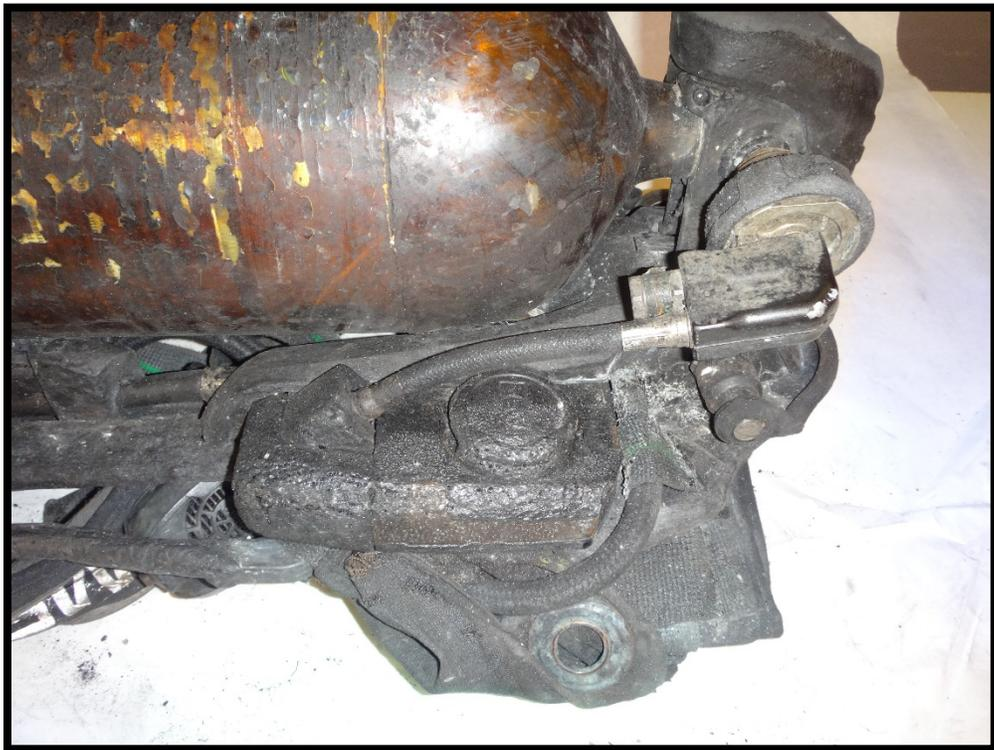
**Figure 15: High pressure hose and cylinder attachment**
