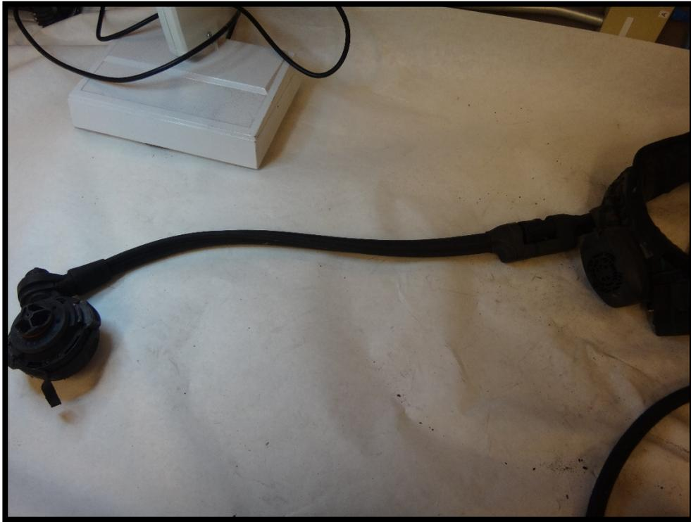
**Figure 8: Mask mounted regulator and low pressure line connected to SCBA**
