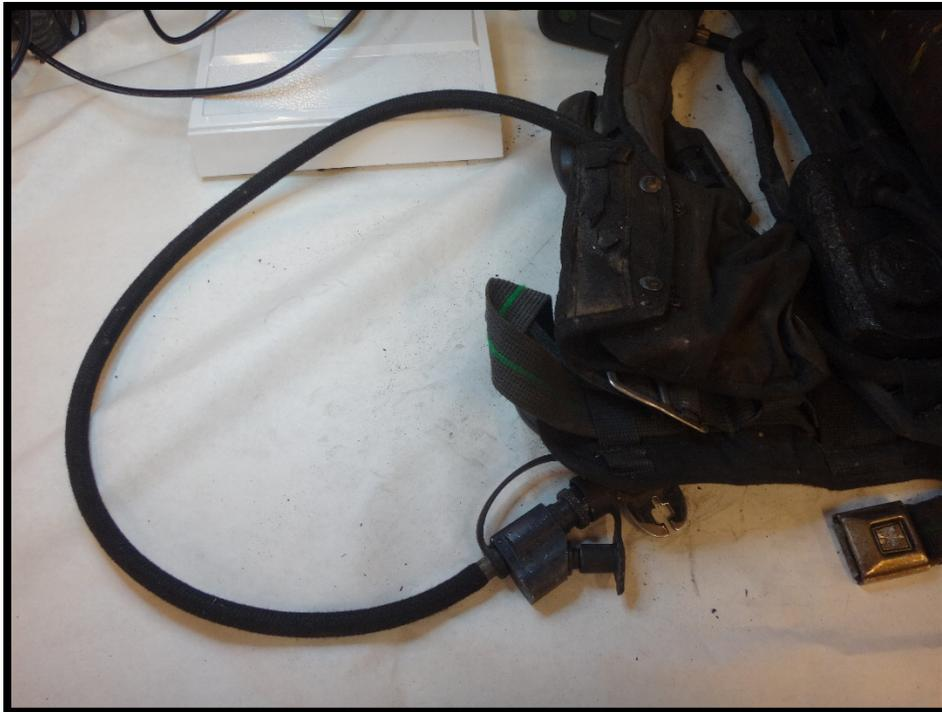
**Figure 19: ExtendAire II EBSS hose with male and female Quick Connect**
