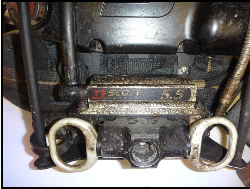
**Figure 9: Pressure reducer.**
