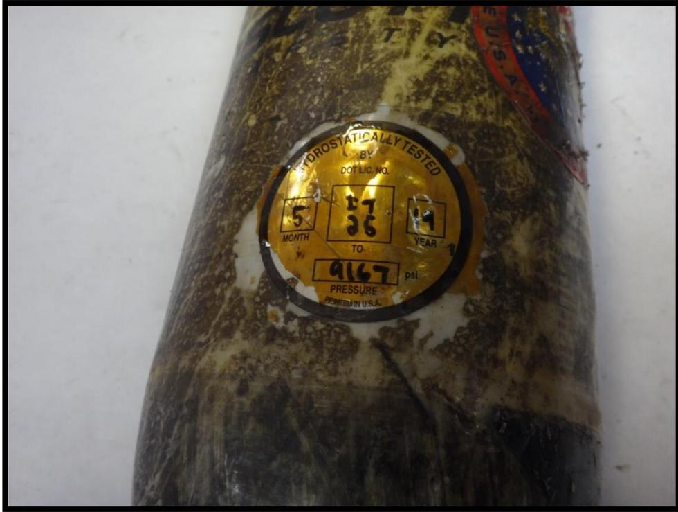
Figure 21: Cylinder hydrostatically tested label.
