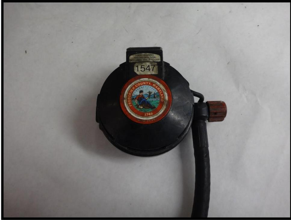
Figure 5: Mask-mounted regulator.
