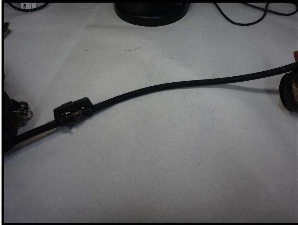
**Figure 7: Low-pressure hose with quick disconnect (connected).**
