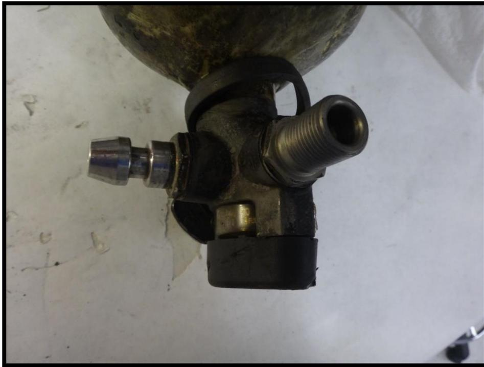
**Figure 20: Cylinder snap-change connector, threaded compress gas association (CGA) (for filling only), and rubber bumper.**
