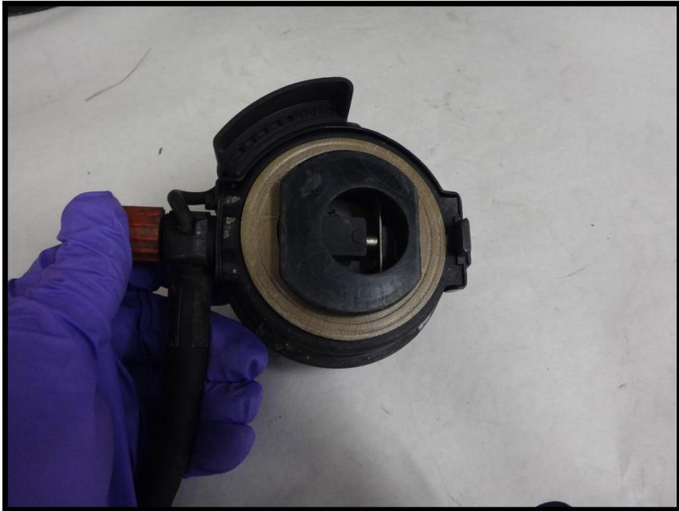
Figure 6: Inside seal of mask-mounted regulator and HUD.
