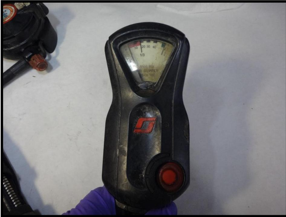
Figure 11: PASS control console.
