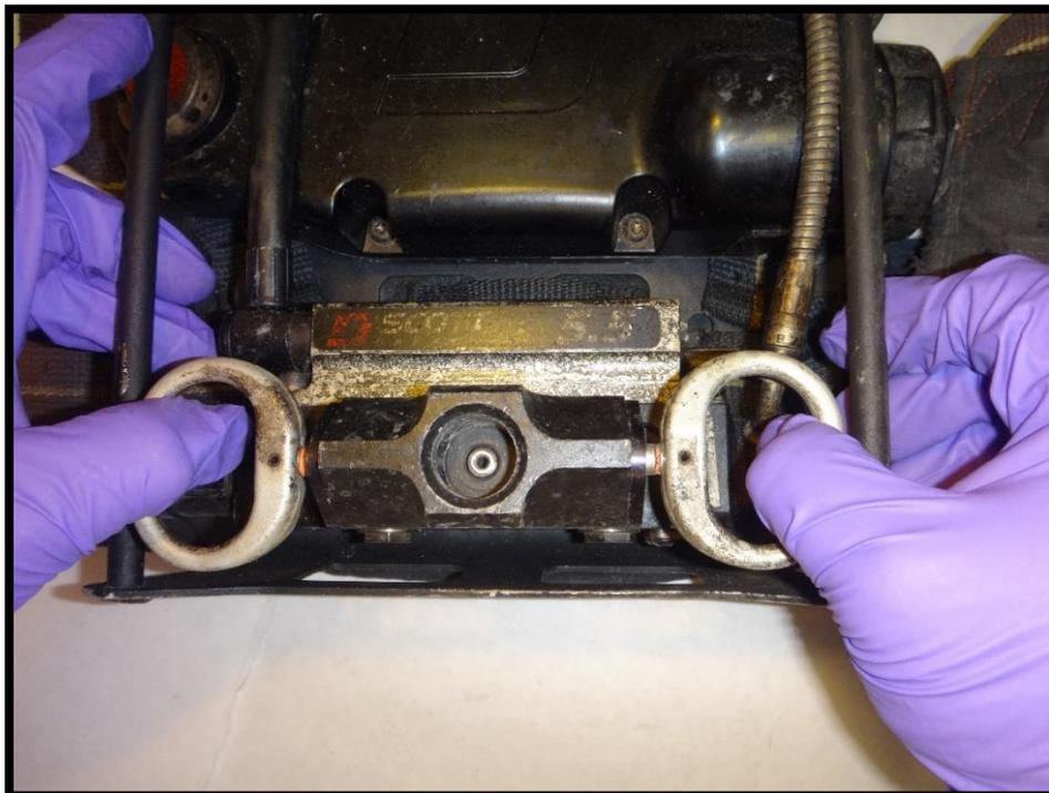
**Figure 18: Cylinder snap-change connector.**
