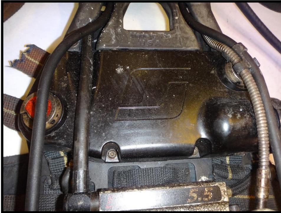
Figure 13: PASS control module.
