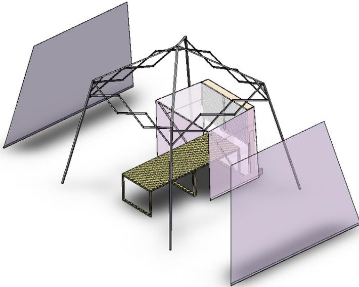
c. For both the left and right side of the enclosure, position and attach one of the plastic sheets to the frame using duct tape. Position the excess length at the bottom for use in making a ballast sleeve. Sloped-wall canopies will have excess plastic width extending beyond the top of the legs, this can be trimmed or wrapped around the corner and attached.
