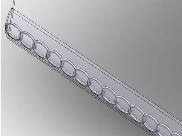
g. Tape the excess plastic at the bottom of the rear and side walls to the floor or fold it over to create a pocket into which ballast (utility chain) can be placed. The pocket is secured using duct tape. Insert utility chain into the pocket to act as a linear ballast along the entire pocket length.
