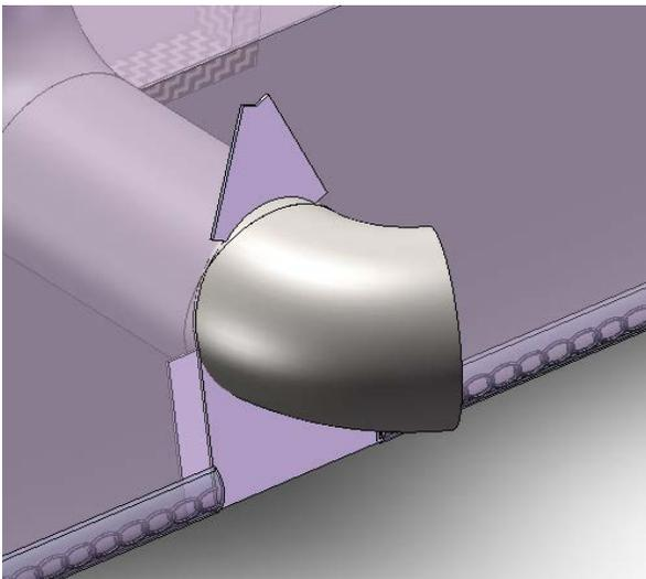
e. Modify the back wall for duct penetration by cutting a slit from the bottom-center of the wall to a height 12-inches above the floor. Insert the duct through the slit and the plastic should fall to the floor on either duct side. Use tape and additional plastic to seal around the duct and prevent excess leakage.
