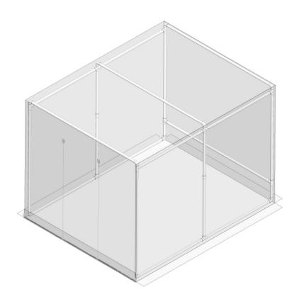
The following materials list and assembly instructions are for a PVC-framed, plastic sheeting-covered tent, intended as an optional 2<sup>nd</sup> level of containment, in conjunction with the expedient airborne isolation *ventilated headboard*. The tent accommodates a single-patient bed (or cot). The design has been optimized to reduce the quantity and cost for construction supplies. All of the construction supplies are items normally found at hardware/building supply stores.
