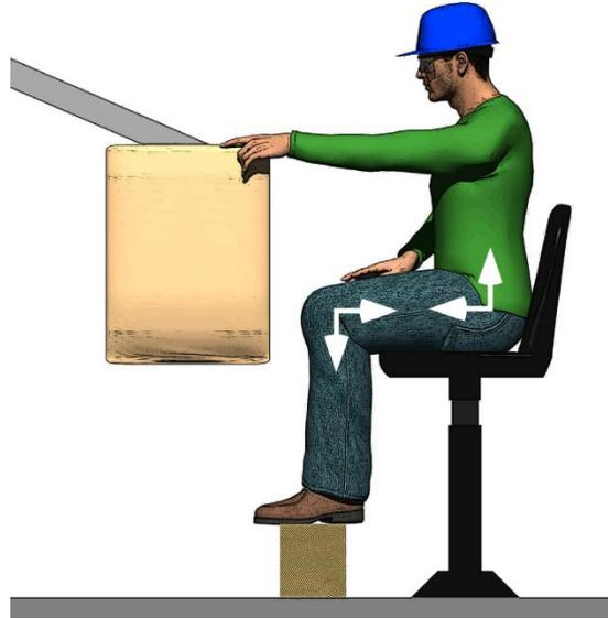
**Figure 19. Worker is sitting with hip and knee at the same level. Both the hips and knees are at approximately 90 degrees angles and the feet are supported.**
