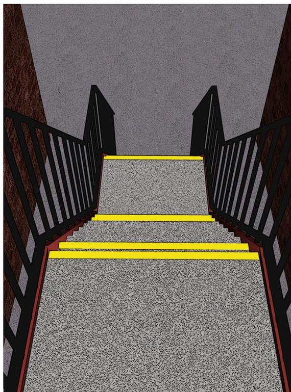
**Figure 13. Painting of stair nosings before and after landings.**
