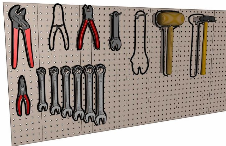
**Figure 11. Tool shadow board.**
