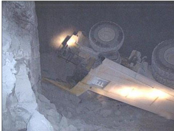
**Figure 19: Overturned haul truck at an underground metal/nonmetal mine where the trainer of a new driver, not wearing a seatbelt, was fatally injured; but the trainee, wearing a seatbelt, survived.**
