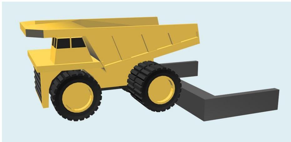
**Figure 11. Bumper block with an exposed barrier and ready for dumping at hopper/crusher.**
