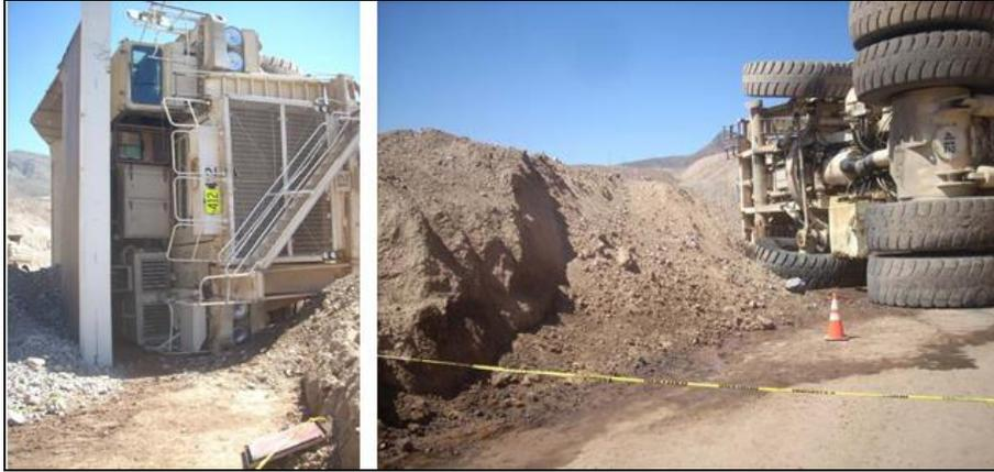
**Figure 22: A 240-ton haul truck climbed the berm and overturned onto the haul road. The driver, who sustained fatal injuries, was not wearing a seatbelt and fell from the cab of the truck.**
