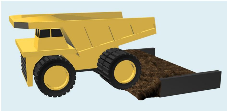
**Figure 10. Excess spillage covering bumper block at the hopper/crusher.**
