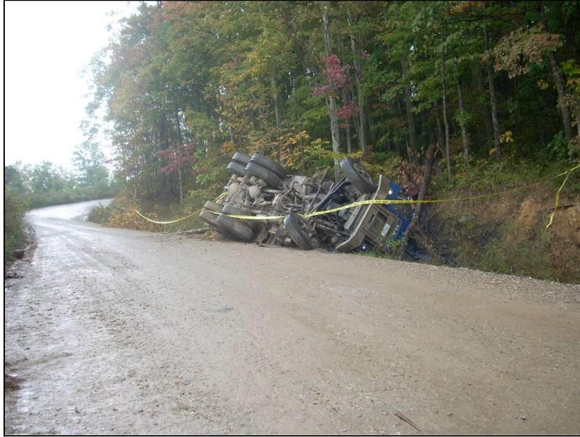
**Figure 20: The driver of an overloaded, tandem-axle haul truck was fatally injured when he may have jumped or was thrown from the cab of the overturned truck.**
