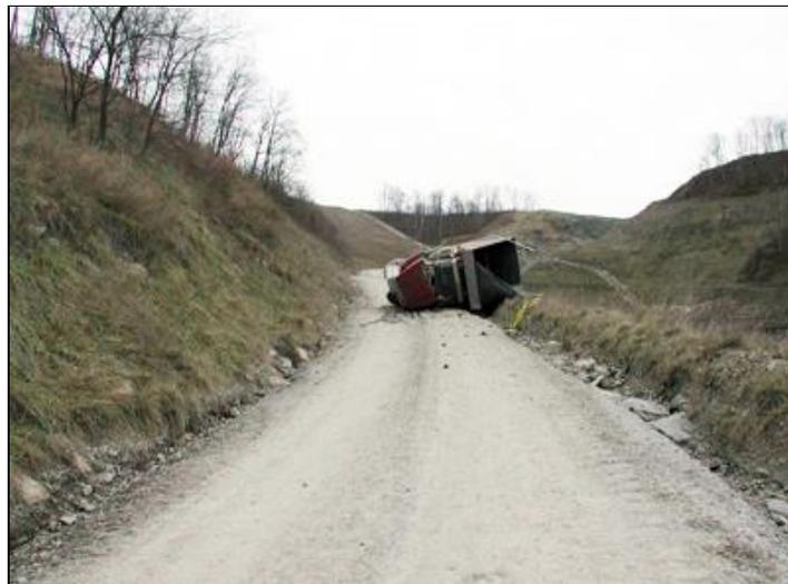
**Figure 21: Loaded haul truck overturned onto the haul road and adjacent drainage ditch. The driver was fatally injured when struck by the left rear tandems of the truck.**
