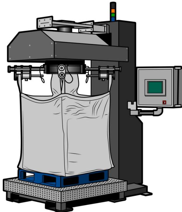
Figure 57. Example of filling station with rotating hooks.
