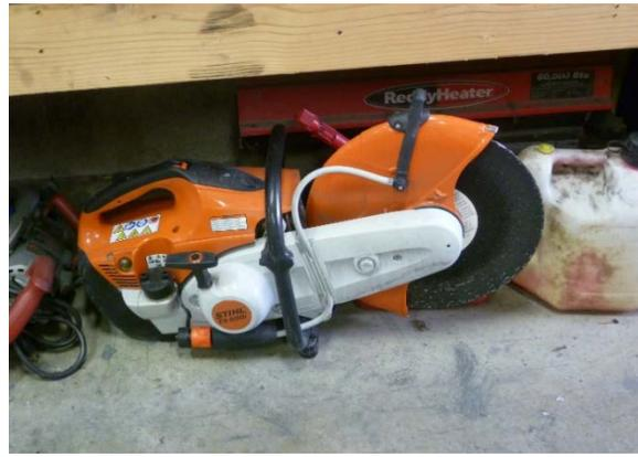
Figure 10. Hand-held, gasoline-powered, water-cooled abrasive cutoff saw. An employee used the saw to cut the 60 pound lead ingots into sizes small enough to fit in the bullet caster melting pot.
