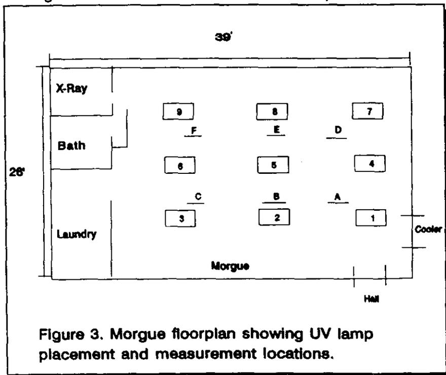
**Figure 3. Morgue floorplan showing UV lamp placement and measurement locations.**
