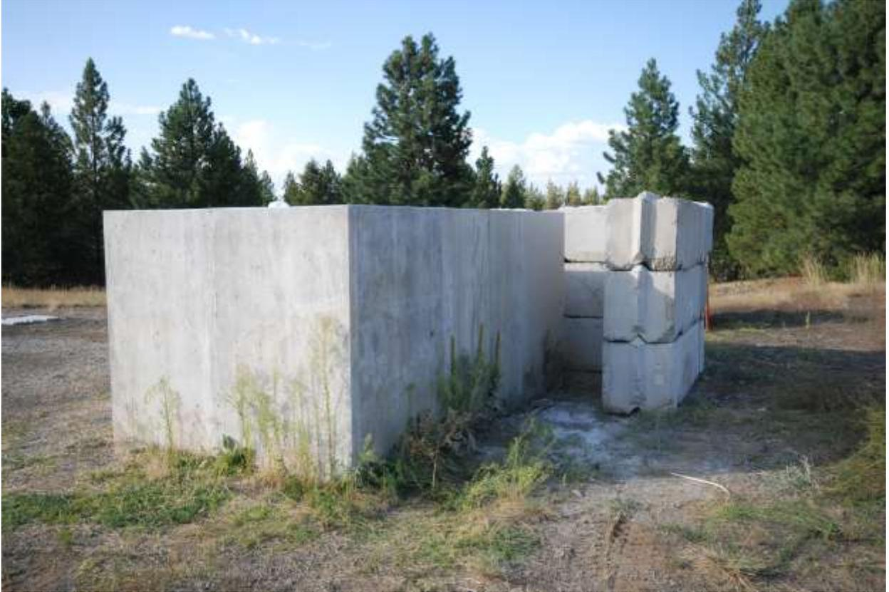
**Figure 12. Block 1 prior to blasting showing flyrock barrier wall installed.**
