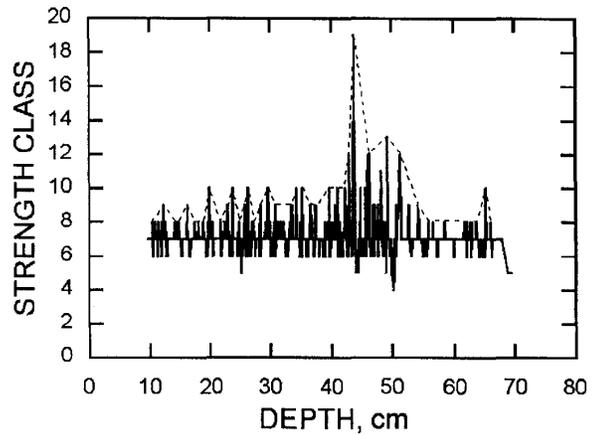
Figure 14.—Detection of inclusion from change in strength.
