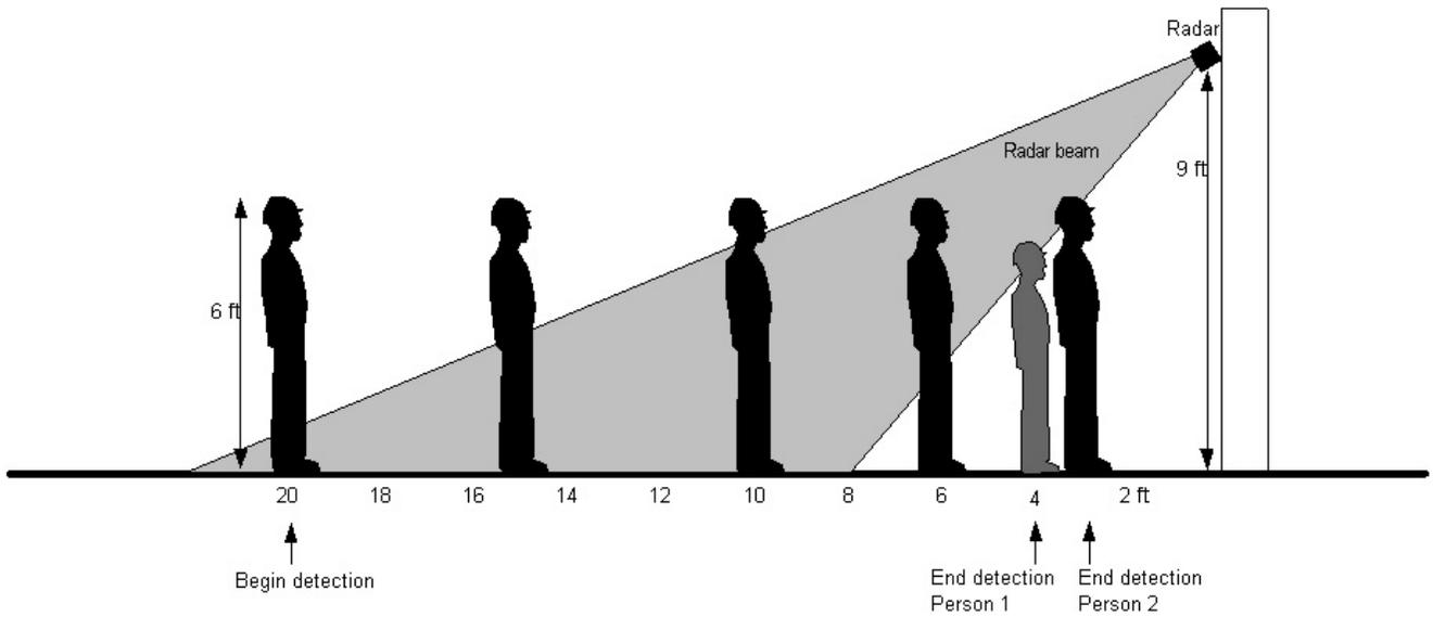
Figure 19.—Example of differences in inner detection ranges.
