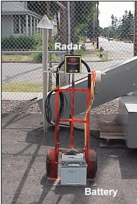
Figure 3.—Radar system mounted on dolly for testing.
