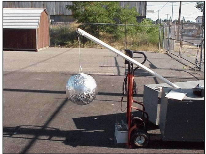
Figure 4.—A test sphere with diameter of 36 cm (14 in).
