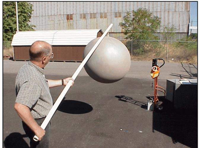
Figure 5.—Ninety-one centimeter (36 in) in diameter weather balloon coated with conductive paint.
