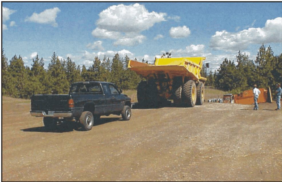
Figure 6.—Test configuration using pickup as obstacle.
