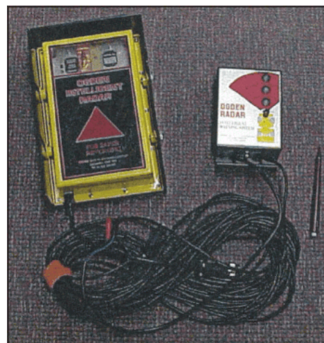
Figure 2.—FMCW radar-based collision warning system manufactured by Ogden Safety Systems showing antenna and electronic enclosure (left) and alarm display (right).
