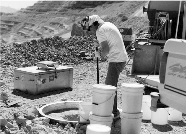
Figure 4.—Frame for in situ density tests.
