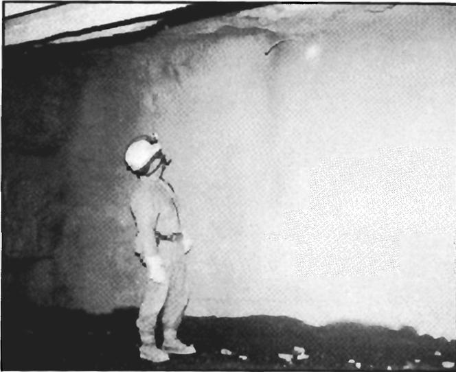
Figure 27.—Front (C-drift) side of seal 3 after LLEM test 348.
