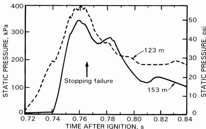
Figure 21.—Pressure data for stopping 5, showing time of stopping failure for LLEM test 348.
