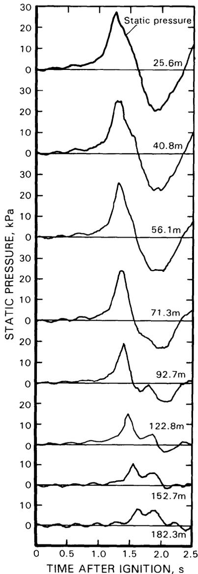
**Figure 35.—Pressure traces as a function of distance in C-drift for LLEM test 350.**
