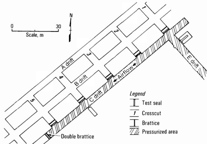
Figure 5.—Pressurized entry for leakage determination rates across the seals.
