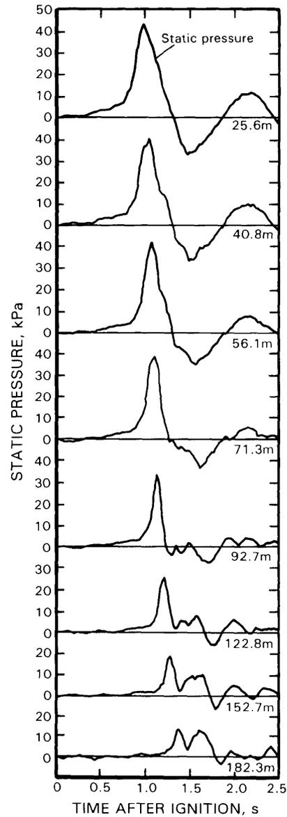
**Figure 36.—Pressure traces as a function of distance in C-drift for LLEM test 351.**
