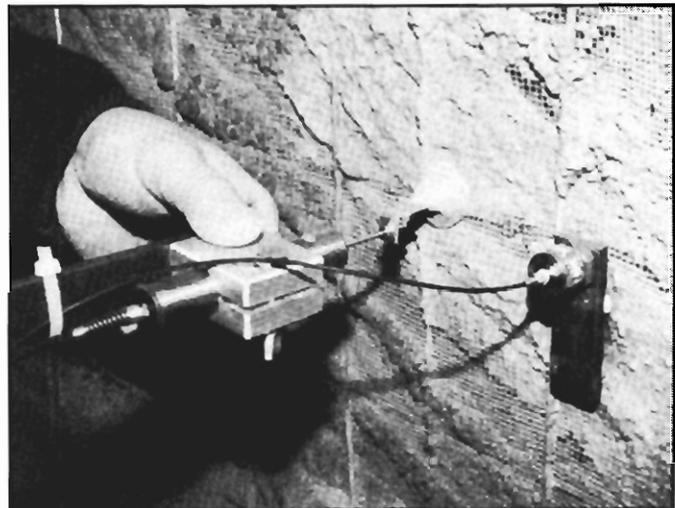
**Figure 3.—Linear variable displacement transducer (LVDT) and accelerometer attached to a seal.**
