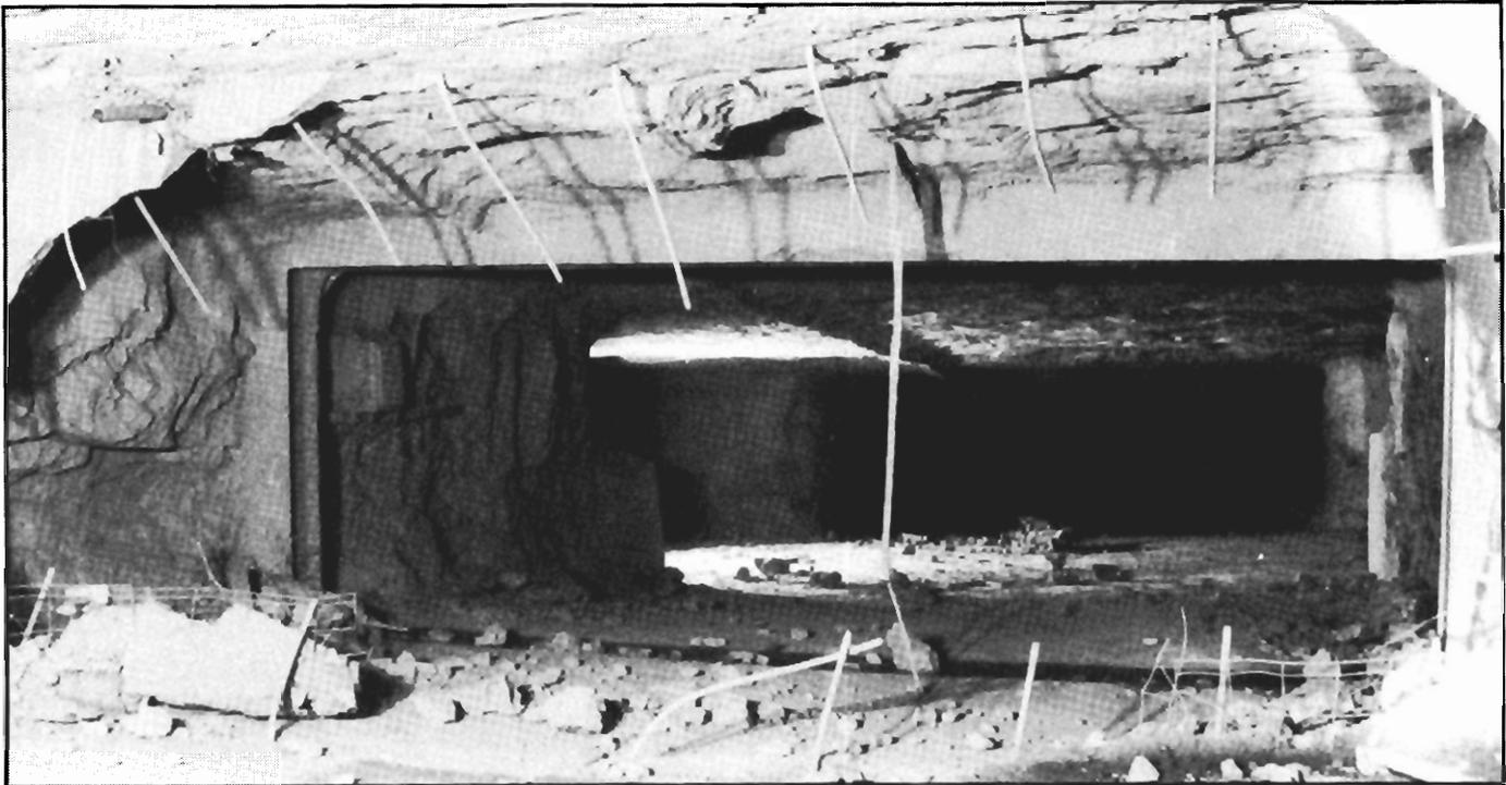
Figure 24.—Remains of seal 4 after LLEM test 348.
