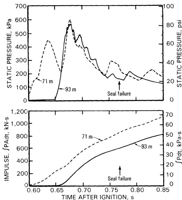
Figure 31.—Pressure and impulse data for seal 3, showing time of seal failure for LLEM test 349.
