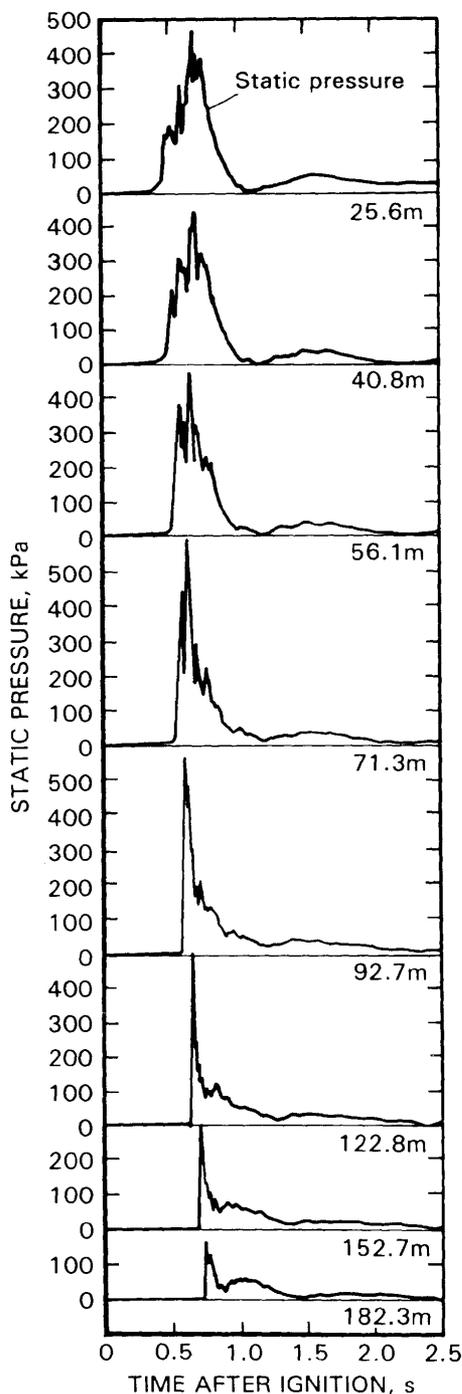
Figure 30.—Pressure traces as a function of distance in C-drift for LLEM test 349.
