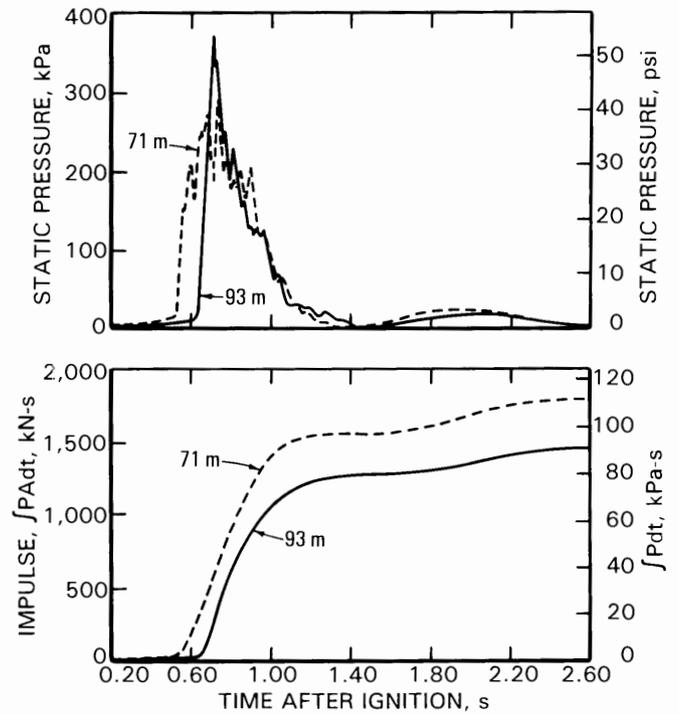
Figure 26.—Pressure and impulse data for seal 3 for LLEM test 348.
