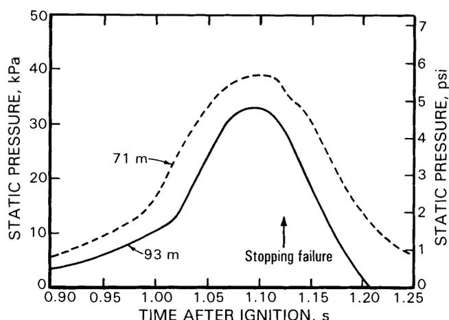
Figure 37.—Pressure data for stopping 3, showing time of stopping failure for LLEM test 351.
