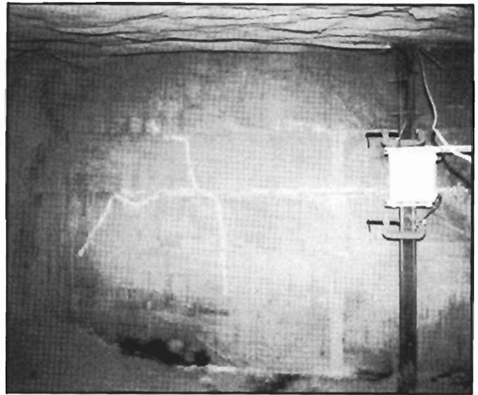
Figure 29.—Back (B-drift) side of seal 2 after LLEM test 348, showing crack pattern marked with white chalk.
