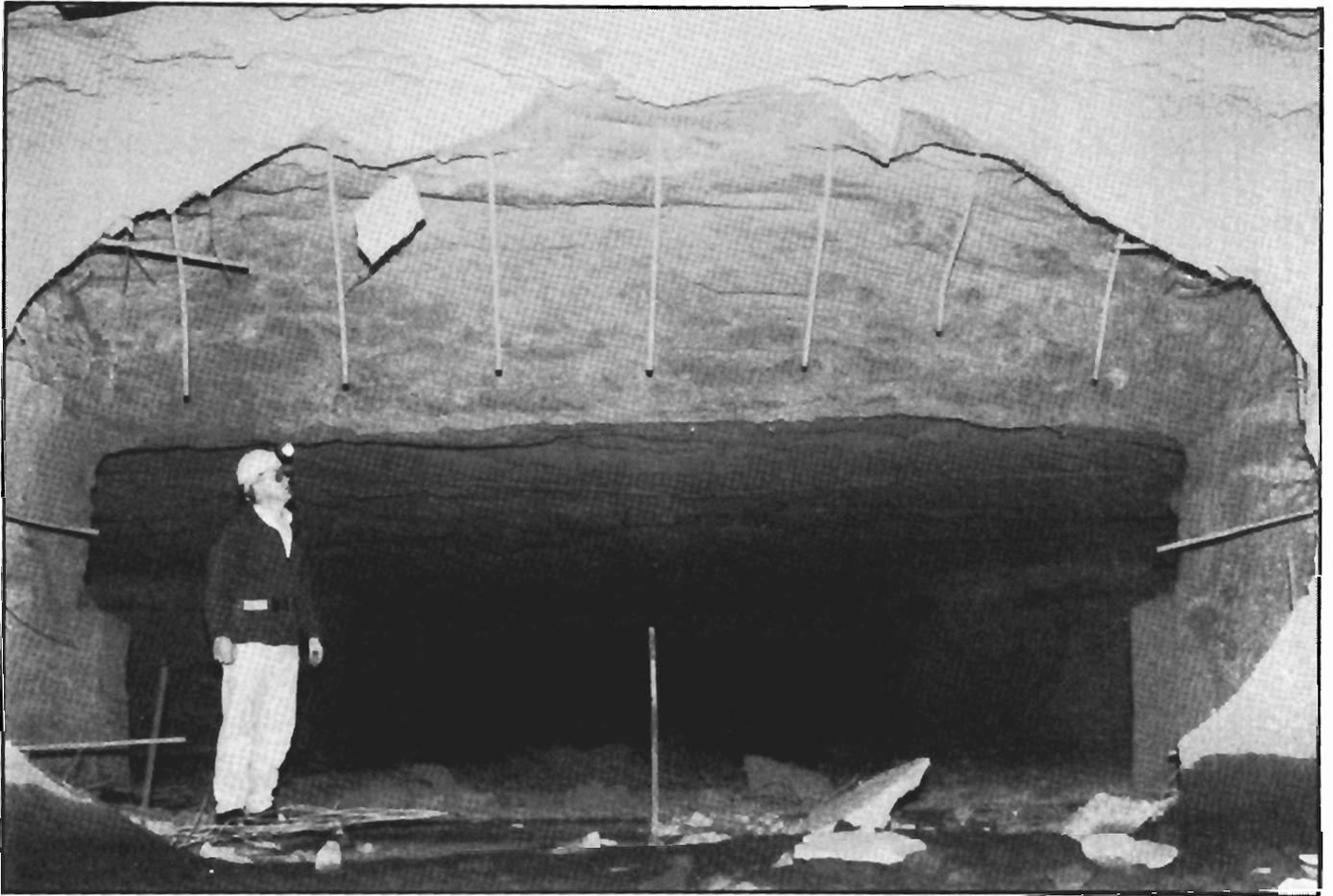
Figure 32.—Remains of seal 3 after LLEM test 349.
