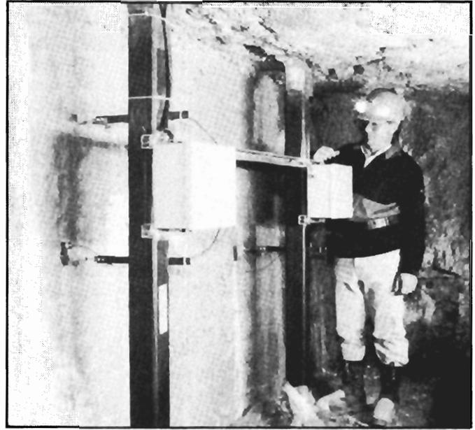
**Figure 4.—Support posts and instrumentation on the back side of a seal.**
