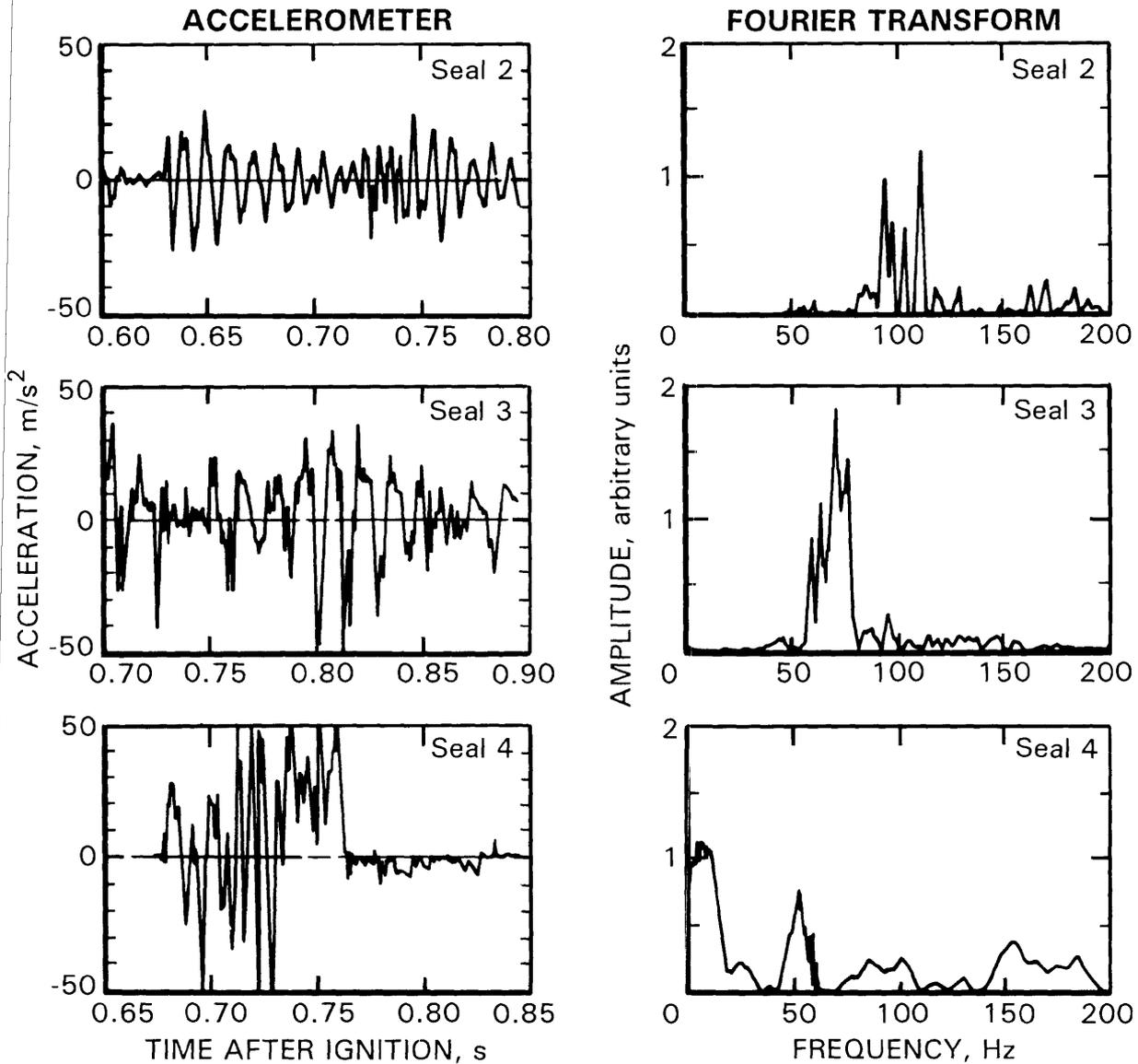
Figure D-1.—Data from middle accelerometers on seals 2, 3, and 4 for LLEM test 348, along with their Fourier transforms.
