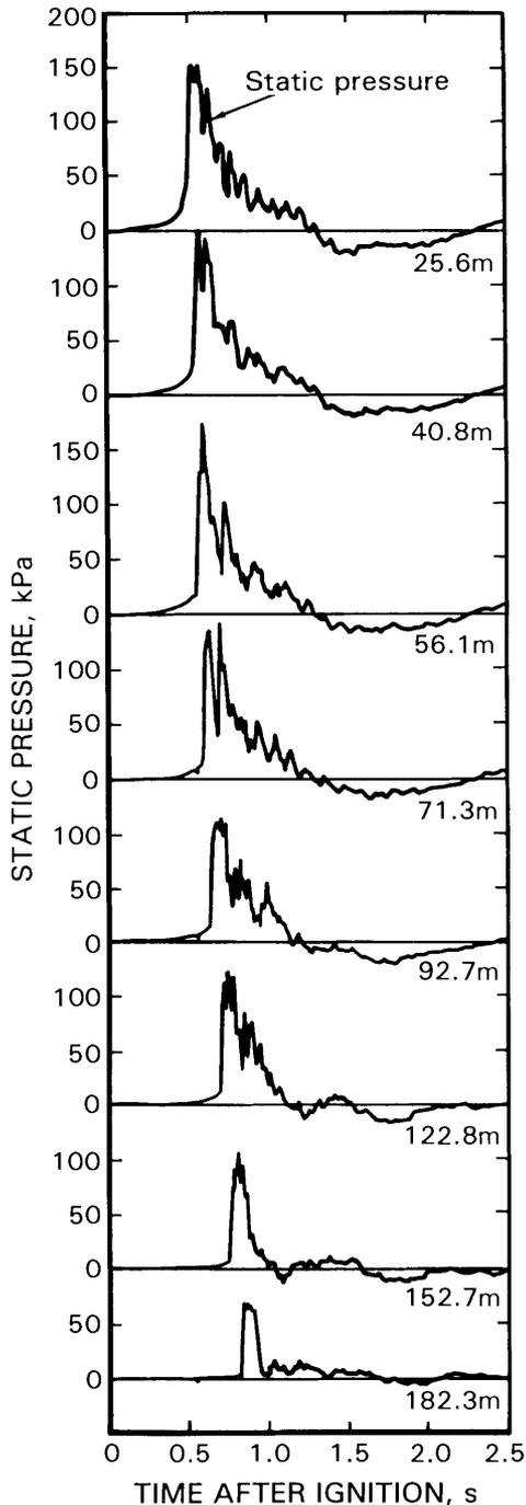
Figure 19.—Pressure traces as a function of distance in C-drift for LLEM test 347.
