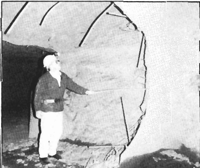
Figure 33.—Remains of seal 3 after LLEM test 349 (closeup view near wall).
