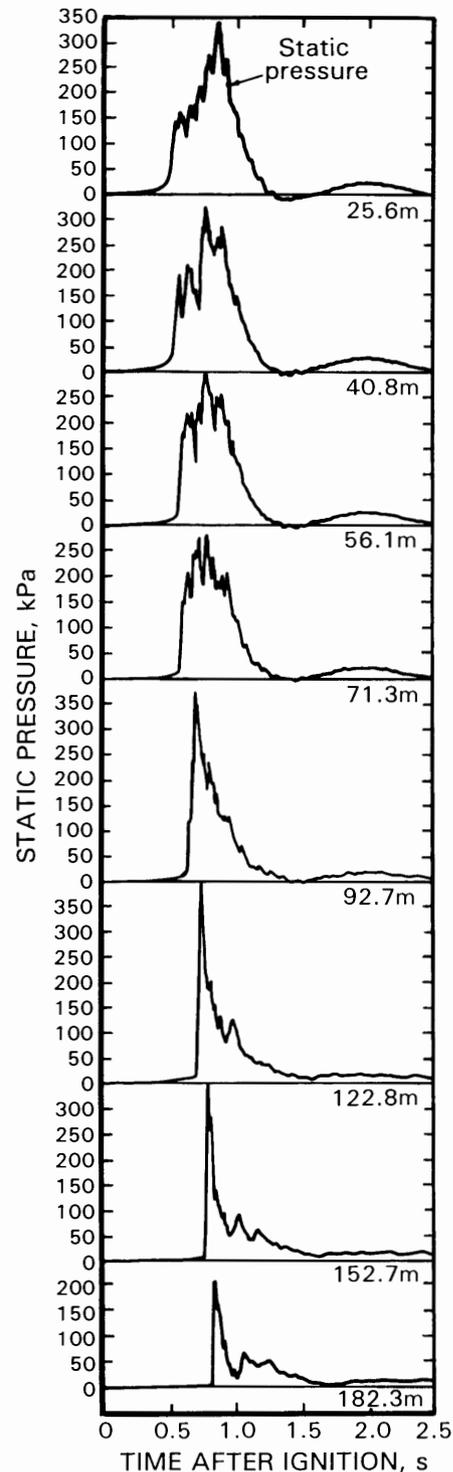
**Figure 20.—Pressure traces as a function of distance in C-drift for LLEM test 348.**
