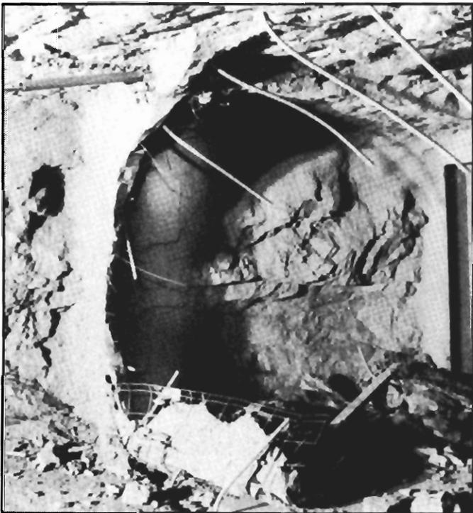
Figure 25.—Remains of seal 4 after LLEM test 348 (closeup view near wall).
