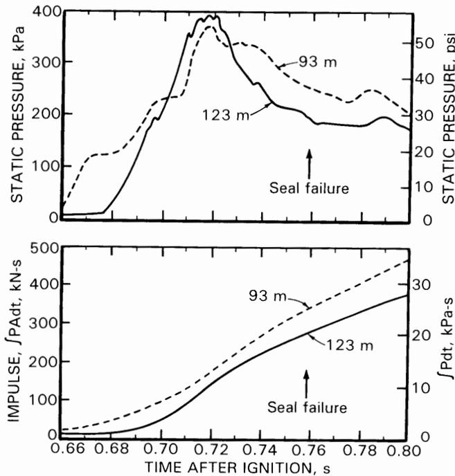
Figure 23.—Pressure and impulse data for seal 4, showing time of seal failure for LLEM test 348.
