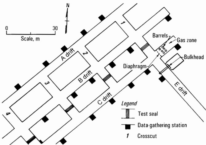
Figure 2.—Seal test area in the LLEM.
