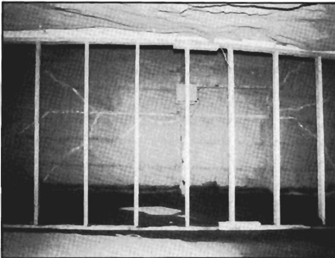
Figure 28.—Back (B-drift) side of seal 3 after LLEM test 348, showing crack pattern marked with white chalk.
