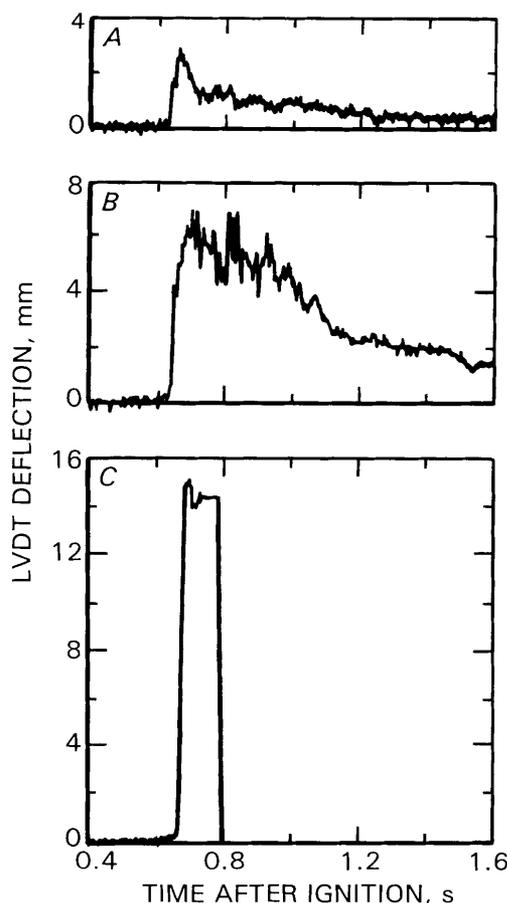
Figure 38.—Data for the middle LVDT on seal 3 for (A) LLEM test 347, (B) LLEM test 348, and (C) LLEM test 349.
