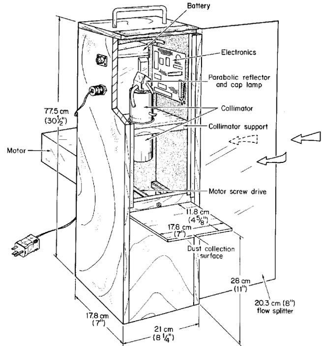
Figure 4.—Float dust deposition meter used during full-scale studies at the Lake Lynn Experimental Mine.
