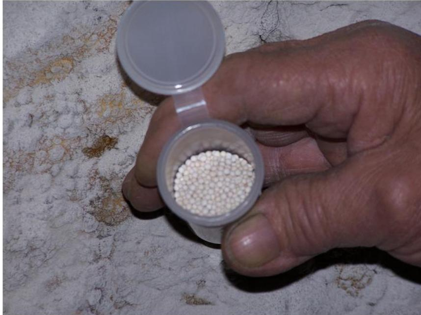
**Figure C1. Sample tube containing molecular sieves.**
