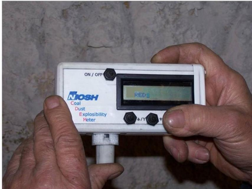
**Figure C6. Testing a dust sample with the CDEM.**
