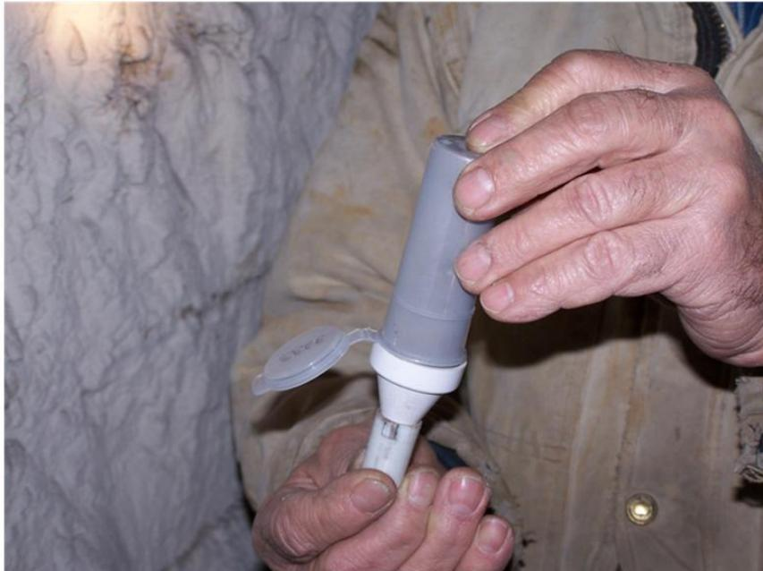
**Figure C5. Transferring dust to a sample cup.**
