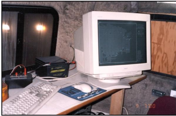
Microseismic system at mine site trailer.
