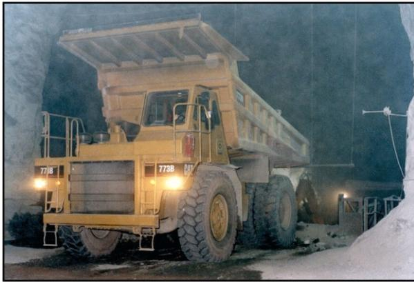
Haul truck dumping at a crusher in an underground limestone mine.
