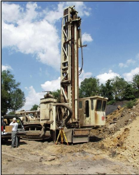
Preparing to sample dust generated by a surface drill.
