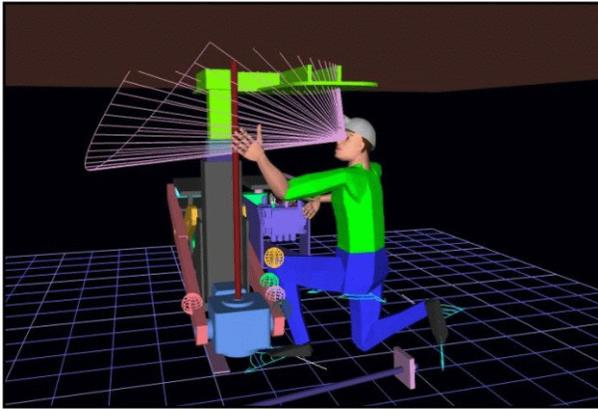
Computer simulation is being used in research to determine safe boom speeds for roof bolters.
