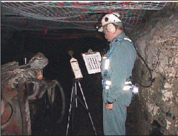
Noise profiling of underground mining equipment.
