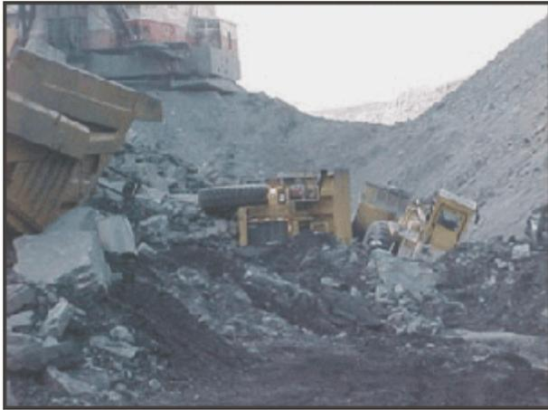
Catastrophic slope failure in a surface mine.
