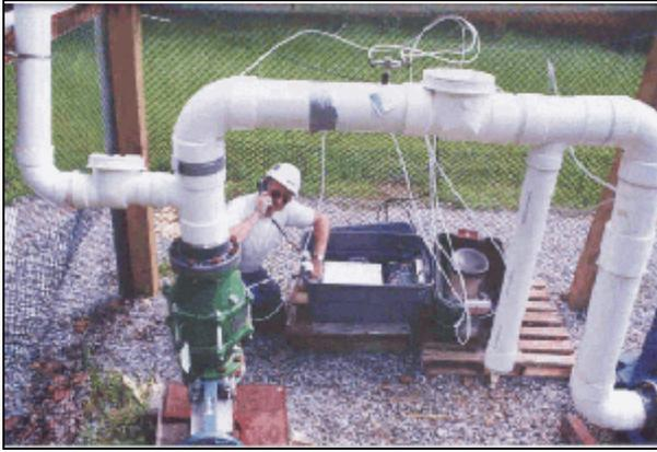
A researcher checks the cellular telephone data transmission components of the Remote Gob Gas Venthole Data Acquisition and Transmission System.
