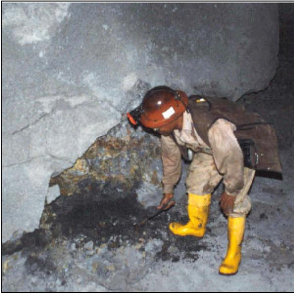
Rib failure at an underground gold mine in Nevada.
