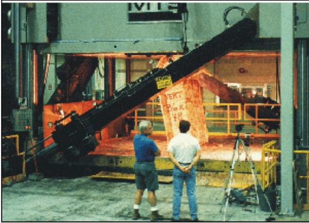
Safety performance testing of an innovative timber support in the Mine Roof Simulator.
