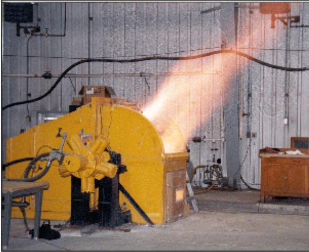
Frictional test apparatus showing ignition of methane-air.
