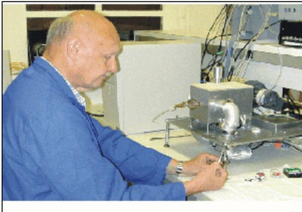
Research scientists, using the thermo-optical method (NIOSH method 5040 for carbon) to determine the amount of DPM on filter samples collected in the workplace, are able to assess worker exposure and effectiveness of emission control systems.
