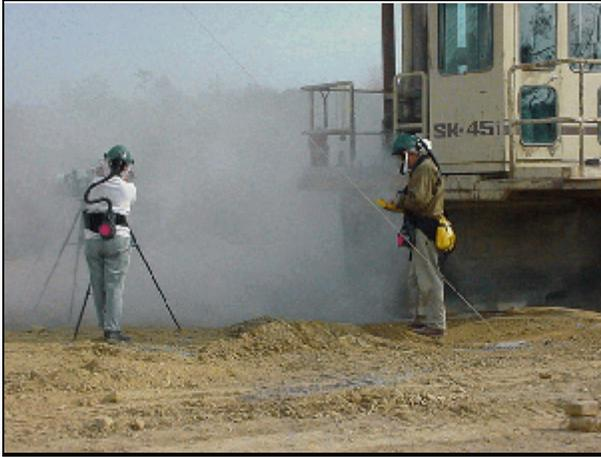
Integration of GPS and GIS to map the distribution of air-borne and ground dust and particulate matter.
