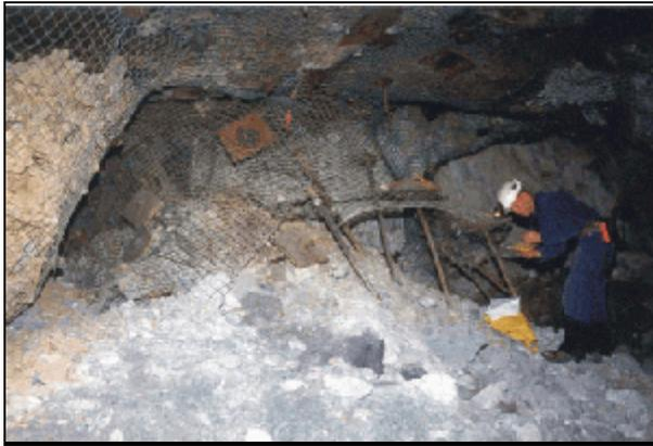
Rock burst damage in a hard-rock mine.
