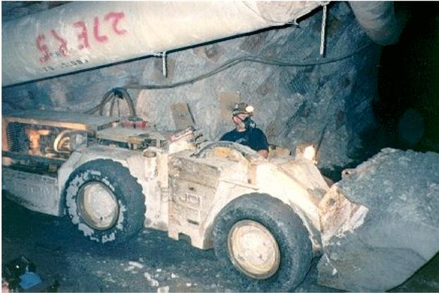
**Diesel exhaust filtration on mining equipment offers substantial reductions in workplace concentrations of diesel particulate matter.**
