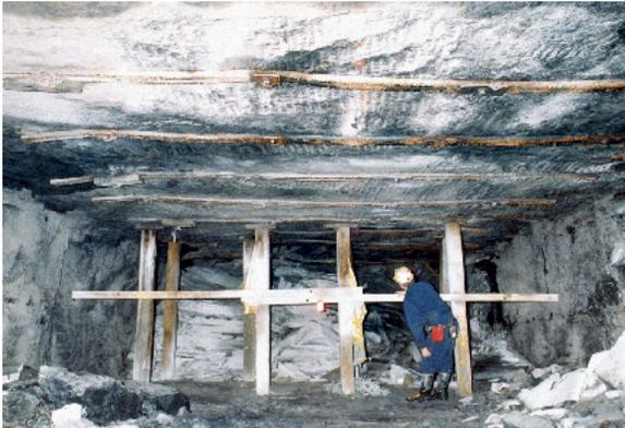
Site of fatality caused by massive sandstone roof failure in a mine in Mingo County, WV.
