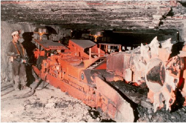
Miner operating a continuous mining machine using a remote control.
