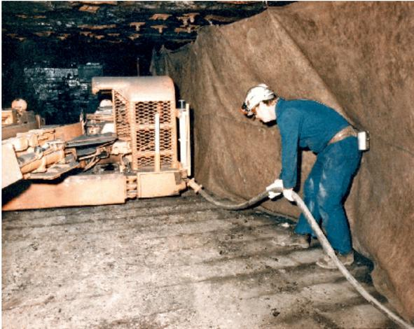
Underground coal mine workers may be electrically shocked when handling portable power cables with defective insulation.
