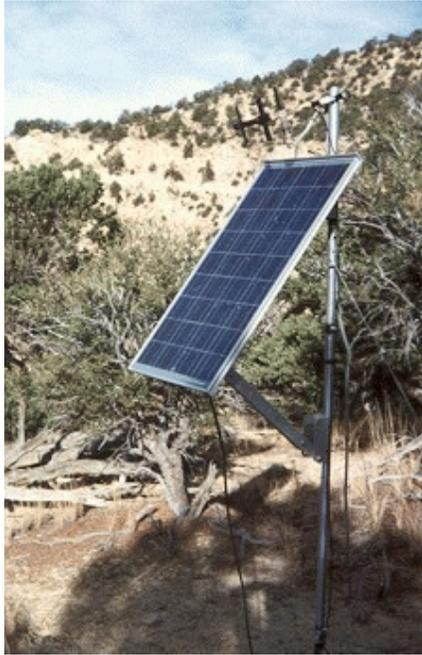
Solar panel generates energy for monitoring seismic activity in the mountains.
