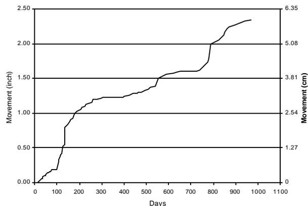
Figure 21. Roof movement at RMSS #27.
