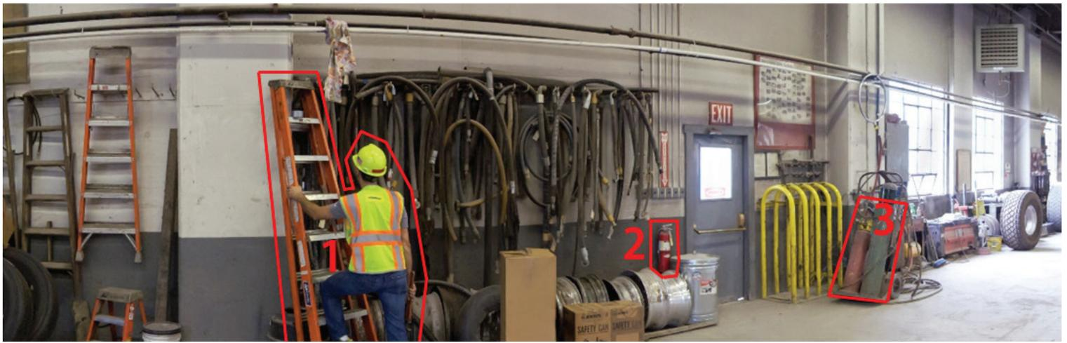
Figure 2: Example of three hazards outlined in red from EXAMiner, taken from the left side of the panoramic image of the shop shown in Figure 1.
